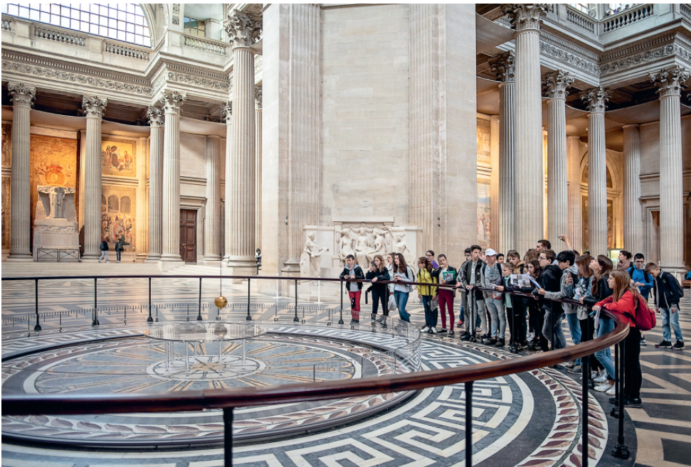
Figure 1. A Foucault pendulum placed in the hall of the Pantheon in Paris, where the experiment designed by Foucault was carried out in 1851. The pendulum, once shifted from its equilibrium position, swings in a plane that is progressively rotating.
