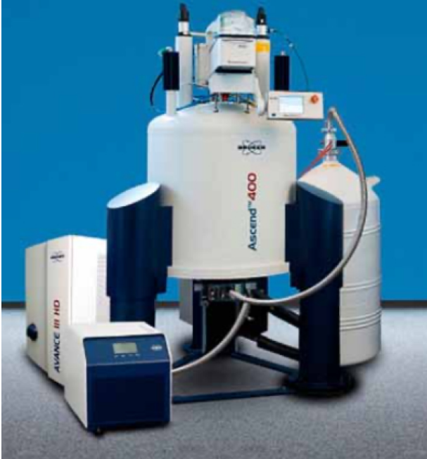
Figure 4. Medium-size NMR spectrometer for laboratory measurements. The sample is placed in a tube that is often settled from the top of the device. The liquid nitrogen reservoir on the right cools the superconducting magnet.
