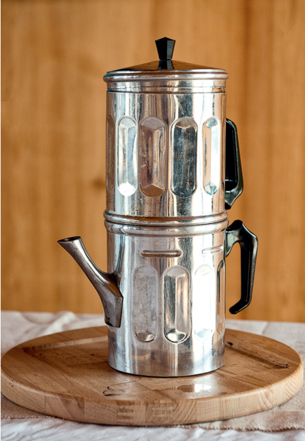
Figure 5. Neapolitan coffee maker. When the water in the bottom boils, the coffee maker is turned over, and the coffee passes through the filter by gravity.
