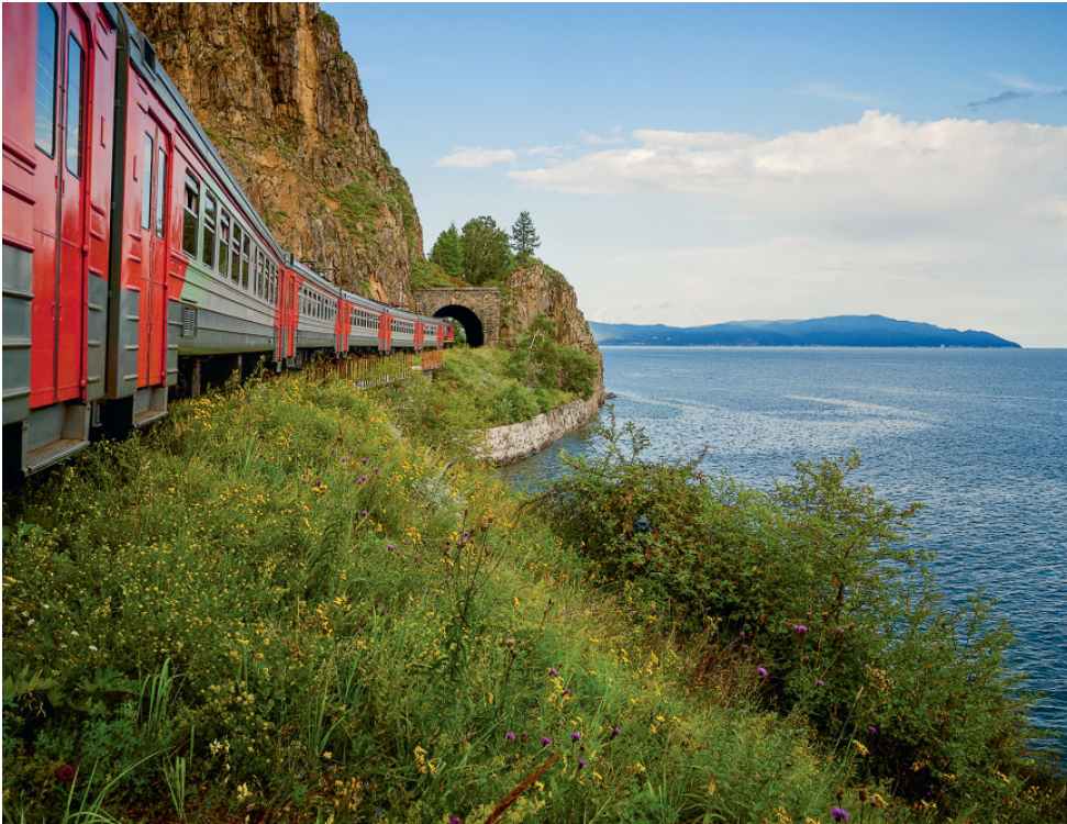
Figure 1. When the train enters a tunnel at high speed, an unpleasant sensation occurs in the passenger's ears due to a variation of the pressure.
