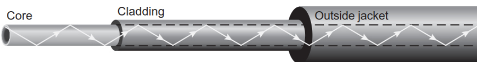
Figure 2. Trajectory of a light ray inside an optical fibre. The propagating ray is totally reflected at the interface between the heart and the sheath, thus being driven along the fibre. The data are codified by means of variation in the intensity of the light.
