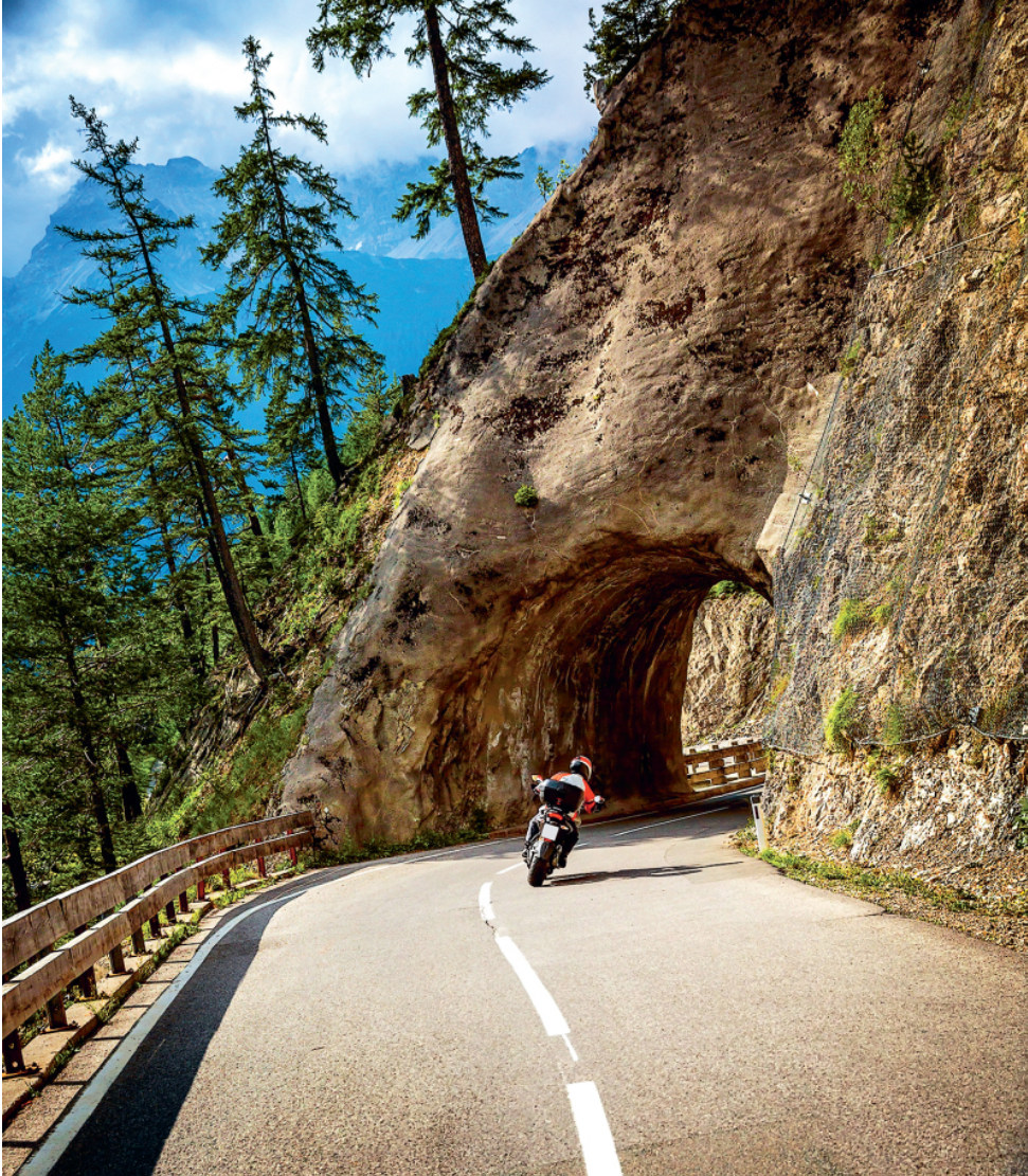
Figure 5. The motorcyclist is leaning towards the interior of the curve in order to cancel the effect of centrifugal force. In a narrow curve, the speed of rotation is increased, and therefore the centrifugal force also increases and becomes relevant.
