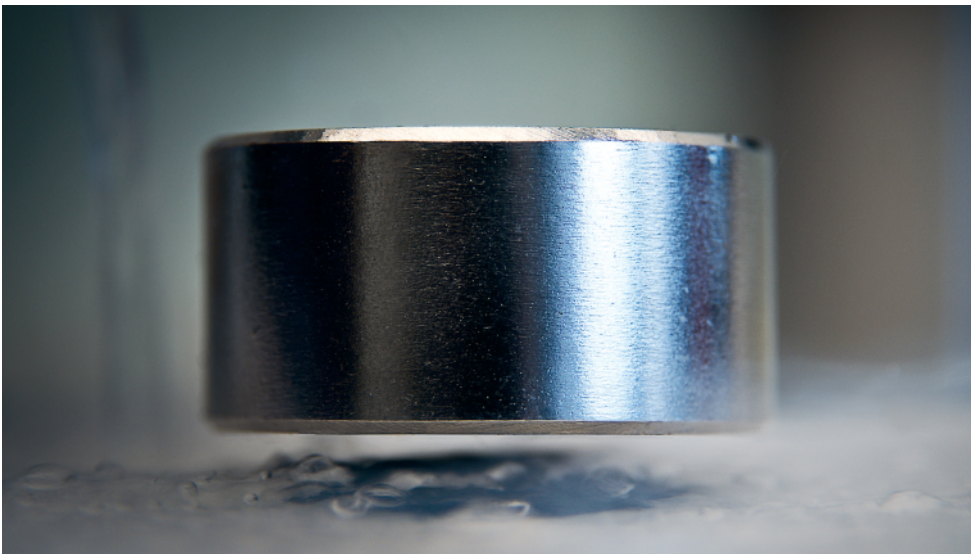
Figure 4. Permanent magnet levitates over a superconductor.
