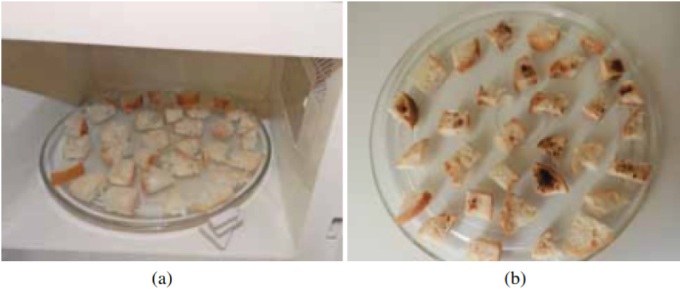
Figure 6. The experiment shows the marked heterogeneity in a microwave oven during the heating. (a) A plate with bread chips is put on the oven plate which is prevented from rotating. (b) After turning on the radiation (for about a minute, at average power), some bread chips are carbonised, while others continue to be white, and others only slightly burned.
