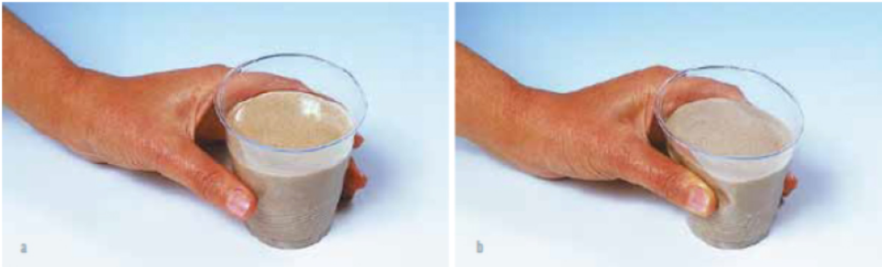
Figure 8. Evidence of the effect related to spreading out of the sand under pressure. (a) The plastic jar containing sand filled with water up to the level of the sand; (b) when the plastic jar is pressed in the middle, the water disappears from the surface of the sand.
