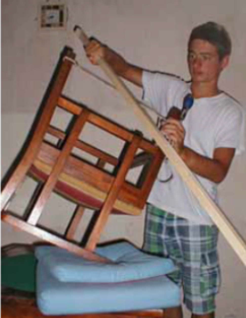
Figure 4. Experiment of rubbing a ruler on taut cord. The cord is shifted from its equilibrium position but does not vibrate unless one keeps the contact with the rule. On the other hand, one can get a sound “pizzicato” by briefly plucking the cord.
