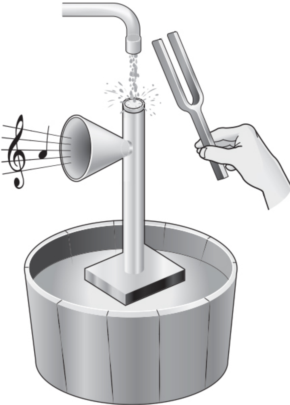
Figure 13. The water microphone of Alexander Bell.
