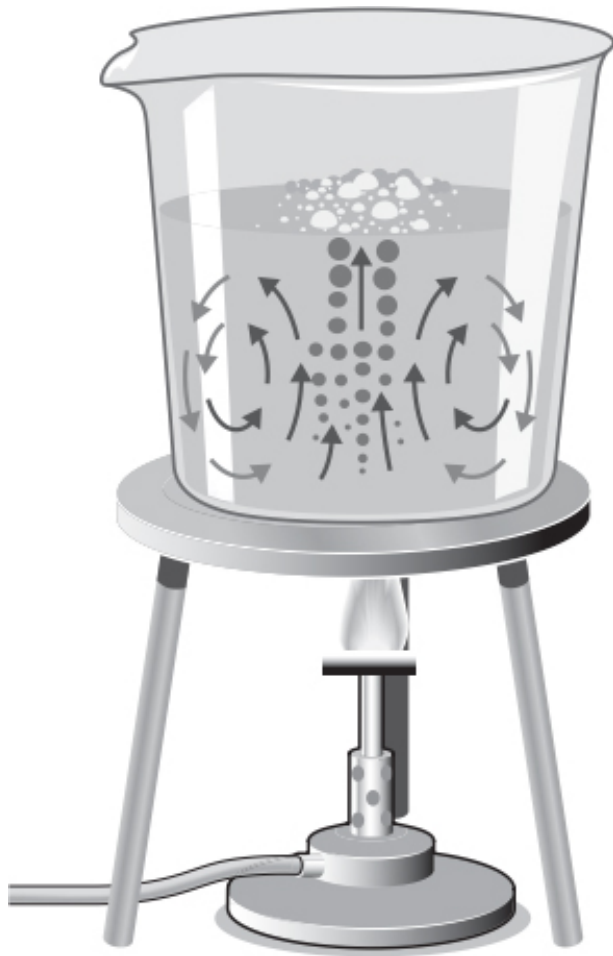
Figure 8. Evidence of convection currents by heating a glass of water. The liquid in contact with the bottom is getting warm and goes up, inducing a circulation in the vessel.
