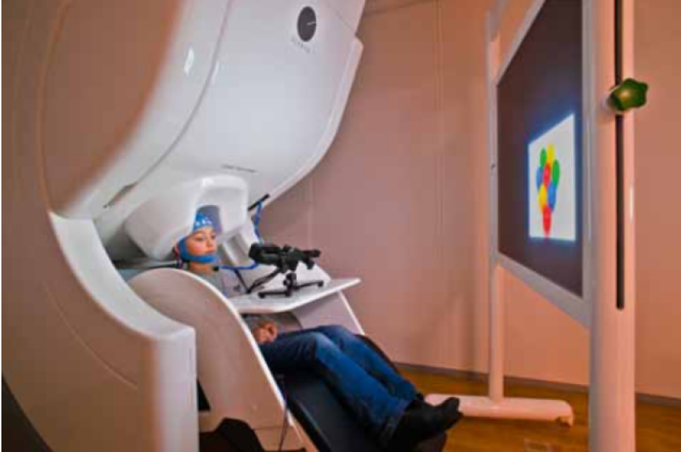
Figure 5. Magnetoencephalographic scanner, consisting of 306 SQUIDs that register even extremely weak magnetic fields generated by neural activity. The top of the scanner contains the liquid helium needed to cool the device. The child's neural activity is detected through visual and auditory stimulation (a black oculometer complements the apparatus).
