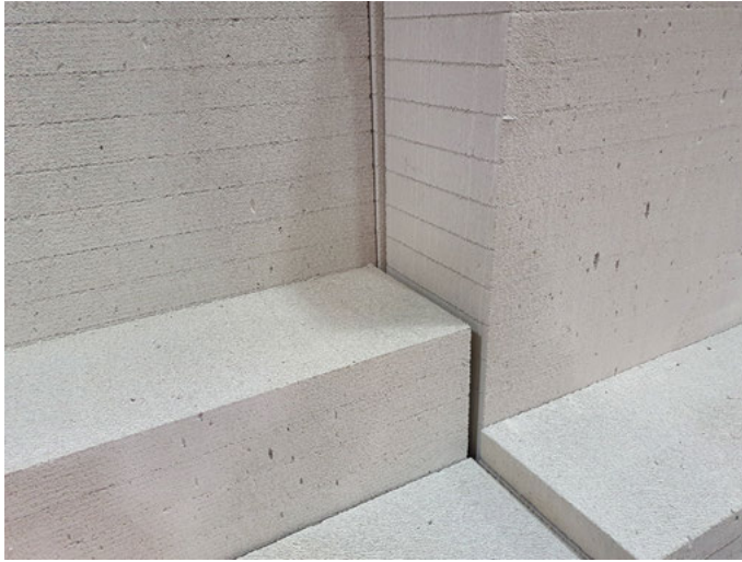
Figure 16.3: Panels consisting of pure uncolored concrete.
