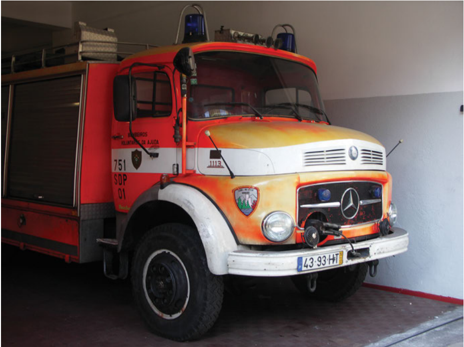
Figure 22.71: Organic fluorescent pigments require special application techniques and care because they are not light stable.
