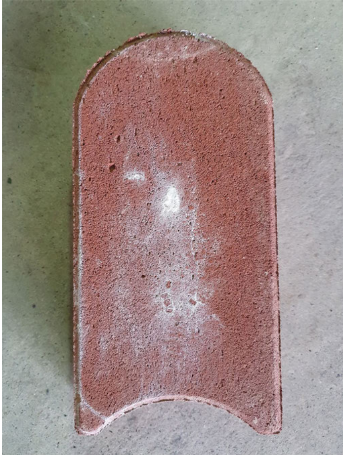
Figure 16.4: Paving slab showing the effect of efflorescence.
