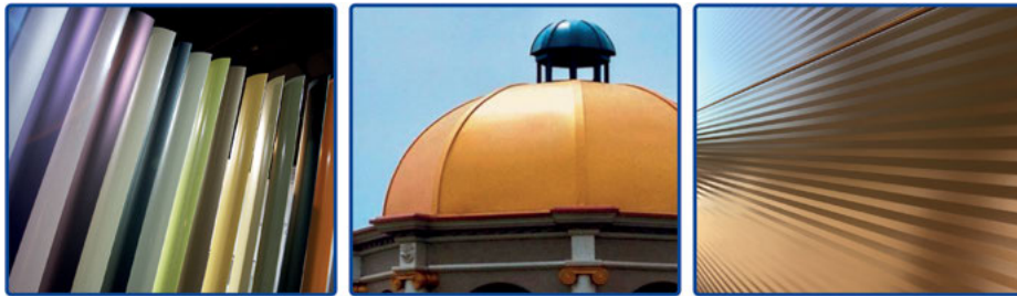
Figure 17.18: Effect pigments used in coatings, shown here in architectural applicants (left to right): powder coating, dispersion and coil coating application [160].
