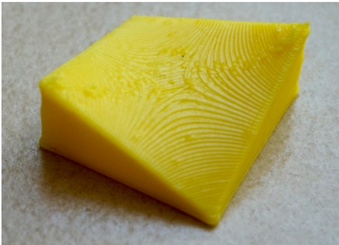
Figure 1-1. Saddle function with a flat bottom. Printed at quarter scale, so each side is about 25 mm, or just under an inch long. Layer height was 0.2 mm
