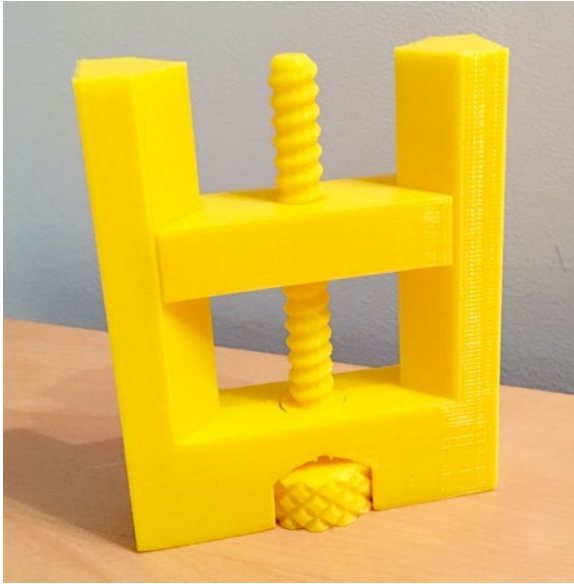
Figure 5-7. Vise (screw) model
