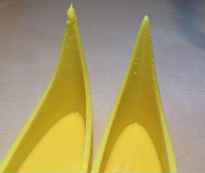
Figure 3-9. The Halley's Comet orbit model peak printed without a cooling tower (L) and with one (R)
