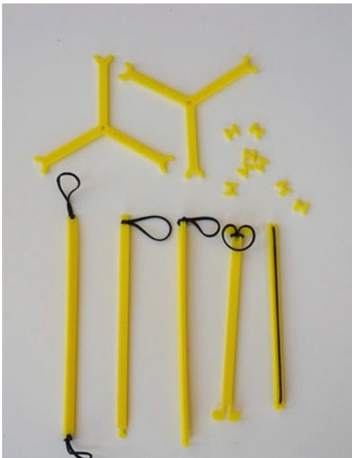
Figure 8-18. The tensegrity elements and assembly aids that did not work (with the one that did on the bottom right)
