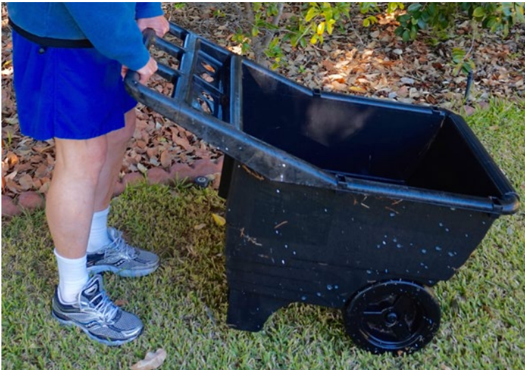
Figure 5-8. Wheel and axle, combined with a lever, in a modern wheelbarrow
