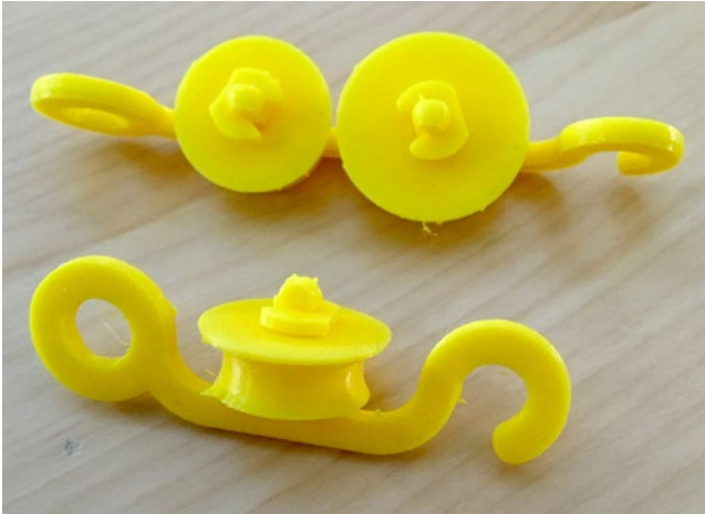
Figure 5-13. The pulleys printed in Figure 5-11, assembled
