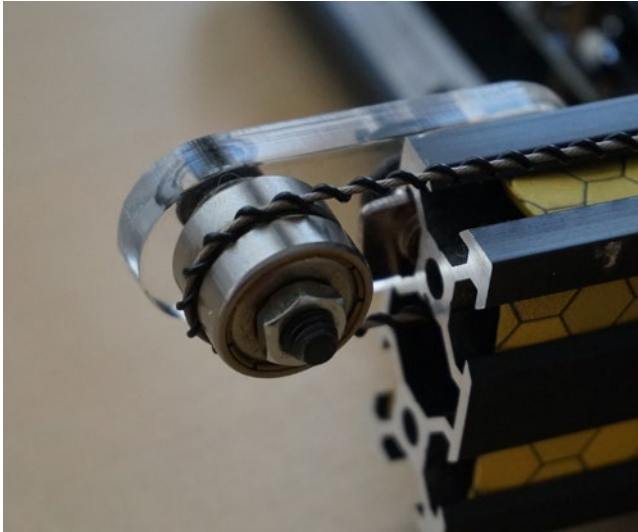
Figure 5-9. Idler pulley on a consumer 3D printer
