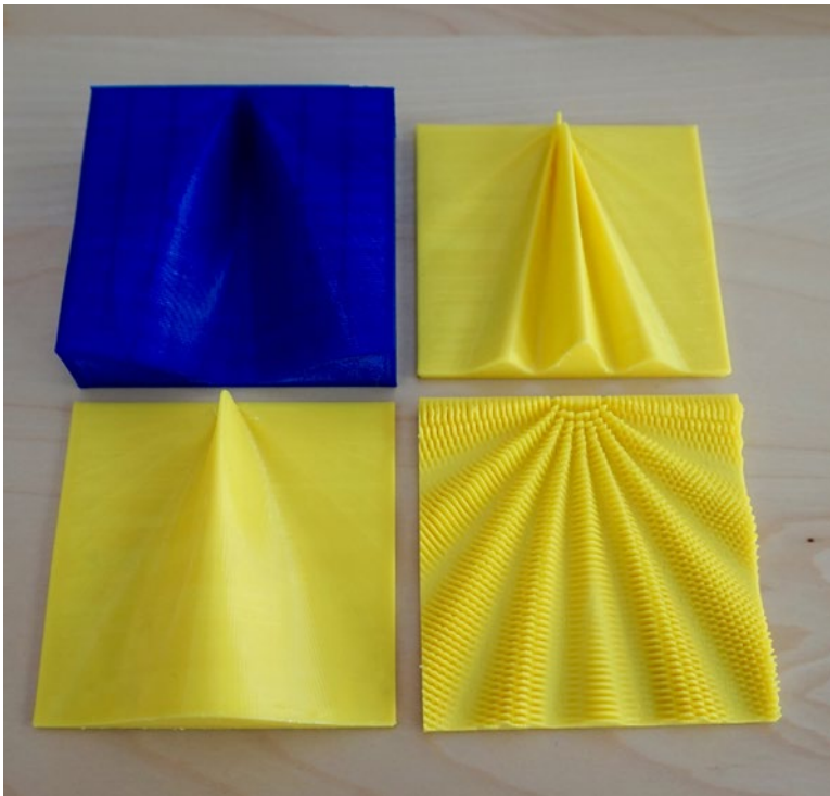
Figure 2-9. Inverted one slit (top L), two slits (top R), one slit (bottom L), and two point sources spaced the same as the slits and using the same wavelength (bottom R)
