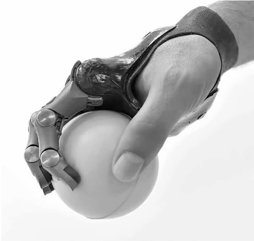
Figure 5.3 Automatically designed 3D printed partial hand prosthetic component.
