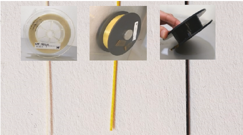
FIGURE 2.4 Photograph of glass, Kevlar, and carbon fiber filaments.
