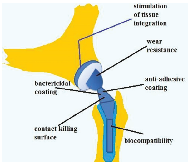
FIGURE 24.1 Schematic of artificial bone prostheses showing antibacterial properties. Adapted with permission [5]. Copyright: The Authors, some rights reserved; exclusive licensee [IOP Publishing]. Distributed under a Creative Commons Attribution License 3.0 (CC BY).
