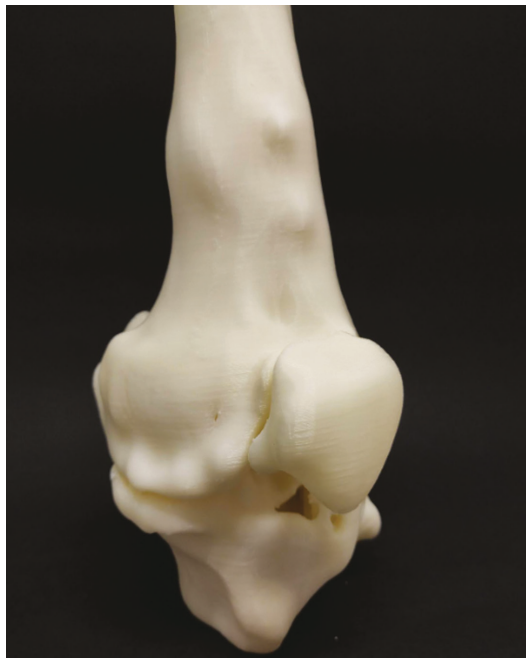
FIGURE 21.5 3D printed model of a knee, including patella, femur, and tibia, manufactured in ABS.
