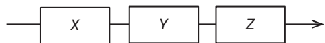
Figure 2.6 A machine consists of three linked systems: each system can “work” or “fail.”
