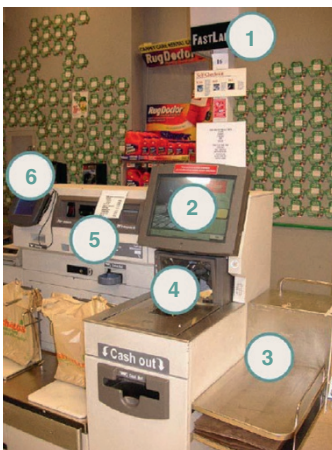
Self-checkout process pieces: 1. Lane light/store attendant call 2. Touch screen monitor 3. Basket stand 4. Barcode scanner cum weighing scale 5. Payment module 6. ATM PIN pad
