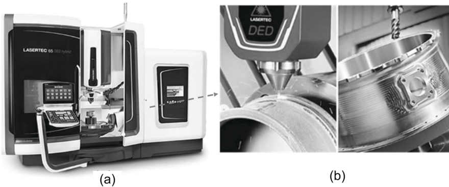
FIGURE 9.3 Laser deposition setup installed onto a CNC milling machine for offline hybrid additive/subtractive manufacturing: (a) DMG Mori Lasertec 65 hybrid manufacturing machine, (b) laser head with five-axis deposition coaxial nozzle (left) and five-axis milling machine (right). Reprinted with permission from Elsevier (Sefene, Hailu, and Tsegaw 2022).
