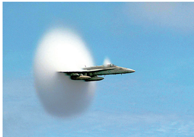
FIGURE 5.26 A cloud sometimes forms just as a plane accelerates to pass—or break—the sound barrier. Moist air is believed to form the cloud's water droplets as air pressure drops behind the shock wave. Source: US Navy photo by John Gay.
