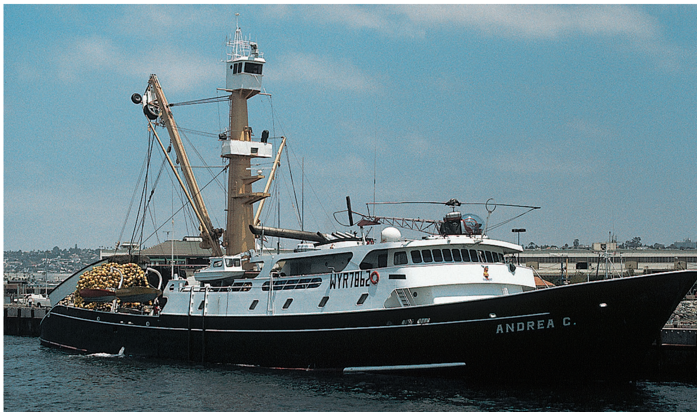
FIGURE 24.11 A modern-day tuna fishing boat. Note the time-tested “crow’s nest” lookout on the mast and the more modern helicopter fastened on top. Both are used to look for schools of tuna, but the helicopter also does other jobs. ©McGraw-Hill Education/Bill Tillery, photographer
