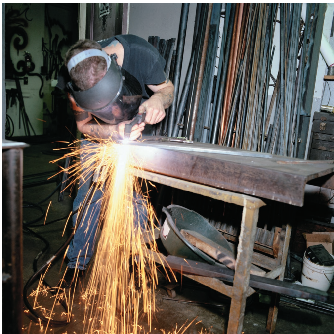
FIGURE 9.9 Acetylene is a hydrocarbon consisting of two carbon atoms and two hydrogen atoms held together by a triple covalent bond between the two carbon atoms. When mixed with oxygen gas, the resulting flame is hot enough to cut through most metals.
