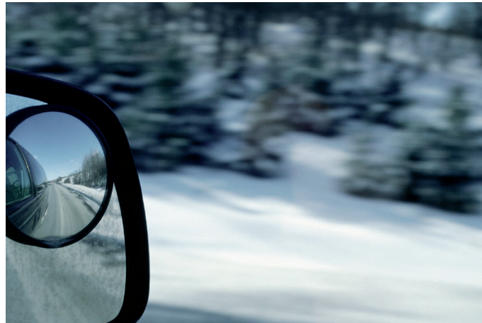
FIGURE 7.13 This convex mirror provides a wide-angle view, increasing your field of vision. ©image 100/Alamy
