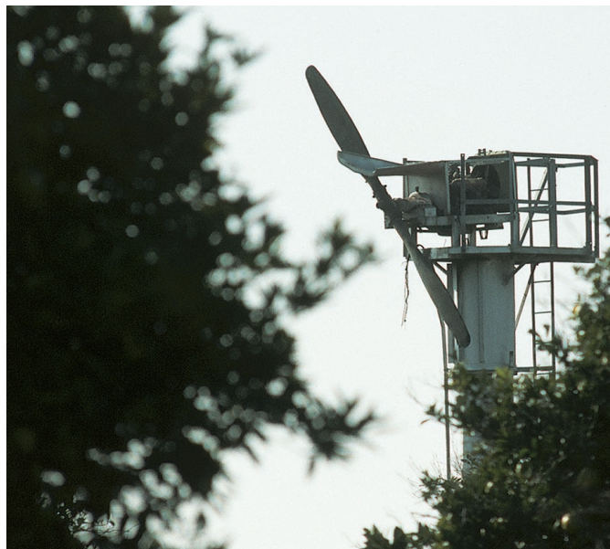
FIGURE 22.16 Fans like this one are used to mix the warmer, upper layers of air with the cooling air in the orchard on nights when frost is likely to form. ©McGraw-Hill Education/Bill Tillery, photographer
