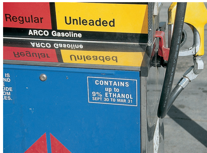
FIGURE 12.15 Gasoline is a mixture of hydrocarbons (C 8 H 18 , for example) that contain no atoms of oxygen. Gasohol contains ethyl alcohol, C 2 H 5 OH, which does contain oxygen. The addition of alcohol to gasoline, therefore, adds oxygen to the fuel. Since carbon monoxide forms when there is an insufficient supply of oxygen, the addition of alcohol to gasoline helps cut down on carbon monoxide emissions.
