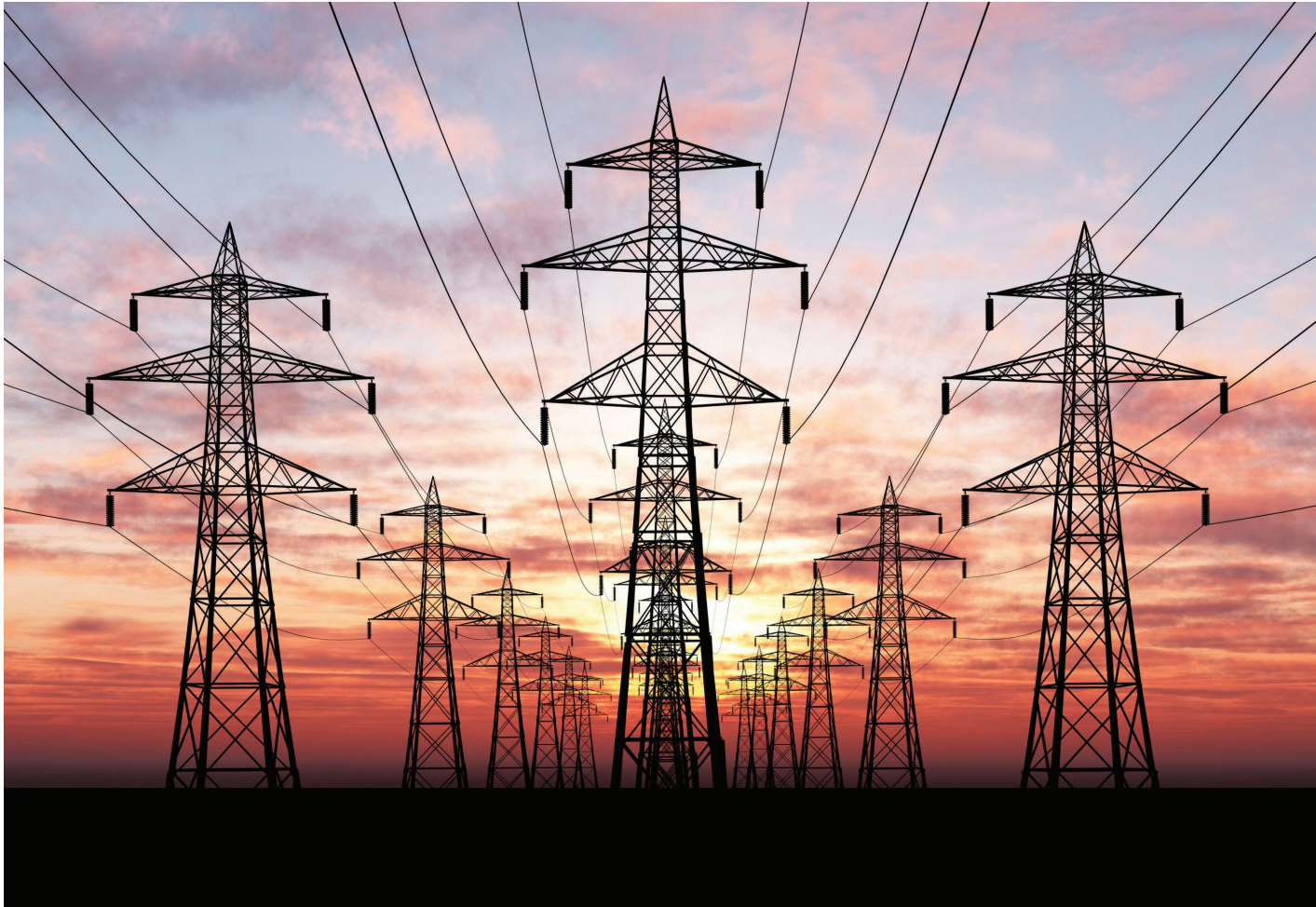
FIGURE 6.13 What is the nature of the electric current carried by these conducting lines? It is an electric field that moves at nearly the speed of light. The field causes a net motion of electrons that constitutes a flow of charge, a current. ©TebNad/Getty Images
