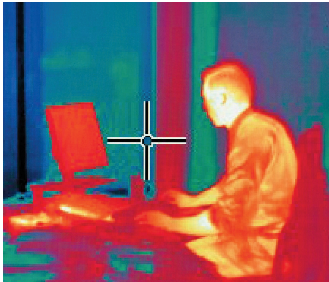
FIGURE 7.4 A special camera is able to capture the infrared energy emitted by an office worker sitting at a desk. This light is invisible to the unaided human eye, but it is real none the less. ©Cultura Creative/Alamy Stock Photo
