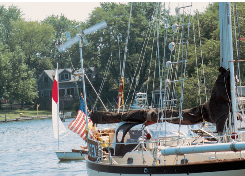
FIGURE 3.21 Wind is another form of solar energy. This wind turbine generates electrical energy for this sailboat, charging batteries for backup power when the wind is not blowing. In case you are wondering, the turbine cannot be used to make a wind to move the boat. In accord with Newton's laws of motion, this would not produce a net force on the boat. ©McGraw-Hill Education/Bill Tillery, photographer
