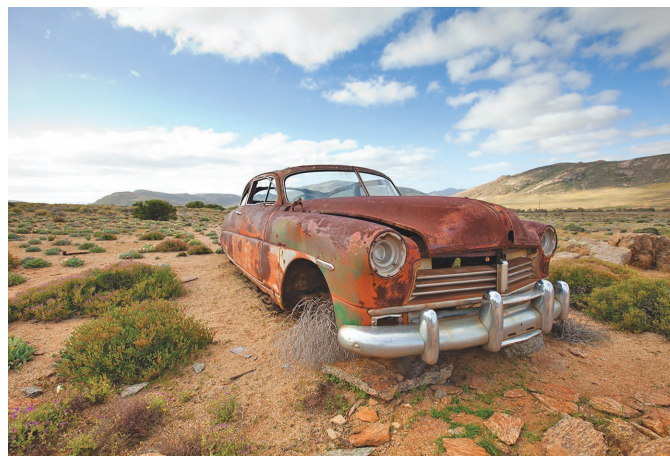
FIGURE 10.10 Rusting iron is a common example of a combination reaction, where two or more substances combine to form a new compound. Rust is iron(III) oxide formed on this old car from the combination of iron and oxygen under moist conditions.
