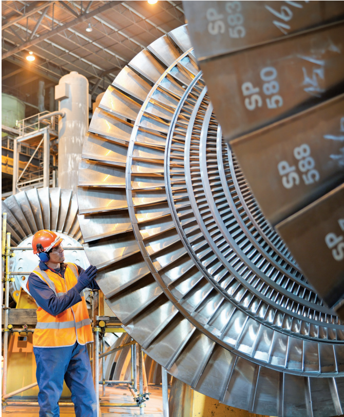
FIGURE 3.15 The blades of a steam turbine. In a power plant, chemical or nuclear energy is used to heat water to steam, which is directed against the turbine blades. The mechanical energy of the turbine turns an electric generator. Thus, a power plant converts chemical or nuclear energy to mechanical energy, which is then converted to electrical energy. ©Monty Rakusen/Getty Images
