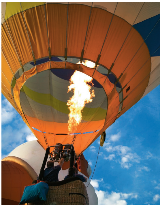
FIGURE 10.7 One of two burners is operating at the moment as this hot air balloon ascends. The burners are fueled by propane ( C_3H_8 ), a liquefied petroleum gas (LPG). Like other forms of petroleum, propane releases large amounts of heat during the chemical reaction of burning. ©Open Door/Alamy
