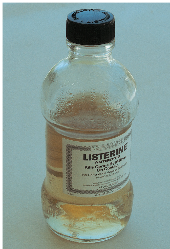
FIGURE 4.22 The inside of this closed bottle is isolated from the environment, so the space above the liquid becomes saturated. While it is saturated, the evaporation rate equals the condensation rate. When the bottle is cooled, condensation exceeds evaporation and droplets of liquid form on the inside surfaces. ©McGraw-Hill Education/Bill Tillery, photographer
