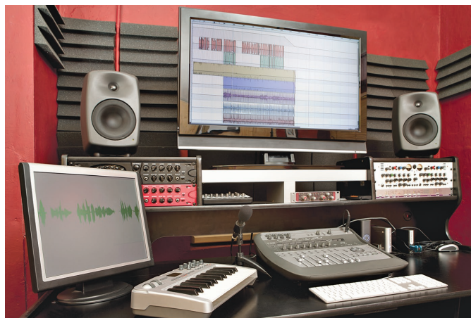
FIGURE 5.14 This multi-media control room is acoustically enhanced by covering portions of the walls with sound-absorbing baffles. Reverberation and echoes cannot occur in this treated room because absorbed sounds are not reflected. ©Oktay Ortakcioglu/Getty Images
