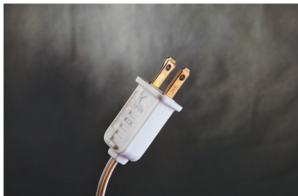
FIGURE 6.39 This is the so-called “polarized” plug, with one prong larger than the other. The larger prong can fit only in the larger slot of the outlet, so the smaller prong (the current-carrying wire) always goes in the smaller slot. This is a safety feature that, when used correctly, results in the switch disconnecting the current-carrying wire rather than the ground wire. ©Deborah Van Kirk/Alamy Stock Photo
