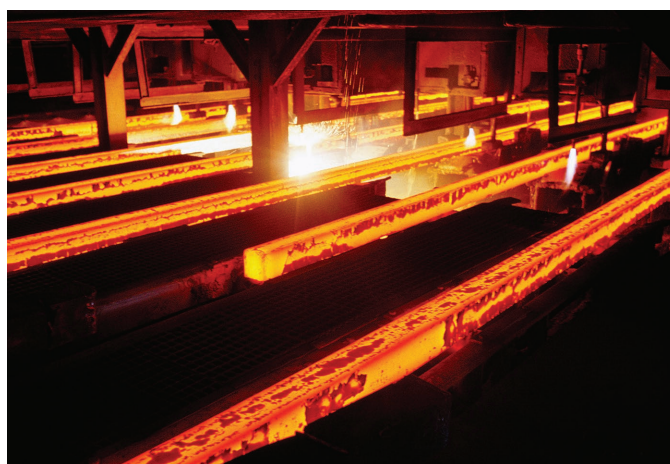
FIGURE 4.1 Heat and modern technology are inseparable. These glowing steel slabs, at over 1,100°C (about 2,000°F), are cut by an automatic flame torch. The slabs are converted to sheet steel for use in the automotive, appliance, and building industries. ©Glow Images
