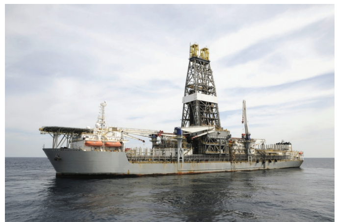
FIGURE 18.1 This drilling ship samples sediment and rock from the deep ocean floor. It can only sample materials well within the upper crust of Earth, however, barely scratching the surface of Earth's interior. ©Brad Martin/Getty Images
