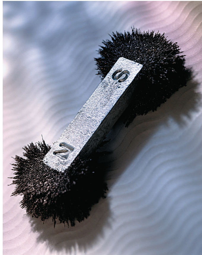
FIGURE 6.18 Every magnet has ends, or poles, about which the magnetic properties seem to be concentrated. As this photo shows, more iron filings are attracted to the poles, revealing their location. ©Steve Cole/Photodisc/Getty Images
