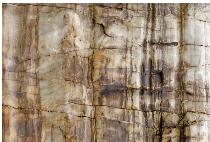
FIGURE 17.21 This is a sample of marble, a coarse-grained metamorphic rock with interlocking calcite crystals. The calcite crystals were recrystallized from limestone during metamorphism. ©Imagemore/Glow Images
