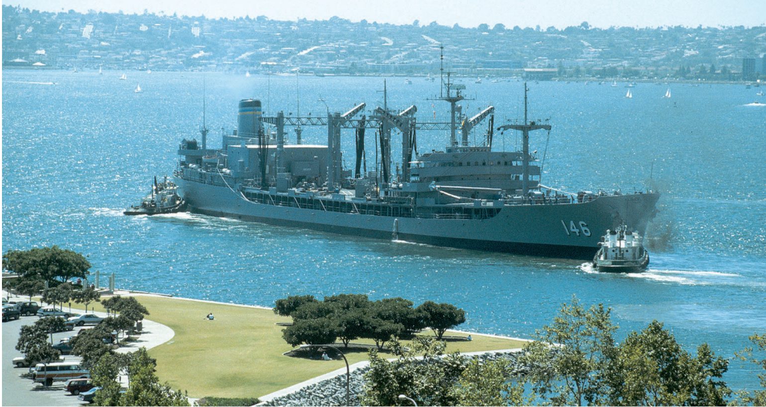
FIGURE 2.7 The rate of movement and the direction of movement of this ship are determined by a combination of direction and size of force from each of the tugboats. In which direction are the two tugboats pushing? What evidence would indicate that one tugboat is pushing with a greater force? If the tugboat by the numbers is pushing with a greater force and the back tugboat is keeping the back of the ship from moving, what will happen? ©McGraw-Hill Education/Bill Tillery, photographer
