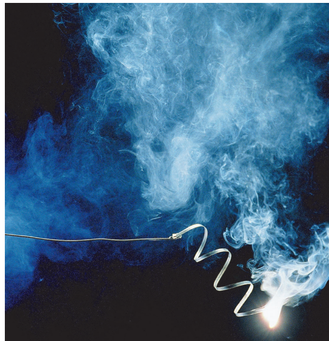
FIGURE 9.3 Magnesium is an alkaline earth metal that burns brightly in air, releasing heat and light. As chemical energy is released, new chemical substances are formed. One new chemical material produced here is magnesium oxide, a soft, powdery material that forms an alkaline solution in water (called milk of magnesia ).
