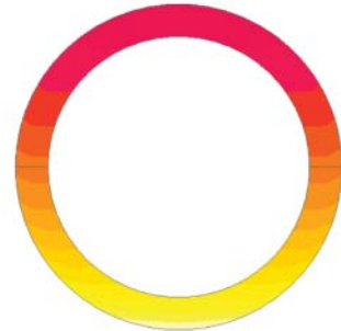
Figure 8.9 Loss density around copper conductor of radius a = 0.01 m.
