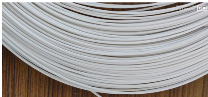
Fig. 4.5 Representative extruded H60 feedstock filament [5]
