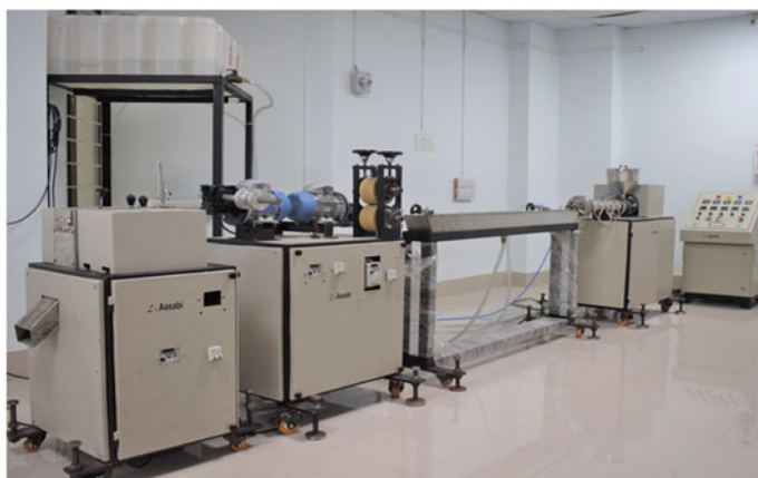
Fig. 4.4 a Schematic representation of the industrial-scale single-screw extruder and b experimental setup
