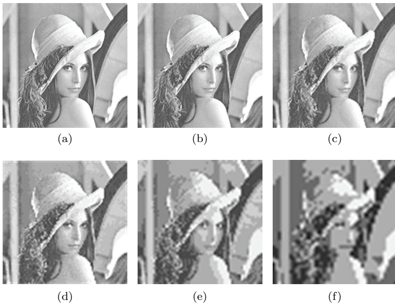
Figure 2.14. Effect of simultaneous changes in image spatial resolutions and gray levels.
