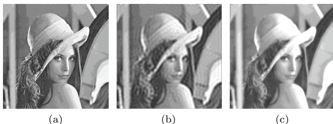
Figure 4.7. Frequency domain low-pass filtering to eliminate false contours.
