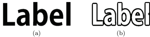
Figure A.4. An application example of the combination of dilation and logic operations.
