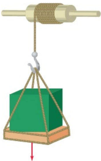
Figure 10-50 Motor overhauling load.
