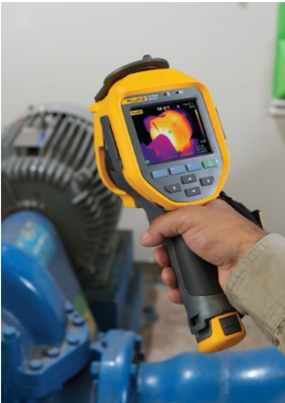
Figure 2-42 Motor thermal imaging inspection.
