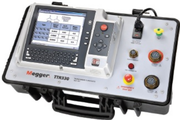
Figure 3-20 Transformer turns ratio test set.
