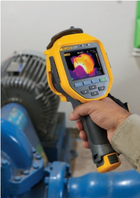
Figure 2-42 Motor thermal imaging inspection.
