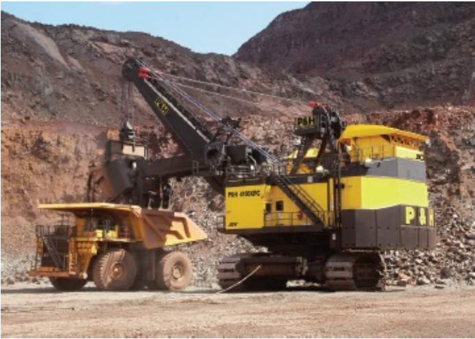
Figure 10-38 Electric mining shovel—DC drive.
