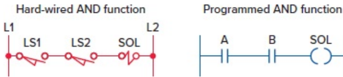
Figure 9-61 Hard-wired circuit and the equivalent PLC logic program for an AND logic control function.
