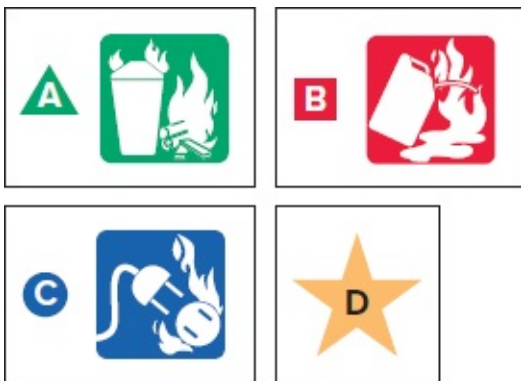
Figure 1-21 Types of fire extinguishers and their applications.
