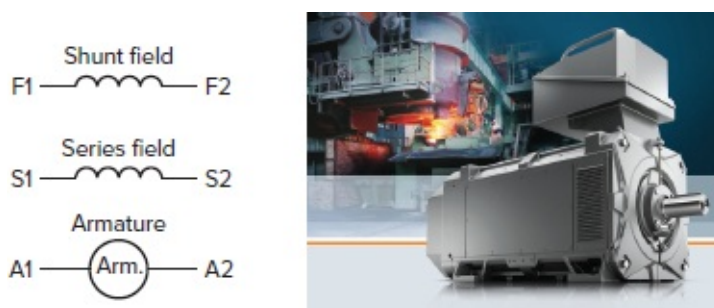
Figure 2-27 Parts of a DC compound motor.
