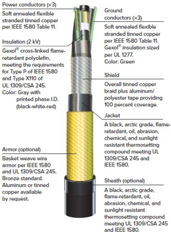
Figure 10-20 VFD shielded power cable.
