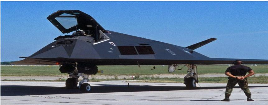
**Figure 16.15** The complicated shaping of F-117A- for purposes of RCS reduction.
