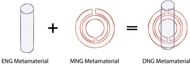
**Figure 1.4** Combination of thin metallic strip wire and SRR to form double negative material.
