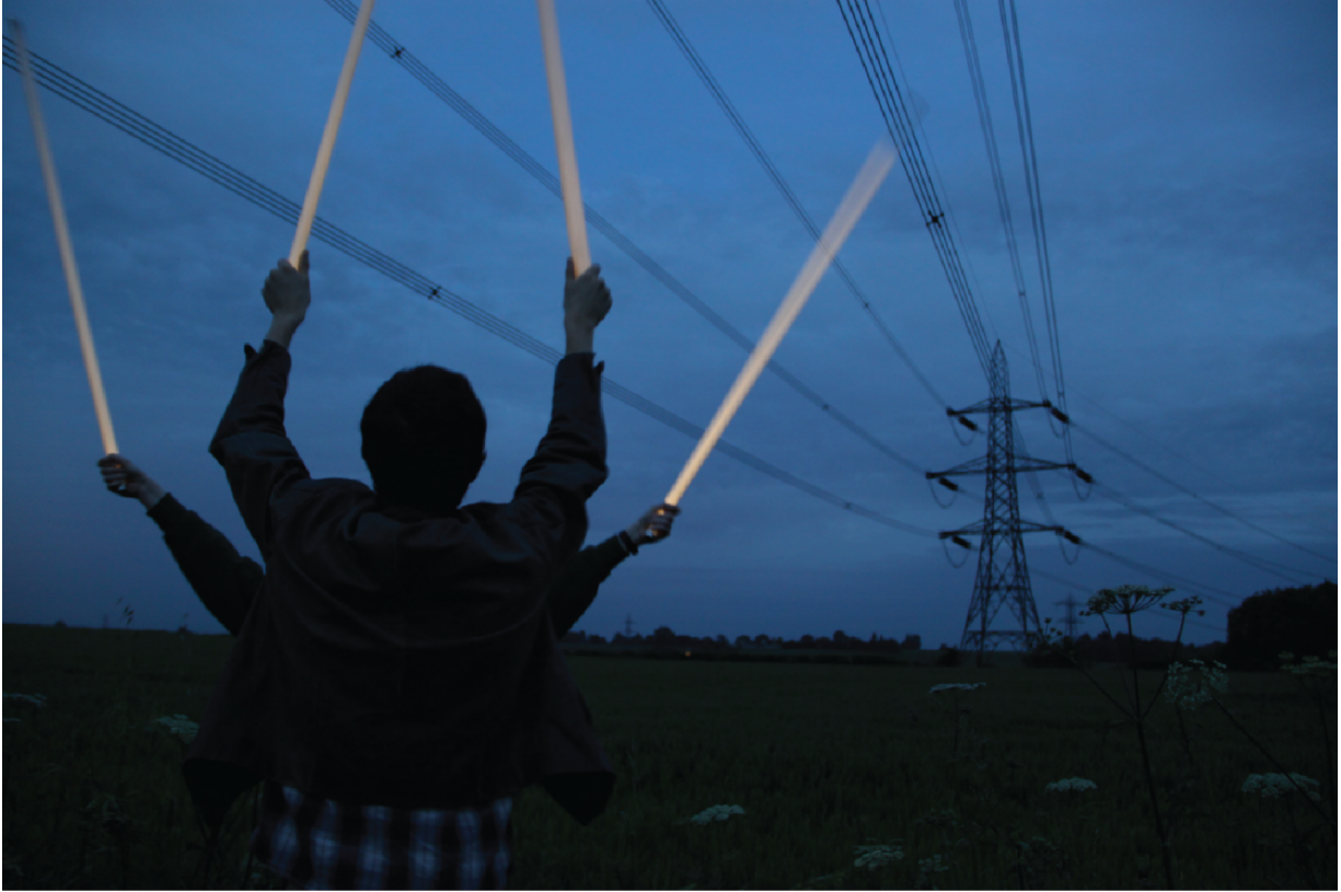
Figure 6.7 Fluorescent tubes illuminated by harvesting energy from the electromagnetic wave around a power transmission line.
