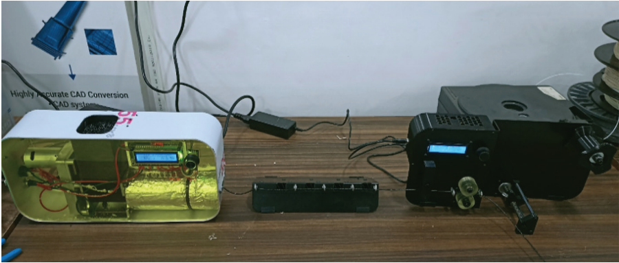
FIGURE 6.7 Wire extrusion using SSE.
