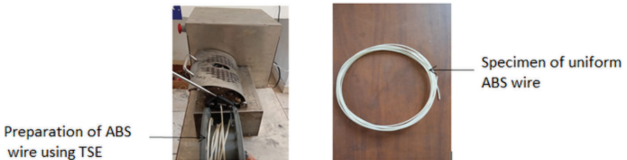
FIGURE 2.5 (a) Extrusion process of ABS filament (b) Extruded ABS filament.
