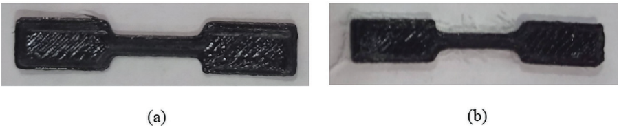
FIGURE 6.8 Dumbbells printed (a) TPU only, (b) TPU + Fabric.
