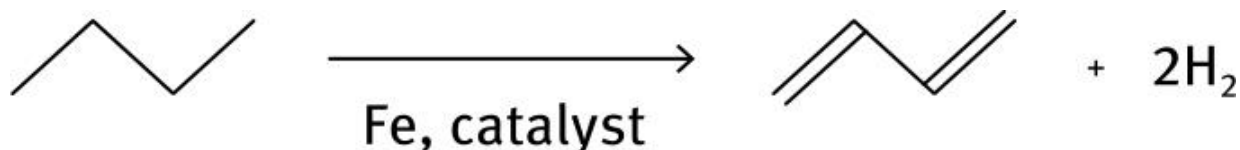
Figure 12.6 Butadiene Production from Butane.
