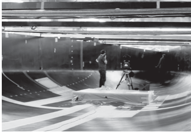
Figure 6.5 Surface patches on the hull marked and scanned
