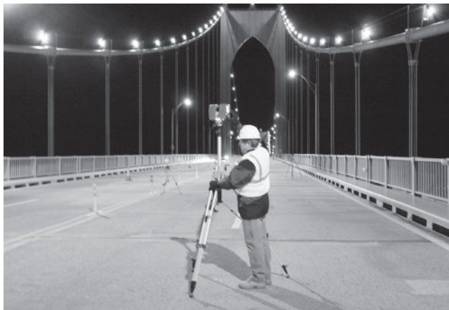
Figure 7.19 Adjusting scanner at fixed spacing intervals and heights to control scan density of road surface
