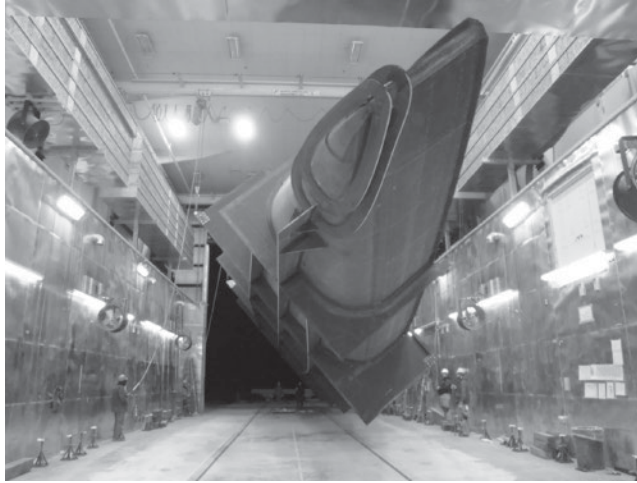
Figure 6.4 The ship's hull hung, allowing access to all areas of its hull for scanning
