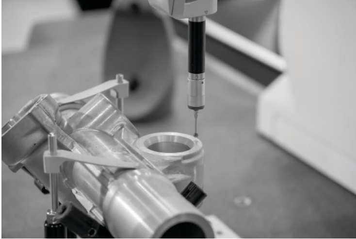
Figure 3.3 Probe tip of a CMM measuring a machined part
