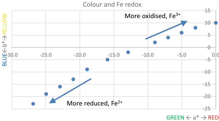
Fig. 5.2 CIELAB colour coordinates for different iron redox states. The coordinates are for glasses of total fixed iron (0.1 wt%) but varying Fe 2+ :Fe 3+ ratios; Fe 3+ concentrations are increasing in 0.01 wt % steps from left to right. The y-axis measures the blue (–): yellow (+), while the x-axis measures the green (–) to red (+) ratio. The z-axis out of the page represents intensity. Very oxidised glasses are yellow, very reduced glasses are blue; most commercial glasses green
