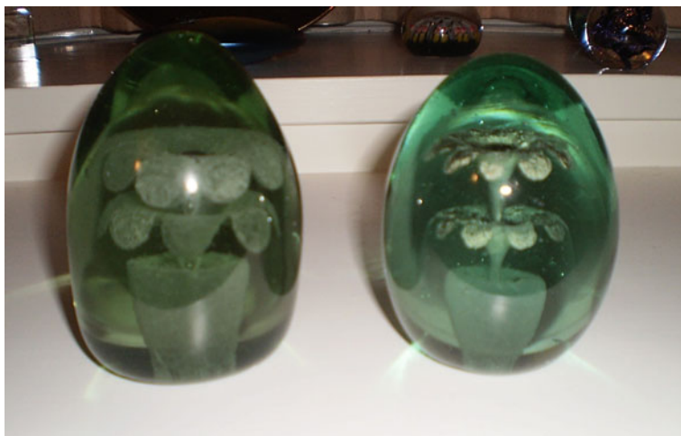
Fig. 5.1 Victorian dump (paperweight) made from glass left over in the crucible at the end of the working day (left). The green tint arises from iron present as an impurity. The paperweight on the right is a modern copy coloured using chromium
