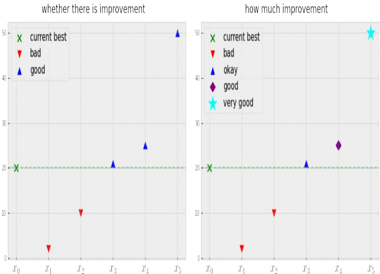
Figure 7.7. The difference between Probability of Improvement (left) and Expected Improvement (right). The former only cares whether we improve from the incumbent or not, while the latter considers how much improvement is made.
