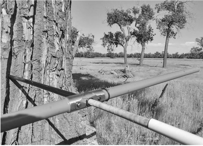
Figure 3 A tree-ring sample is extracted from a plains cottonwood ( Populus deltoides ssp. monilifera ) on the Yellowstone River floodplain in Montana using an increment borer and then stored for transport in a white paper straw. Photo by Derek School.
