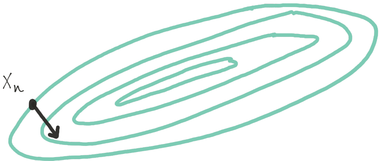
Figure 7: Steepest descent with highly correlated parameters.
