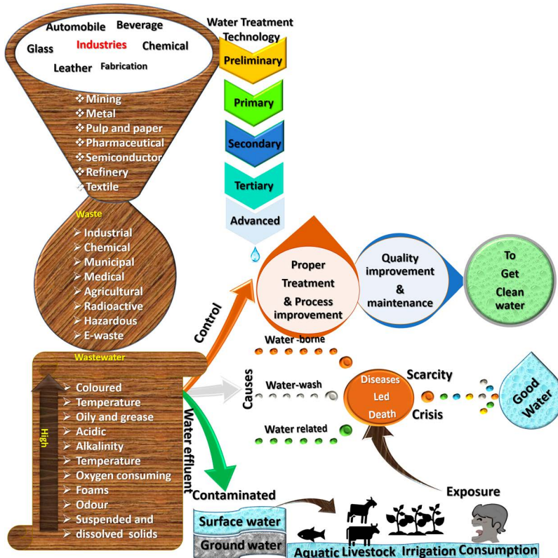
Figure 18.1 Causes and effects of water pollutants from various industries as well as relevant waste water treatment methods and management systems.
