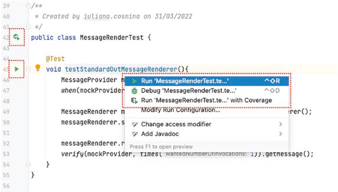
Figure 4-5. IntelliJ IDEA options for running tests
