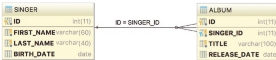
Figure 6-1. Simple data model for the example code
