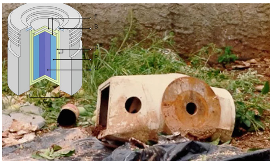
Fig. 3 The remains of the treatment machine head. The inset on the left shows a schematic drawing of the source, which is usually 1.5–3 cm in diameter
