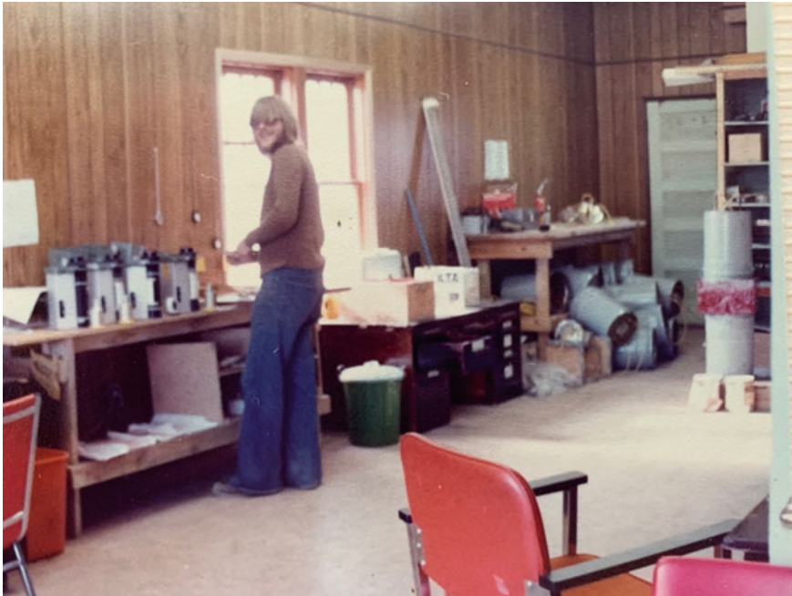
Fig. 1 The author doing an experiment to test concrete sealants to prevent radon from entering homes. The experimental apparatus can be seen on the right; large paint cans sealed to concrete slabs that had been coated with different applications of sealant. Enough uranium ore, hand-harvested prospector style, in the countryside surrounding Uranium City, to create about 5 \times 10^5 Bq/l of radon gas, was in the bottom can and then the gas collected in the top can was measured
