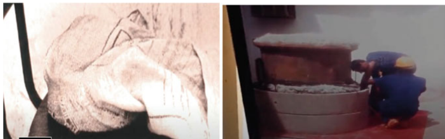
Fig. 7 On the left is a picture of the bag containing the source and, on the right the concrete container quickly built to house the remains of the source
