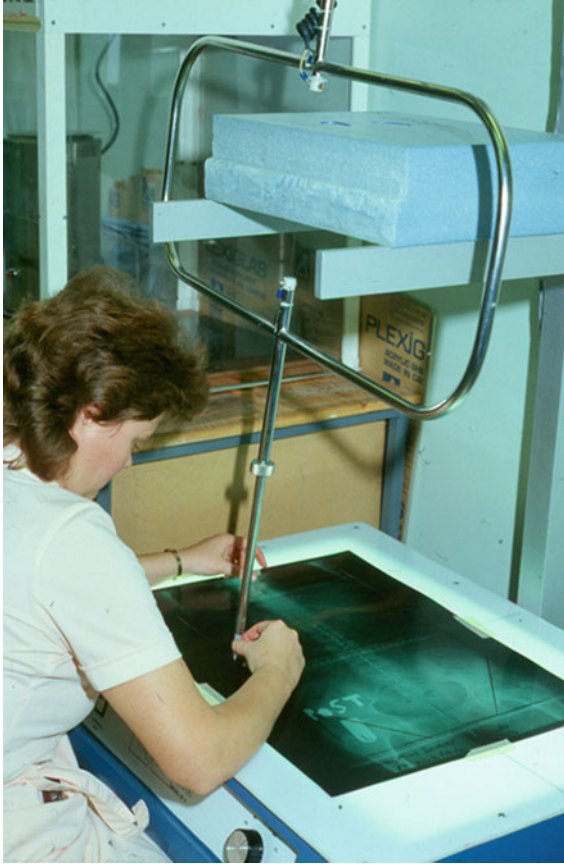
Fig. 1 Technician tracing field outline on x-ray film using the hot-wire cutter. The sections cut out of the Styrofoam will be filled with Cerrobend shielding
