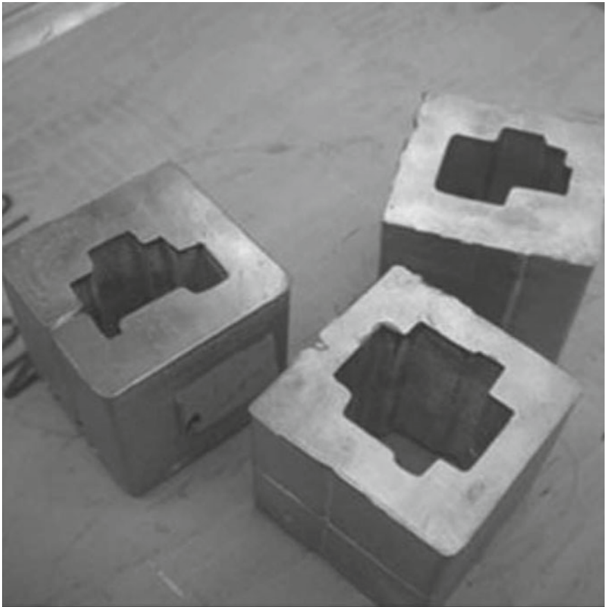
Fig. 2 Low melting point metal alloy blocks designed specifically for each patient and each radiation treatment field
