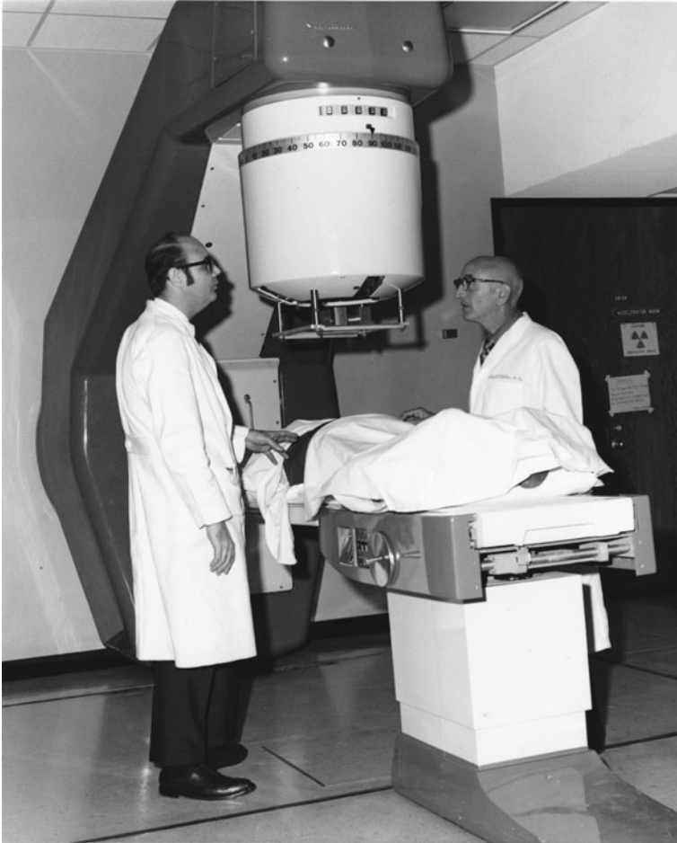
Fig. 4 Drs. Lindberg and Fletcher standing on the moveable portion of the floor. Note the treatment couch mounted in the reverse position with the top portion rotated 180 degrees and cantilevered over the moveable floor. This photo was taken from just inside the entrance
