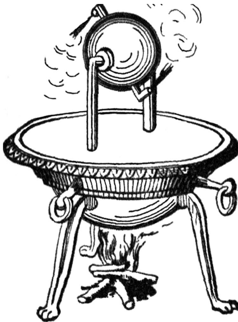
FIGURE 5 A sketch of the aeolipile , as devised by Ctesibius ( https://commons.wikimedia.org/wiki/File:Hero%27s_Aeolipile,_1st_century_AD,_Alexandria_%28reconstruction%29.jpg ).
