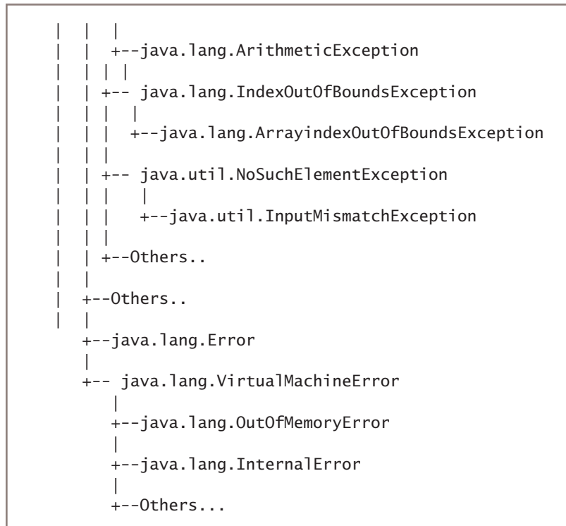
Figure 12-1 The Exception and Error class inheritance hierarchy
