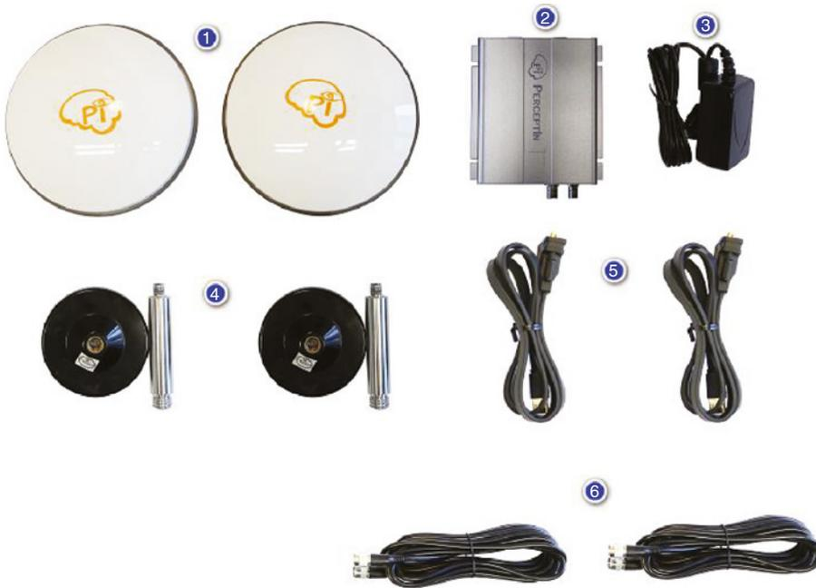
**Figure 5.20** Rover hardware components: 1, GNSS antenna; 2, GNSS receiver module; 3, power supply (5 V); 4, magnetic foundation plate; 5, serial to USB connector; and 6, GNSS antenna cable (TNC male to TNC male).
