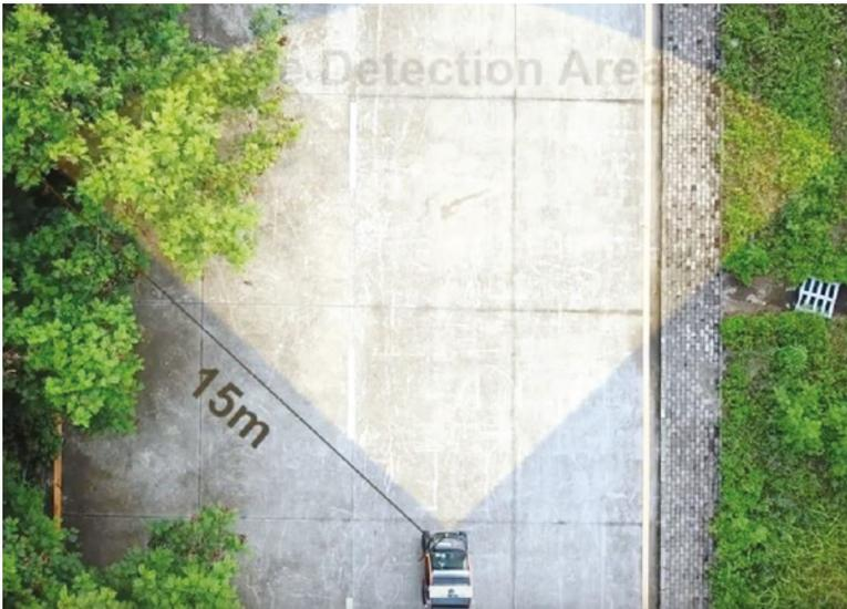
Figure 4.4 Detection range of mmWave radar.
