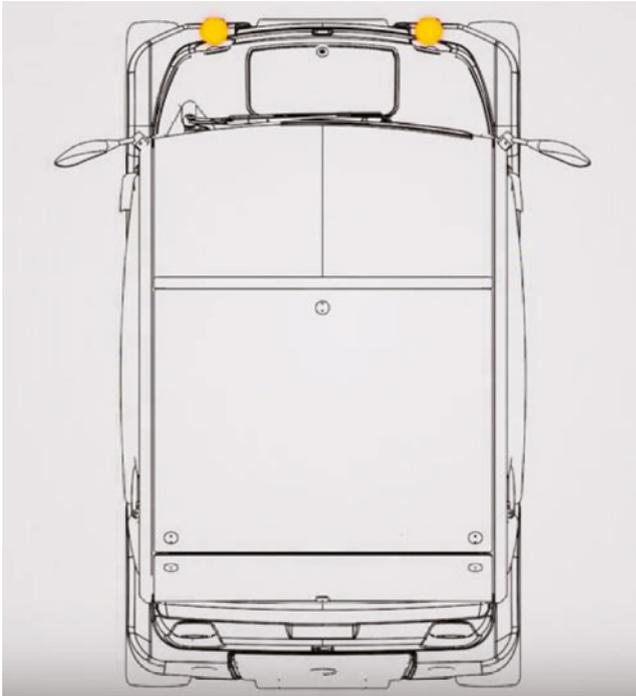
**Figure 4.8** Sample configuration of sonar.
