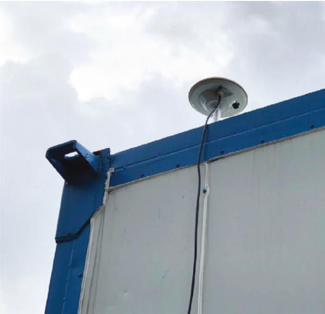
**Figure 5.12** Placement of a GNSS base station antenna.
