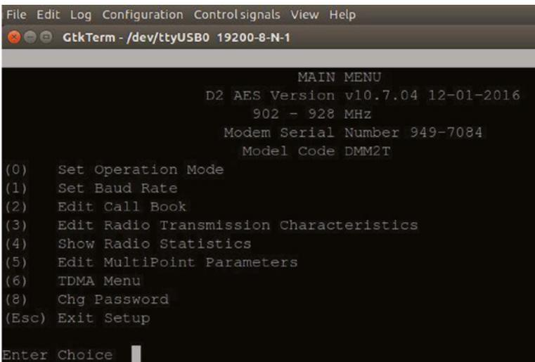
Figure 5.27 900MHz or 2.4GHz radio programming screen on GtkTerm.
