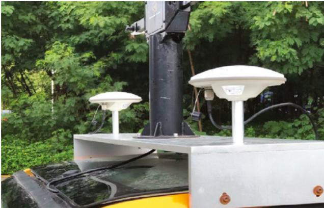
**Figure 5.21** Rover station antenna installation.
