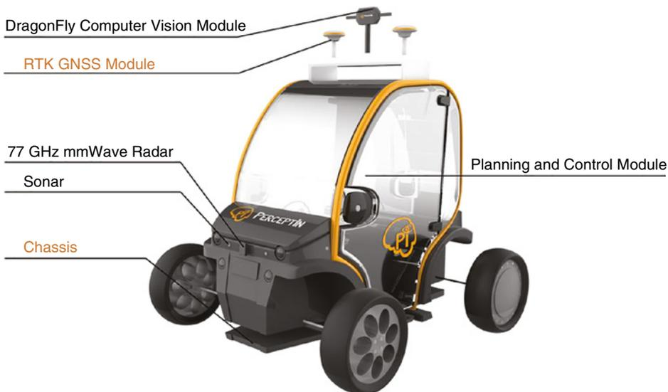
**Figure 1.2** Modular design of a DragonFly Pod.
