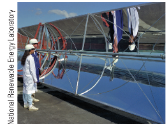
A solar thermal parabolic trough.
