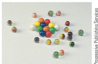
Figure 15.2 A mixture of magnetic marbles with nonmagnetic ones results in the separation of the two different kinds of marbles.
