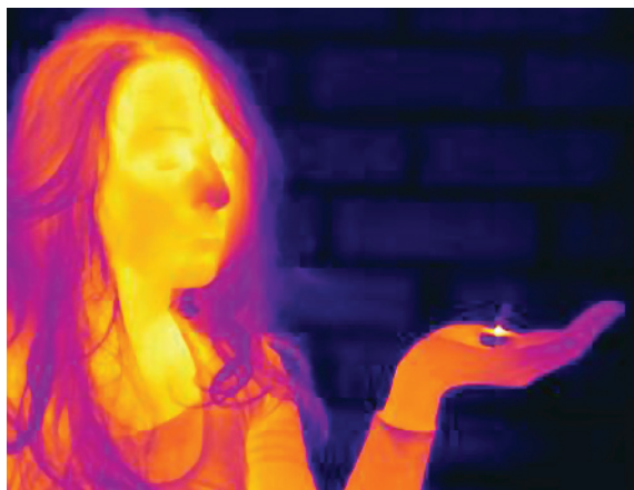
Infrared image of a person in the dark. The infrared light emitted by all warm objects can be “seen” with an infrared camera.
