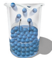
Figure 12.4 Molecules in a liquid, undergoing constant random motion, may acquire enough energy to overcome attractions with neighbors and fly into the gas phase.
