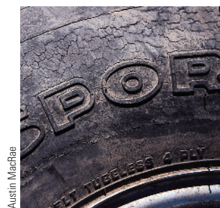
The cracking of rubber products, such as this automobile tire, are primarily caused by the formation of ozone and PAN.
