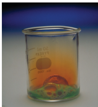
Acids dissolve some metals. Here nitric acid is dissolving the copper that composes a penny. The green-blue color of the solution is due to Cu 2+ ions in solution. The Cu 2+ ions are formed as the copper dissolves. (Pennies were composed of mostly copper until 1983.)
