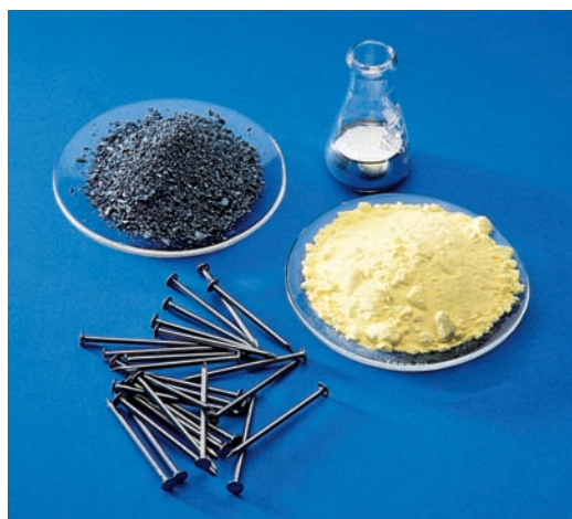
Figure 8.2 One-mole samples of iron (nails), iodine crystals, liquid mercury, and powdered sulfur.
