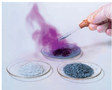
Figure 7.7 When powdered aluminum and iodine (shown in the foreground) are mixed (and a little water added), they react vigorously.
