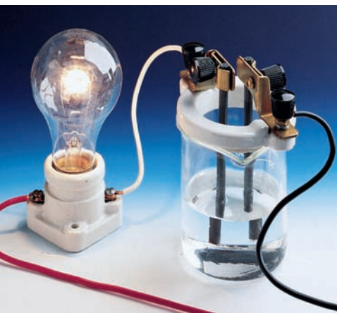
A hydrochloric acid solution readily conducts electric current, as shown by the brightness of the bulb.
