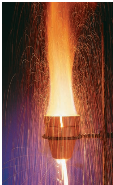
Figure 7.6 The thermite reaction gives off so much heat that the iron formed is molten.
