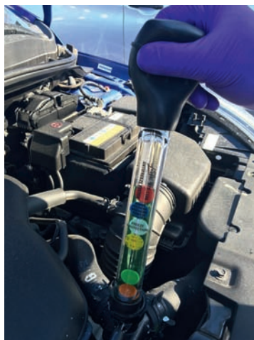
Figure 2.11 A hydrometer being used to determine the density of the antifreeze solution in a car's radiator.
