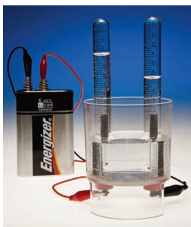
Figure 18.10 The electrolysis of water produces hydrogen gas at the cathode (on the right) and oxygen gas at the anode (on the left). A nonreacting strong electrolyte such as \text{Na}_2\text{SO}_4 is needed to furnish ions to allow the flow of current.
