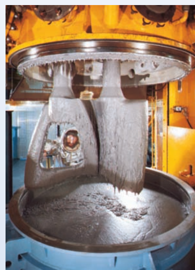
Figure 7.10 A mix bowl mixing propellant for a rocket motor.
