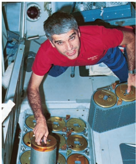
Astronaut Sidney M. Gutierrez changes the lithium hydroxide canisters on the Space Shuttle Columbia .
