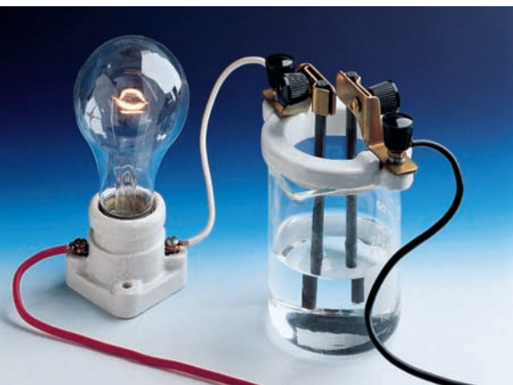
An acetic acid solution conducts only a small amount of current, as shown by the dimly lit bulb.
