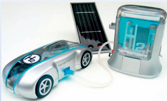
Even model cars are becoming “green.” The H-racer from Horizon Fuel Cell Technologies uses a hydrogen–oxygen fuel cell.
