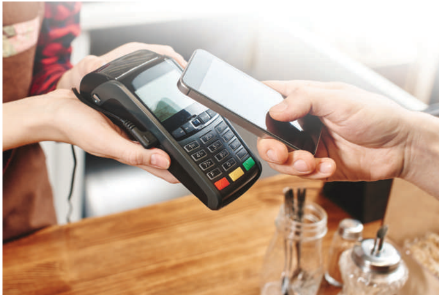
Figure 10.3 Contactless Payment Payment is made just by holding a smartphone near the reader.
