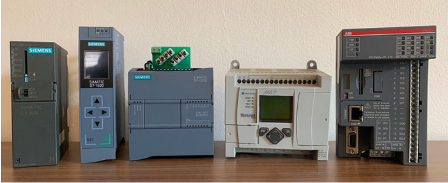
Fig. 5 PLCs procured for experimental purposes including, from left to right, Siemens S7-300, S7-1500, S7-1200, Allen-Bradley MicroLogix 1100, and ABB PM554-TP-ETH
