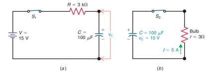
through the 3- $\Omega$  r of the bulb at the start of the decay. Then  $v_{\rm C}$  and  $i_{\rm C}$  drop to zero in five time constants.
