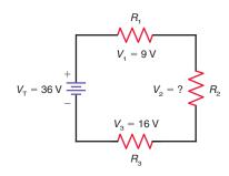
**4-19** MultiSim In Fig. 4–32, solve for the individual resistor voltage drops. Then, using Kirchhoff's voltage law, find  $V_{\rm T}$ .
