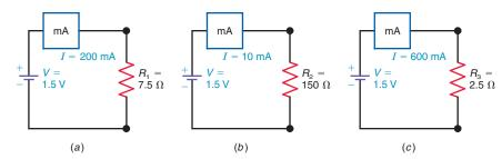
Figure 12–17 illustrates three different cases of using the applied voltage of 1.5 V from a dry cell. In Fig. 12–17*a*, the load resistance  $R_1$  is 7.5  $\Omega$ . Then *I* is 1.5/7.5 =  $\frac{1}{5}$  A or 200 mA.
