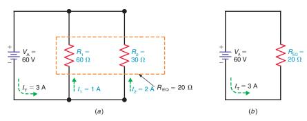
The total load connected to the source voltage is the same as though one equivalent resistance of  $20~\Omega$  were connected across the main line. This is illustrated by the equivalent circuit in Fig. 5–6b. For any number of parallel resistances of any value, use the following equation,
