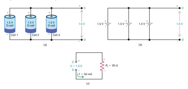
drain of 100 mA. Bad cells should not be connected in parallel with good cells, however, since the cells in good condition will supply more current, which may overload the good cells. In addition, a cell with lower output voltage will act as a load resistance, draining excessive current from the cells that have higher output voltage.
