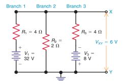
**Figure 10–17** The same circuit as in Fig. 9–5 for Kirchhoff's laws, but shown with parallel branches to calculate  $V_{XY}$  by Millman's theorem.
