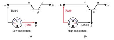
**Figure 28–10** Testing the collector-base junction of a transistor with an analog ohmmeter. (a) Low resistance is measured because the analog meter forward-biases the collector-base junction. (b) High resistance is measured because the analog meter reverse-biases the collector-base junction.
