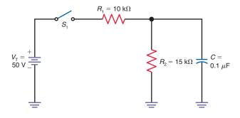
**22–43** Refer to Fig. 22–21. (a) How long will it take C to fully charge after  $S_1$  is closed? (b) What is  $V_C$  1 ms after  $S_1$  is
