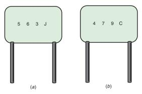
**ANSWER** In Fig. 16–12*a*, the first two numbers are 5 and 6, respectively, for 56 as the first two digits in the numerical value of the capacitance. The third number, 3, indicates a multiplier of 1000, or  $56 \times 1000 = 56,000$  pF. The letter J indicates a capacitor tolerance of  $\pm 5\%$ .
