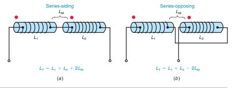
the series-aiding connection. Let this be  $L_{\rm T_a}$ . Then the connections to one coil are reversed to measure the total inductance for the series-opposing coils. Let this be  $L_{\rm T_a}$ . Then
