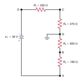
**4-48** In Fig. 4–47, solve for  $V_{AG}$ ,  $V_{BG}$ , and  $V_{CG}$ .
