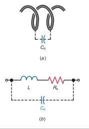
Special methods for minimum  $C_{\rm d}$  include space-wound coils, where the turns are spaced far apart; the honeycomb or universal winding, with the turns crossing each other at right angles; and the bank winding, with separate sections called pies. These windings are for rf coils. In audio and power transformers, a grounded conductor shield, called a Faraday screen, is often placed between windings to reduce capacitive coupling.
