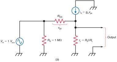
signal is applied to the gate, whereas the output is taken from the source. Notice that there is no drain resistor. Since the drain is tied directly to  $V_{\rm DD}$ , it is at ground for AC signals.
