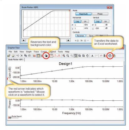
Once the plot is selected, the data can be exported to an Excel worksheet by mouse clicking on the Excel icon in the upper right hand side of the tool bar, as shown in Fig. F–81. The export feature will create a new worksheet with the X and Y data in adjacent columns. Figure F–82 shows data from the generic oscilloscope captured by the Grapher.
