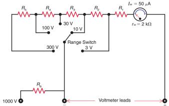
Note: When using the 1000 V jack, the range switch is set to 300 V.
