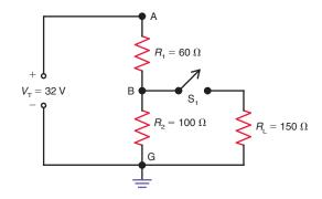
**7-27** With  $S_1$  closed in Fig. 7–30, which resistor has only the bleeder current,  $I_{\rm B}$ , flowing through it?
