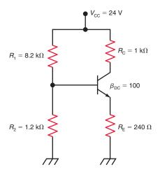
**28-37** Draw a DC load line for the transistor circuit in Fig. 28–28, and indicate the values of  $I_{\text{C(sat)}}$ ,  $V_{\text{CE(off)}}$ ,  $I_{\text{CQ}}$ , and  $V_{\text{CEQ}}$  on the load line.
