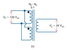
that is approximately 5 to 10% higher than its rated value. Let's use the transformer in Fig. 19–14a as an example. It has a rated secondary current of 2 A. If 120 V is connected to the primary and no load is connected to the secondary, each half of the secondary will measure somewhere between 13.2 and 13.9 V approximately. However, with the rated current of 2 A drawn from the secondary, each half of the secondary will measure approximately 12.6 V.
