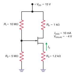
**30–19** In Fig. 30–29, solve for  $I_{\rm D}$  and  $V_{\rm D}$ .
