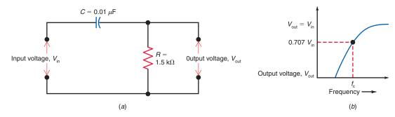
Figure 26–17 RL high-pass filter. (a) Circuit. (b) Graph of  $V_{\text{out}}$  versus frequency.
