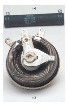
Chap. 11, "Conductors and Insulators." The insulated core is commonly porcelain, cement, or just plain pressed paper. Bare wire is used, but the entire unit is generally encased in an insulating material. Typical fixed and variable wire-wound resistors are shown in Fig. 2–3.
