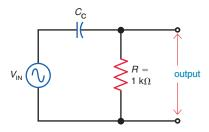
**18–39** In Fig. 18–29, assume that  $C_{\rm C}=0.047~\mu{\rm F}$  and R=1 $k\Omega$ , as shown. For these values, what is the lowest frequency of the applied voltage that will provide an  $X_{c}$ of 100  $\Omega$ ? At this frequency, what is the phase angle,  $\theta_7$ ?
