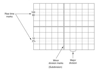
calibrated at some set value—for example, 5 mV/Div., 10 mV/Div., or 2 V/Div. This allows the scope to be used for peak-to-peak voltage measurements of the vertical input signal. Dual-trace scopes have a separate variable control for each channel.
