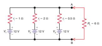
**Figure 12–37** Circuit diagram for Critical Thinking Prob. 12–19.
