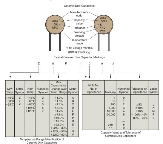
**Figure 16–14** Ceramic disk capacitor for Example 16–8.
