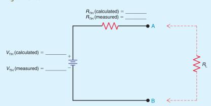
The magic in Thevenin's theorem lies in the fact that the Thevenin equivalent circuit driving terminals A and B remains the same regardless of the value of  $R_{\rm L}$ . In the original circuit of Fig. 10–48, every time  $R_{\rm L}$  was changed the entire circuit would have to be resolved. Not with Thevenin's theorem! Just plug the new value of  $R_{\rm L}$  into the Thevenin equivalent circuit, and make one simple calculation.
