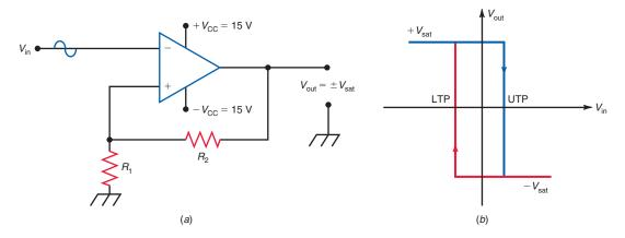
switches to  $+V_{\rm sat}$ . When  $V_{\rm in}$  drops below +5 V,  $V_{\rm out}$  switches to  $-V_{\rm sat}$ . The transfer characteristic is shown in Fig. 33–25b. In fact  $V_{\rm ref}$  can be either positive or negative. The reference voltage is usually obtained by attaching a resistive voltage divider to either  $+V_{\rm CC}$  or  $-V_{\rm CC}$ . In some cases, it may even be desirable to have an adjustment that allows the reference voltage to vary.
