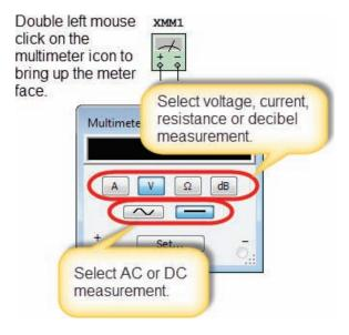
then "DC" or "AC" measurement. Every circuit must have a ground. Figure F–49 contains a Quick Hint on the use of the generic multimeter.
