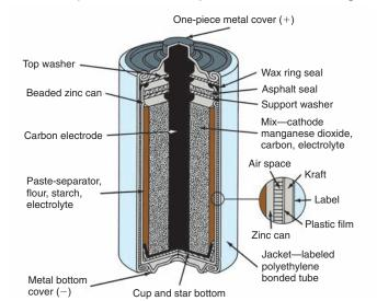
Figure 12-4 Cutaway view of carbon-zinc dry cell. This is size D with a height of 2<sup>1</sup>/<sub>4</sub> in.
