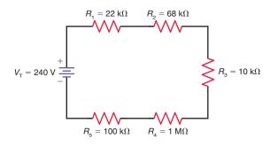
**4-9** Recalculate the values for  $R_{\rm T}$  and I in Fig. 4–27 if  $R_{\rm 4}$  is changed to 100 k $\Omega$ .
