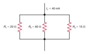
**7-19** In Fig. 7–24, solve for  $I_1$ ,  $I_2$ , and  $I_3$ .
