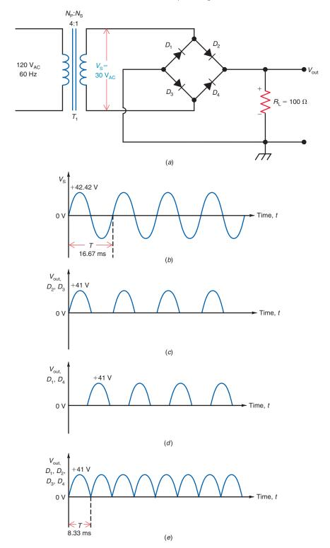
**Figure 27–20** Full-wave bridge rectifier showing diodes  $D_1$  and  $D_4$  reverse-biased during positive alternation of secondary voltage. Each diode in the bridge must withstand a peak inverse voltage that is 0.7 V less than the peak value of the full secondary voltage.
