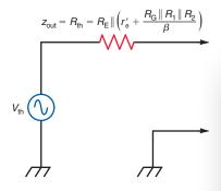
where  $R_{\rm G}$  represents the internal resistance of the AC generator driving the base of the emitter follower. The derivation of this equation is quite complex and is therefore not covered here. However, Fig. 29–10 represents the Thevenin equivalent circuit for the output of an emitter follower. Since the circuit is assumed to be predominantly resistive,  $z_{\rm out}$  can also be designated as  $R_{\rm th}$ . A typical emitter follower has an output impedance of 10  $\Omega$  or less.
