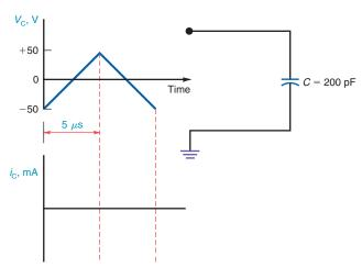
18-43 In Fig. 18-33, show the corresponding charge and discharge current for the waveshape of capacitor voltage shown.
