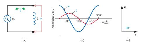
The voltage across L in this circuit is determined by the applied voltage, since they must be the same. The inductive effect here is to make the current have values that produce L(di/dt) equal to the parallel voltage.
