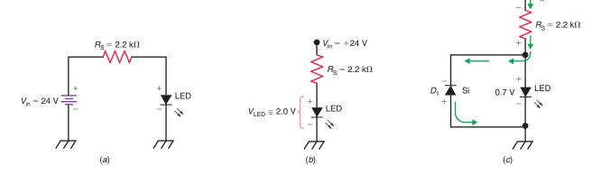
Figure 27–24*b* shows how the circuit of Fig. 27–24*a* is normally drawn in commercial schematics. It is common practice to show only the potential difference and its polarity with respect to chassis ground.
