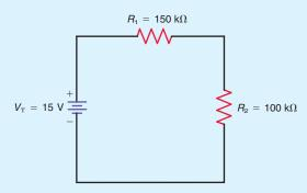
Construct the series circuit in Fig. 8–36. With your analog VOM set to the 10-V range, measure and record the voltage across  $R_2$ :  $V_2 =$
