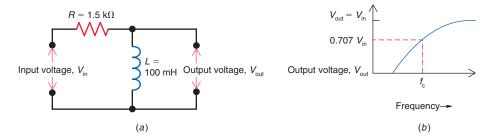
At very low frequencies, the output voltage approaches zero because the ratio  $R/Z_{\rm T}$  becomes very small as  $X_{\rm C}$  and thus  $Z_{\rm T}$  approach infinity. At very high frequencies,  $V_{\rm out}$  is approximately equal to  $V_{\rm in}$ , because the ratio  $R/Z_{\rm T}$  approaches one as  $Z_{\rm T}$  and R become approximately the same value.
