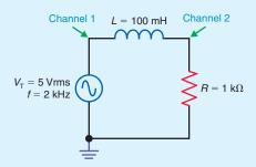
Construct the circuit in Fig. 21–36. Set the total voltage,  $V_{\rm T}$ , to 5 Vrms and the frequency, f, to 2 kHz. Using a DMM, measure and record the following circuit values:
