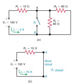
**Figure 6–14** Effect of an open path in a series-parallel circuit. (a) Normal circuit with  $S_2$  closed. (b) Series circuit with  $R_1$  and  $R_2$  when  $S_2$  is open. Now  $R_3$  in the open path has no current and zero IR voltage drop.
