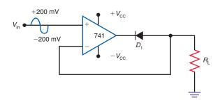
**33–55** What is the output in Fig. 33–45 if a 100- $\mu$ F capacitor is connected at the output?
