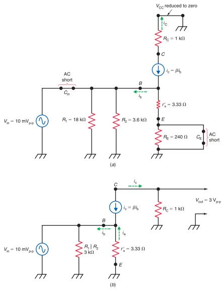
In Fig. 29–5b the output equals the AC voltage across the collector resistor,  $R_{\rm C}$ . This can be expressed as
