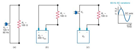
Also, if you connect the same  $R_{\rm L}$  across the 200-V<sub>DC</sub> source in Fig. 26–3b, instead of using the AC source, the steady direct current in  $R_{\rm L}$  will be  $^{200}/_{100}$ , or 2 A. The battery source voltage and its current are considered steady DC values because there are no variations.
