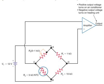
temperature drops back to 25°C, the resistance of the thermistor increases to its original value, thus causing the voltage  $V_{\rm CD}$  to return to 0 V. This shuts off the air conditioner.
