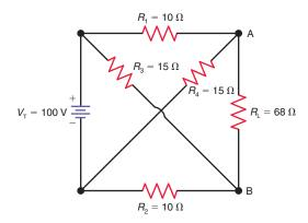
**10–43** In Fig. 10–47, use the superposition theorem to solve for  $I_{\rm L}$  and  $V_{\rm L}$ .
