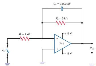
**33–43** Calculate the cutoff frequency,  $f_{\rm C}$ , for the circuit in Fig. 33–39.
