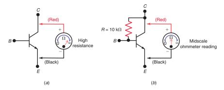
of the ohmmeter be used. These limits will produce the most reliable results. This test is rather crude, but it does provide a unique way of testing for transistor action.
