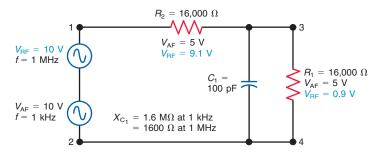
the applied voltage, equal to the 5 V across  $R_2$  and 5 V across  $R_1$ . This 5 V at 1000 Hz is also present across  $C_1$ , since it is in parallel with  $R_1$ .
