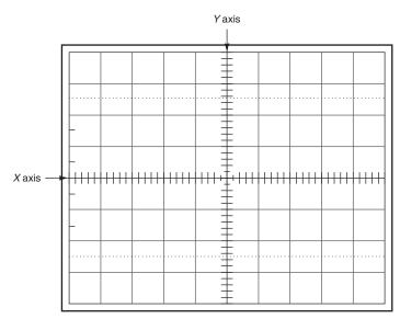
Figure E-8 Oscilloscope screen (graticule).
