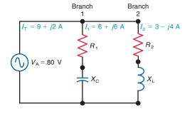
Note that  $I_1$  has +j for the  $+90^{\circ}$  of capacitive current, and  $I_2$  has -j for inductive current. These current phasors have signs opposite from their reactance phasors.
