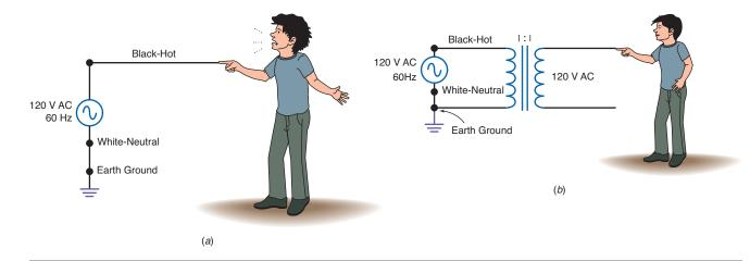
with just one lead of the transformer secondary, there is no path back to earth ground to complete the circuit and as a result, no electric shock.
