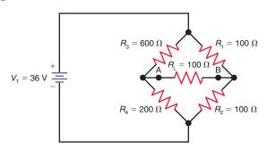
**10–22** Using the Thevenin equivalent circuit for Fig. 10–34, calculate the values for  $I_{\rm L}$  and  $V_{\rm L}$ .
