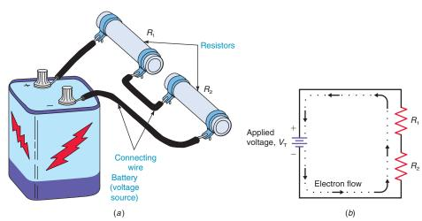
**Figure 4–1** A series circuit. (a) Pictorial wiring diagram. (b) Schematic diagram.
