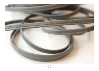
duty insulation jacket as compared to those designed for indoor use only. Although outdoor extension cords can always be used indoors, indoor extension cords should never be used outdoors! Also, never use an extension cord whose insulation is damaged or compromised. Exposed strands of copper wire present a safety hazard to those working in and around the area where the extension cord is being used.
