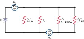
**5–59** In Fig. 5–37, solve for  $V_A$ ,  $I_1$ ,  $I_2$ ,  $I_4$ ,  $R_1$ ,  $R_3$ , and  $R_{EQ}$ .
