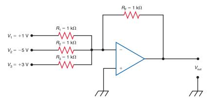
Because the inverting input has zero current, all of the input currents combine to flow through the feedback resistor,  $R_{\rm F}$ . Because  $R_1 = R_2 = R_3 = R_{\rm F}$ , the voltage gain of the circuit is one and the output voltage is
