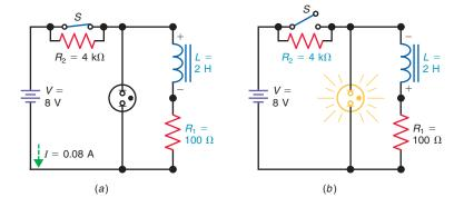
resistance. The steady-state *I* is  $V/R_1 = {}^{8}\!/_{100} = 0.08$  A. This value of *I* is reached after five time constants.
