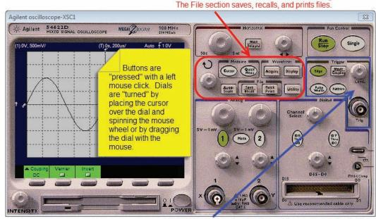
The Trigger controls when the oscilloscope starts to display the waveform. It can start the display on the rising or falling edge. The voltage level at which the oscilloscope is triggered is also selected here.
