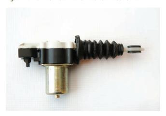
Figure 14-26 shows a solenoid valve used to control the flow of refrigerant in a commercial refrigerator. It should be noted that in many cases the coil assembly and valve body are two separate pieces.
