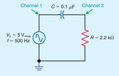
Construct the circuit in Fig. 18–37. Set the total voltage,  $V_T$ , to 5 V rms and the frequency, f, to 500 Hz. Using a DMM, measure and record the following circuit values:
