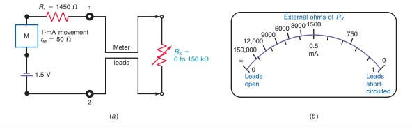
Note that the ohm scale increases from right to left. This arrangement is called a *back-off scale*, with ohm values increasing to the left as the current backs off from full-scale deflection. The back-off scale is a characteristic of any ohmmeter where the internal battery is in series with the meter movement. Then more external  $R_{\rm X}$  decreases the meter current.
