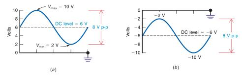
In Fig. 26–4*b*, all values are negative. Notice that here the positive peak of the AC component subtracts from the DC level because of opposite polarities. Now the negative peak adds to the negative DC level to provide a maximum point of negative voltage.
