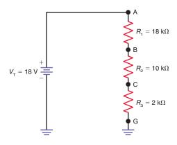
**4-46** In Fig. 4–45, solve for  $V_{AG}$ ,  $V_{BG}$ , and  $V_{CG}$ .
