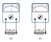
capacitor action, shows that the capacitor can store charge, indicating a normal capacitor. Note that both the rise and the fall of the meter readings are caused by charging. The capacitor discharges when the meter leads are reversed.
