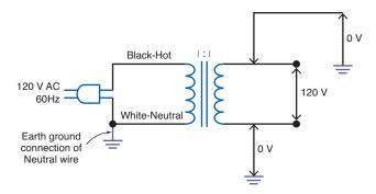
**Fig. 19-35** This illustration shows how an isolation transformer lessens the likelihood of an electric shock. (a) Accidently touching the hot wire of the  $120\text{-V}_{AC}$  power line while in contact with earth ground results in a severe electric shock or even electrocution. (b) Touching only one secondary lead of an isolation transformer while in contact with earth ground does not result in an electric shock.
