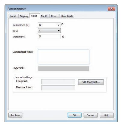
or decrease of resistance is set by the user in the configuration screen. The associated key is also set in the configuration screen, as shown in Fig. F–18.
