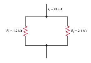
**7-14** Multi*Sim* In Fig. 7–19, solve for  $I_1$  and  $I_2$ .
