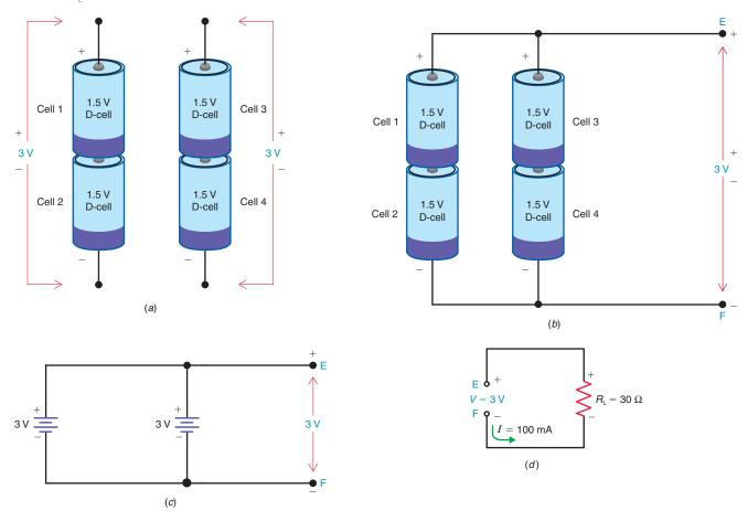
To double the current capacity, another string is connected in parallel. The two strings in parallel have the same 3-V output as one string, but with a current capacity of  $\frac{1}{2}$  A instead of the  $\frac{1}{4}$  A for one string.
