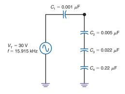
**18–41** In Fig. 18–31, calculate  $V_{c_1}$ ,  $V_{c_2}$ , and  $V_{c_3}$ .
