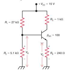
The emitter voltage,  $V_{\rm E}$ , is 0.7 V less than the base voltage,  $V_{\rm B}$ , assuming that the transistor is silicon. This is shown in Formula (28–15):
