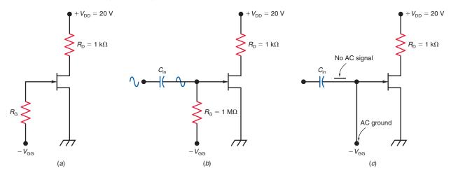
When  $V_{\rm GS}$  is known, the value of the drain current is calculated using Formula (30–2). Then  $V_{\rm DS}$  is calculated as
