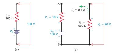
**Figure 12–20** How terminal voltage  $V_L$  drops with more load current. The graph is plotted for values in Table 12–4.
