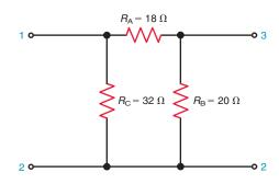
**10–41** In Fig. 10–45, use delta-wye transformations to calculate both  $R_{\rm T}$  and  $I_{\rm T}$ .
