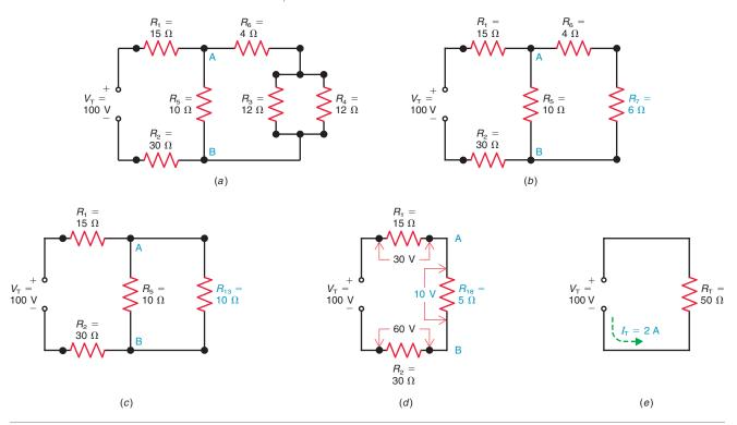
To calculate  $R_{\rm T}$  in Fig. 6–5, the steps are as follows:
