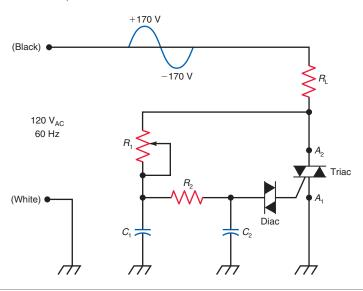
both the positive and negative alternations. As a result, the conduction angle is very small, resulting in only a small amount of AC power delivered to the load,  $R_{\rm L}$ . As  $R_{\rm l}$  is decreased further in value, the triac fires earlier during both alternations. This increases the conduction angle, which means that more AC power will be delivered to the load,  $R_{\rm L}$ .
