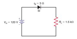
**27–32** In Fig. 27–30, which diode approximations are not necessary when solving for  $I_{\rm L}$  and  $V_{\rm L}$ ? Justify your answer.
