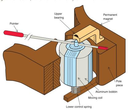
close-up view of the basic components contained within a D'Arsonval meter movement. Notice that the moving coil is wound around a drum which rotates when direct current flows through the wire of the moving coil.
