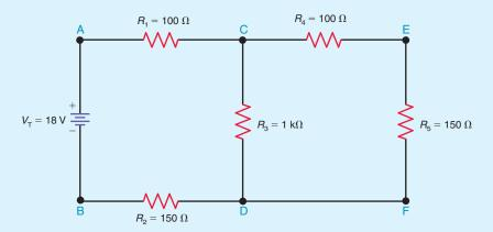
Construct the circuit in Fig. 9–26. Measure and record the following circuit values:
