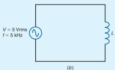
Refer to Fig. 20–17b. With the frequency, f, set to 5 kHz, calculate and record the value of  $X_1$  for each of the following inductance values listed below. Calculate  $X_1$  as  $2\pi fL$ .
