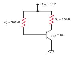
The values in Example 28–12 are shown on the DC load line in Fig. 28–17. Notice that  $V_{\rm CEQ}$  and  $I_{\rm CQ}$  are the same as the  $I_{\rm C}$  and  $V_{\rm CE}$  values calculated in this example, where  $V_{\rm CEQ}=5.48~{\rm V}$  and  $I_{\rm CQ}=4.35~{\rm mA}$ . Remember that  $I_{\rm CQ}$  and  $V_{\rm CEQ}$  represent the quiescent  $I_{\rm C}$  and  $V_{\rm CE}$  values without an AC input signal applied.
