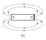
**Figure 13–9** Examples of a closed magnetic ring without any air gap. (a) Two PM horseshoe magnets with opposite poles touching. (b) Toroid magnet.
