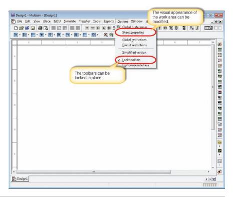
**Sheet Properties** × Sheet visibility Colors Workspace Wiring Font PCB Show grid Uncheck the box to remove the grid of black dots in the work area Custom size A (Letter) Width: 11 \* Orientation 8.5 + Height: Centimeters Inches
