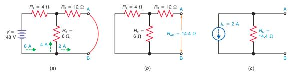
To find  $R_{\rm N}$  in Fig. 10–10b, the short circuit is removed from terminals A and B. Now the source V is short-circuited. Looking back from open terminals A and B, the 4- $\Omega$   $R_{\rm 1}$  is in parallel with the 6- $\Omega$   $R_{\rm 2}$ . This combination is  $^{24}/_{10} = 2.4 \Omega$ . The 2.4  $\Omega$  is in series with the 12- $\Omega$   $R_{\rm 3}$  to make  $R_{\rm AB} = 2.4 + 12 = 14.4 \Omega$ .
