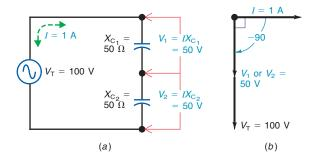
**Figure 23–5** Parallel circuit with  $X_c$  alone. (a) Schematic diagram. (b) Phasor diagram of branch and total line currents and applied voltage.
