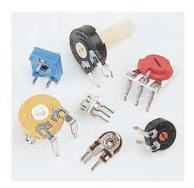
Typical examples of small potentiometers used in electronic circuits are shown in Fig. 2–19.
