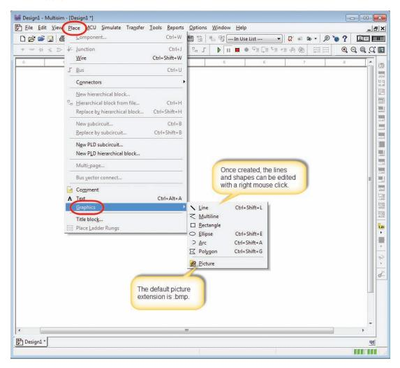
Once the lines or shapes are drawn, they can be modified or repositioned. A right mouse click on a line or shape will cause the Edit menu to open, as shown in Fig. F–88. The properties of the object can be changed in the Edit menu. The line or shape can be repositioned by placing the cursor over the object and holding the left mouse button down while it is dragged to its new location.
