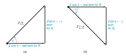
Consider the impedance  $Z/\underline{\theta}$  in polar form. Its value is the hypotenuse of a right triangle with sides formed by the real term and j term in rectangular coordinates. See Fig. 24–9. Therefore, the polar form can be converted to rectangular form by finding the horizontal and vertical sides of the right triangle. Specifically,
