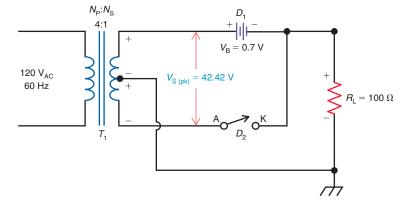
The same analogy can also be used to find the peak inverse voltage across the diode  $D_1$  for the opposite polarity of the secondary voltage. Incidentally, the PIV for  $D_1$  also equals -41.72 V. For any full-wave rectifier using a center-tapped transformer, the PIV for each diode will be 0.7 V less than the peak value of the full secondary voltage.
