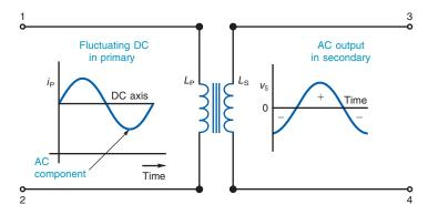
output may be more or less than the AC component in the primary, depending on the turns ratio. This ability to isolate the steady DC component in the primary while providing AC output in the secondary applies to all iron-core and air-core transformers with a separate secondary winding.
