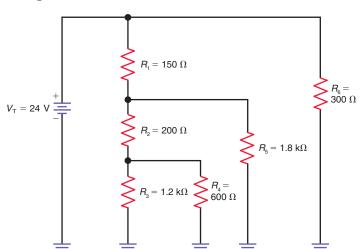
**6–30** In Fig. 6–40, solve for  $R_2$ ,  $V_1$ ,  $V_2$ ,  $V_3$ ,  $I_3$ ,  $I_7$ , and  $V_T$ .
