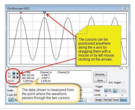
Figure F-62 Voltage measurement with an Agilent oscilloscope.
