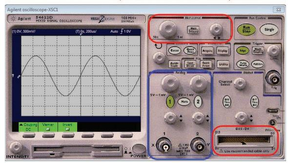
Channels "1" and "2" control the units for the y-axis. The y-axis represents voltage and the units are in volts per division.
