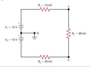
**9–11** In Fig. 9–16, solve for the voltages  $V_{\rm AG}$ ,  $V_{\rm BG}$ ,  $V_{\rm CG}$ ,  $V_{\rm DG}$ , and  $V_{\rm AD}$ . Indicate the proper polarity for each voltage.
