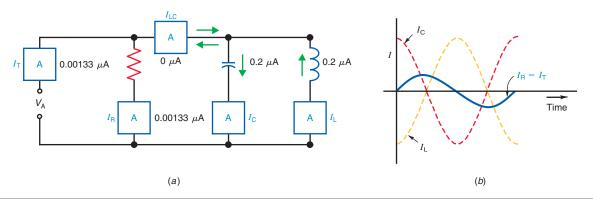
With minimum current in the line, the impedance across the line is maximum at the resonant frequency. The maximum impedance at parallel resonance corresponds to a high value of resistance, without reactance, since the line current is then resistive with zero phase angle.
