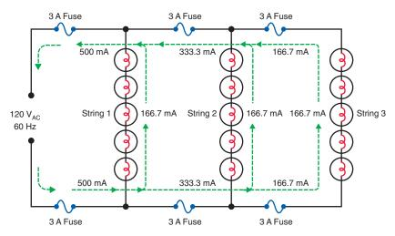
example, if the middle string of lights goes out (dark), the first and last sets will still light. The reason why is that each string of lights is in parallel with the other. If one branch of a parallel circuit opens, the remaining branches are unaffected. This is because the remaining sets of lights are still connected across the  $120\,\mathrm{V}$  power line.
