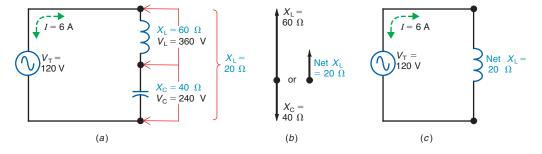
Fig. 23–6c. Then, with 20  $\Omega$  as the net reactance across the 120-V source, the current is 6 A. This current lags the applied voltage  $V_{\rm T}$  by 90° because the net reactance is inductive.
