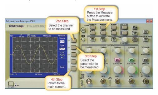
Figure F-70 Tektronix oscilloscope measurement display.
