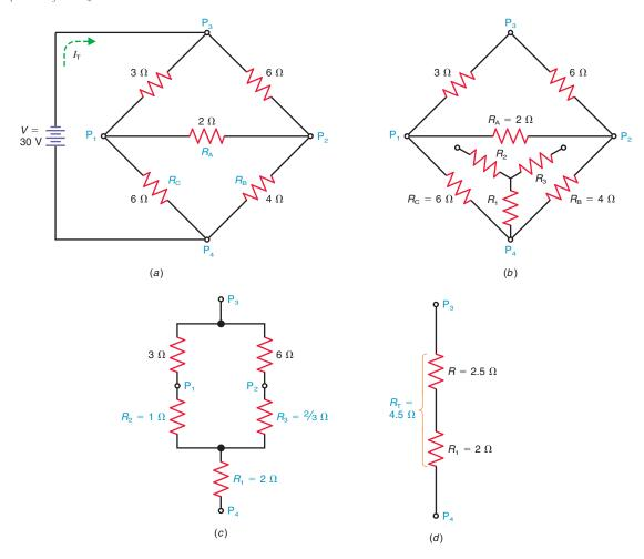
We next use these values for  $R_1$ ,  $R_2$ , and  $R_3$  in an equivalent wye to replace the original delta. Then the resistances form the series-parallel circuit shown in Fig. 10–22c. The combined resistance of the two parallel branches here is  $4 \times 6.67$  divided by 10.67, which equals 2.5  $\Omega$  for R. Adding this 2.5  $\Omega$  to the series  $R_1$  of 2  $\Omega$ , the total resistance is 4.5  $\Omega$  in Fig. 10–22d.
