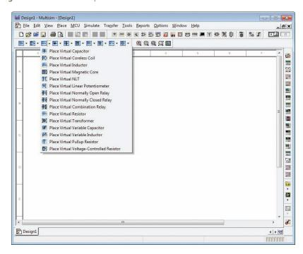
modeled after actual components are limited to real world values. For example, a virtual resistor can have any value resistance and percent tolerance, as shown in Fig. F–13. The configuration screen for each component can be opened by double left mouse click, selecting the component with a single left mouse click and then pressing <Ctrl><M> or selecting the component with a single left mouse click and then choosing "Properties" in the drop-down menu.
