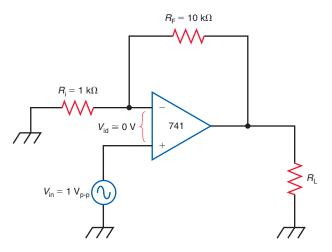
As with the inverting amplifier, the values of  $R_{\rm F}$  and  $R_{\rm i}$  determine the closed-loop voltage gain,  $A_{\rm CL}$ . Because the differential input voltage,  $V_{\rm id}$ , between the op amp input terminals is approximately zero, the current through  $R_{\rm i}$  is found as follows:
