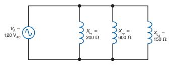
**20–26** In Fig. 20–14, solve for  $L_1$ ,  $L_2$ ,  $L_3$ , and  $L_T$  if the frequency of the applied voltage is 6.366 kHz.
