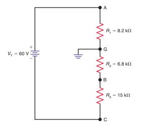
**4-47** In Fig. 4–46, solve for  $V_{AG}$ ,  $V_{BG}$ ,  $V_{CG}$ , and  $V_{DG}$ .
