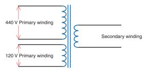
given primary voltage. For example, if 120 V is applied to the lower primary, the upper primary winding is not used. Conversely, if 440 V is applied to the upper primary, the lower primary winding is not used.
