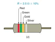
In Fig. 2–9a, the first stripe is red for 2 and the next stripe is green for 5. The red colored decimal multiplier in the third stripe means add two zeros to 25, or multiply the number 25 by  $10^2$ . The result can be illustrated as follows:
