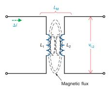
**Figure 19–7** Schematic symbols for two coils with mutual inductance. (*a*) Air core. (*b*) Iron core.
