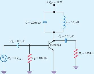
Next, predict the peak-to-peak output voltage across the load  $R_{\rm L}$  if the frequency of  $V_{\rm in}$  equals  $f_{\rm r}$ .  $V_{\rm out(0-p)} =$
