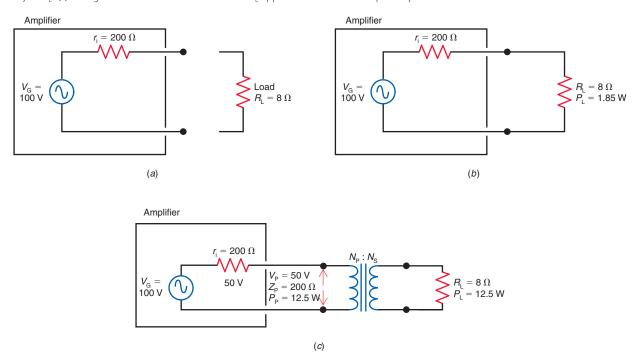
and load are connected directly, as shown in Fig. 19–20*b*, the load receives 1.85 W of power, which is calculated as
