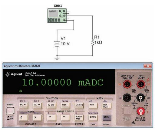
Figure F-57 Agilent multimeter Quick Hint for current measurement.
