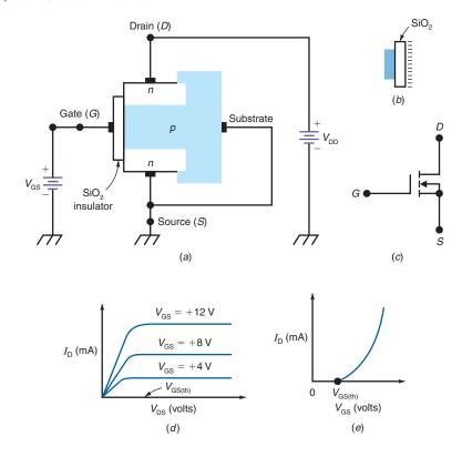
Figure 30–20d shows a typical set of drain curves for the n-channel enhancement-type MOSFET. The lowest curve is the  $V_{\rm GS(th)}$  curve. For more positive gate voltages, the drain current,  $I_{\rm D}$ , increases. The transconductance curve is shown in Fig. 30–20e. Notice that  $I_{\rm D}$  is zero when the gate-source voltage is less than  $V_{\rm GS(th)}$ .
