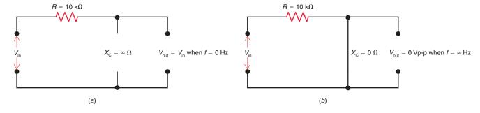
When the frequency of the input voltage is somewhere between zero and infinity, the output voltage can be determined by using Formula (26–1):
