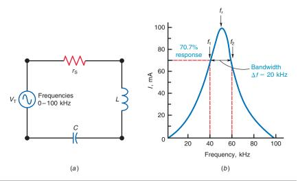
where  $\Delta f$  is the total bandwidth in the same units as the resonant frequency  $f_r$ . The bandwidth  $\Delta f$  can also be abbreviated BW.
