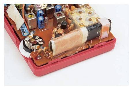
**Figure 21–8** Ferrite-coil antenna for a radio receiver.
