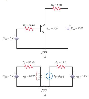
transistors,  $V_{\rm BE}$  equals 0.7 V. Notice that the collector circuit is represented as a current source whose value is dependent only on the values of  $\beta_{\rm DC}$  and  $I_{\rm B}$ . Collector supply voltage variations have little or no effect on the collector current,  $I_{\rm C}$ .
