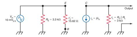
shorts, and the emitter diode has been replaced with its equivalent AC resistance, designated  $r'_e$ . The AC resistance of the emitter diode is calculated as follows:
