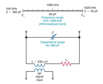
Note that the lowest frequency  $F_{\rm L}$  at 540 kHz is tuned with the highest C at 360 pF. Resonance at the highest frequency  $F_{\rm H}$  at 1620 kHz results from the lowest C at 40 pF.
