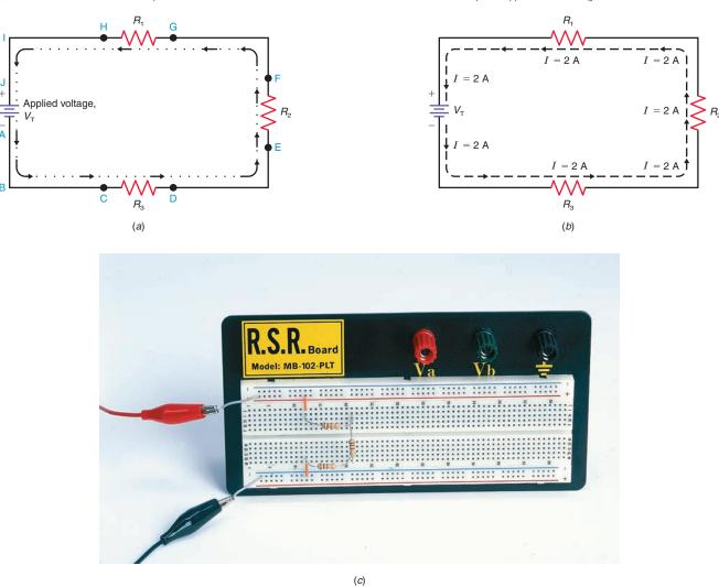
The order in which components are connected in series does not affect the current. In Fig. 4–3b, resistances  $R_1$  and  $R_2$  are connected in reverse order compared with Fig. 4–3a, but in both cases they are in series. The current through each is the same because there is only one path for the electron flow. Similarly,  $R_3$ ,  $R_4$ , and  $R_5$  are in series and have the same current for the connections shown in Fig. 4–3c, d, and e. Furthermore, the resistances need not be equal.
