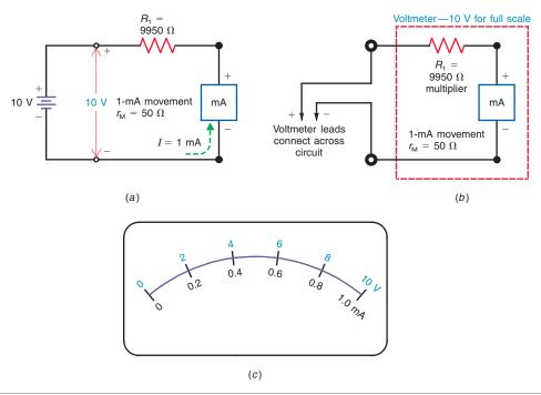
With 1 mA in the meter movement, the full-scale deflection can be calibrated as 10 V on the meter scale, as long as the 9950- $\Omega$  multiplier is included in series with the meter movement. It doesn't matter to which side of the meter movement the multiplier is connected.
