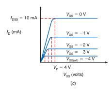
Notice the magnitude of both  $V_{\rm P}$  and  $V_{\rm GS(off)}$  in Fig. 30–5c. It is interesting to note that for any JFET,  $V_{\rm P} = -V_{\rm GS(off)}$ . Most data sheets do not list  $V_{\rm P}$  but almost always list  $V_{\rm GS(off)}$ . The  $V_{\rm GS(off)}$  value of -4 V for the JFET in Fig. 30–5a is a typical value for many JFETs. In Fig. 30–5c,  $V_{\rm P} = -(-4$  V) or  $V_{\rm P} = +4$  V.
