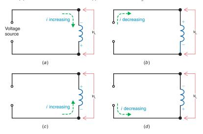
polarity of  $v_L$  can produce current in the same direction, tending to keep the current from decreasing.
