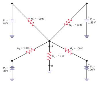
**10–45** Refer to Fig. 10–34. Remove  $R_4$  from the circuit, and show the Thevenin equivalent circuit driving the open terminals. Also, calculate the value of  $I_4$  and  $V_{R_*}$ .
