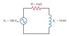
**21–14** In Fig. 21–18, solve for  $Z_T$ , I,  $V_L$ ,  $V_R$ , and  $\theta_Z$ .
