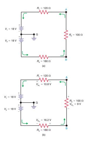
Figure 9–4*b* shows the voltage drops across each resistor. Notice that the polarity of each resistor voltage drop is negative at the end where the electrons enter the resistor and positive at the end where they leave.
