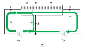
in the collector. If the voltage across the collector-base junction is too large, however, the breakdown voltage may be exceeded, which could destroy the transistor.
