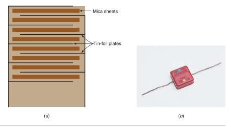
**Figure 16–5** Paper capacitor. (a) Physical construction. (b) Example of a paper capacitor.
