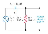
value of  $C_{\rm C}$  for a coupling capacitor having the same reactance. At 100 MHz in the VHF range, the required capacitance is only 1 pF.
