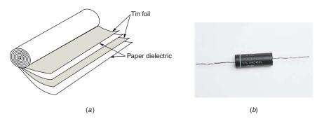
for medium capacitance values of 0.001 to 1.0  $\mu$ F, approximately. The size of a 0.05- $\mu$ F capacitor is typically 1 in. long and  $\frac{3}{8}$ -in. in diameter. A paper capacitor is shown in Fig. 16–5b.
