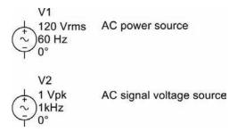
either a power source or a signal voltage source. The amplitude of the power source will be given in RMS voltage ( $V_{RMS}$ ), whereas the amplitude of the signal voltage source will be given in peak voltage ( $V_p$ ).
