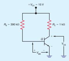
Construct the circuit in Fig. 28–32. Measure and record the following DC values for each of the two transistors:
