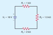
Construct the series circuit in Fig. 4–51. Measure and record the following values.
