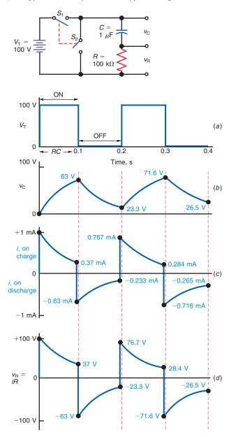
Note that i is an AC waveform around the zero axis, since the charge and discharge currents are in opposite directions. We are arbitrarily taking the charging current as positive values for i.
