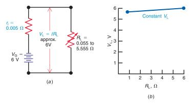
**Figure 12–22** Constant-current generator with high  $r_i$ . The I stays approximately the same 1 mA as  $V_1$  varies with  $R_1$ . (a) Circuit. (b) Graph for I.
