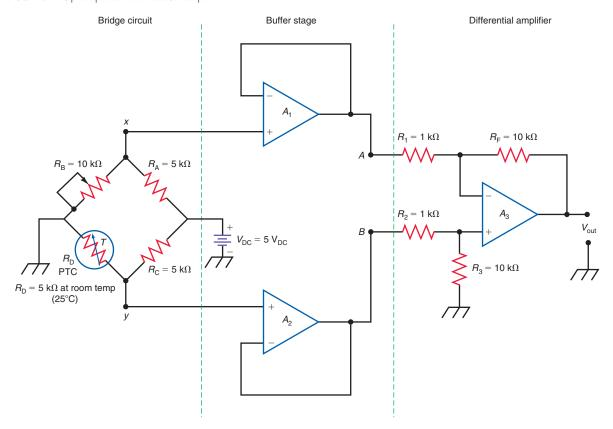
less positive. Since  $V_X$  does not change, the voltage  $V_X - V_Y$  is a positive quantity. Since the gain of the differential amplifier is negative, the output voltage is negative.
