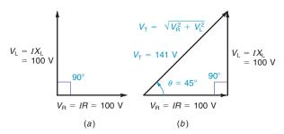
This formula is for  $V_{\rm R}$  and  $V_{\rm L}$  when they are in series, since then they are 90° out of phase. All voltages must be in the same units. When  $V_{\rm T}$  is an rms value,  $V_{\rm R}$  and  $V_{\rm L}$  are also rms values. For the example in Fig. 21–3,
