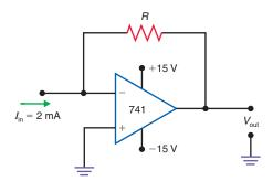
**33–50** In Fig. 33–42, calculate the output voltage,  $V_{\rm out}$ , for the following values of R:
