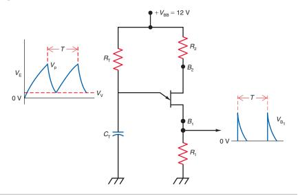
The base 1 voltage waveform,  $V_{\rm B_1}$ , is the most important because it is used to trigger the SCR or triac. The frequency of the base 1 voltage waveform is the same as that of the emitter voltage waveform. The frequency, f, equals 1/T, where T is given by Formula (32–2).
