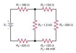
**6–32** In Fig. 6–42, solve for  $R_T$ ,  $I_T$ ,  $V_1$ ,  $V_2$ ,  $V_3$ ,  $V_4$ ,  $V_5$ ,  $V_6$ ,  $I_1$ ,  $I_2$ ,  $I_3$ ,  $I_4$ ,  $I_5$ , and  $I_6$ .
