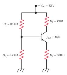
Allowing 0.7 V for  $V_{\rm BE}$ , the emitter voltage,  $V_{\rm E}$  is calculated as
