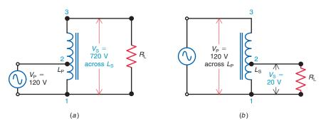
In Fig. 19–13*a*, the autotransformer steps up the generator voltage. Voltage  $V_p$  between 1 and 2 is connected across part of the total turns, and  $V_s$  is induced across all the turns. With six times the turns for the secondary voltage,  $V_s$  also is six times  $V_p$ .
