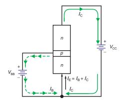
output sides of the circuit. Notice the arrows indicating the direction of the transistor currents  $I_E$ ,  $I_C$ , and  $I_B$ .
