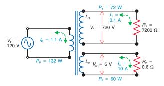
As an aid in these calculations, remember that the side with the higher voltage has the lower current. The primary and secondary *V* and *I* are in the same proportion as the number of turns in the primary and secondary.
