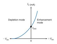
Because D-MOSFETS are normally on devices, the drain current,  $I_{\rm D}$ , can be calculated using Formula (30–2). This formula was given earlier as
