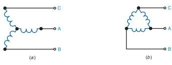
**Figure 15–27** Y connections to a four-wire line with neutral.
