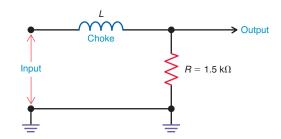
**21–38** If L = 50 mH in Fig. 21–30, then what is the lowest frequency at which L will serve as a choke?
