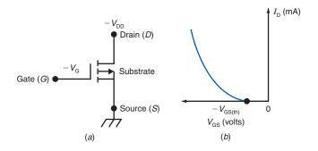
Figure 30–21*b* shows the transconductance curve for the *p*-channel enhancement-type MOSFET. Notice that  $I_D$  is zero until the gate-source voltage is more negative than  $-V_{GS(th)}$ .
