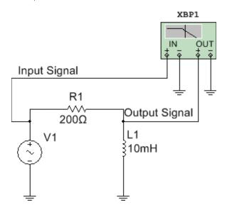
measurement repeated. After operating the circuit at a sufficient number of incremental frequencies, the data would be graphed, with independent variable "frequency" on the x-axis and dependent variable "amplitude" on the y-axis. This process can be very time-consuming. Multisim provides a simpler method of determining the frequency response of a circuit through the use of the virtual Bode plotter.
