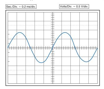
To find the period, T, of the displayed waveform, count the number of horizontal divisions occupied by just one cycle. By viewing the scopes graticule we see that one cycle occupies 5 horizontal divisions. Since the Sec./Div. control is set to 0.2 ms/div., the period, T, is calculated as:
