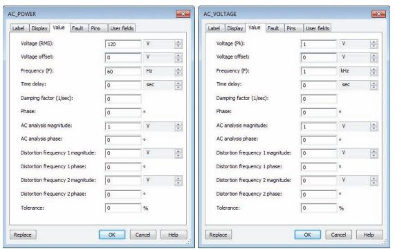
**Figure F–28** Generic function generator and configuration screen.
