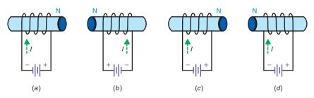
The direction of winding can be over and under, starting from one end of the coil, or under and over with respect to the same starting point. Reversing either the direction of winding or the direction of current reverses the magnetic poles of the solenoid. See Fig. 14–11. When both are reversed, though, the polarity is the same.
