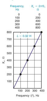
**Figure 20–4** Graph of values to show linear increase of  $X_{\perp}$  for higher values of inductance L. The frequency is constant at 100 Hz.
