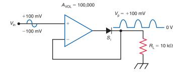
When  $V_{\rm in}$  goes positive, the output of the op amp also goes positive. The diode will turn on when the output of the op amp equals 0.7 V. The amount of input voltage required to obtain 0.7 V at the op-amp output is
