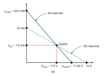
AC load. This implies that there are two load lines: a DC load line and an AC load line. The DC load line shown in Fig. 31-3b has the same endpoints as calculated previously with Fig. 31-2 because the DC quantities do not change with the addition of  $R_{\rm L}$
