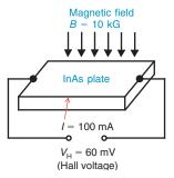
**Figure 13–15** A gaussmeter to measure flux density, with a probe containing an indium arsenide element.
