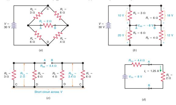
in Fig. 10–6a which would require Kirchhoff's laws for a solution, the Thevenin equivalent in Fig. 10–6b consists of just two voltage dividers. Both the  $R_3$ – $R_4$  divider and the  $R_1$ – $R_2$  divider are across the same 30-V source.
