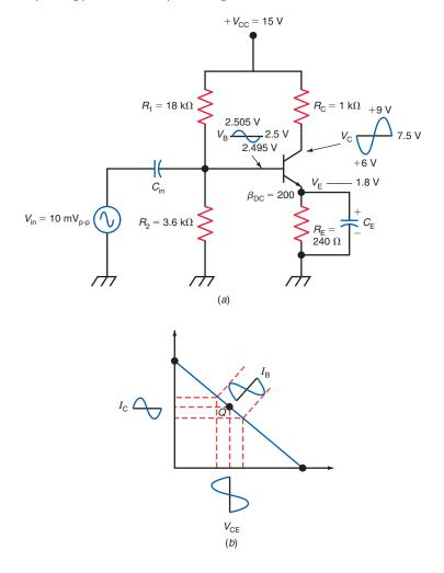
The emitter bypass capacitor holds the emitter constant, as shown in Fig. 29–3*a*. Thus, when the base voltage varies and the emitter voltage is held constant, the change is directly across the base-emitter junction of the transistor.
