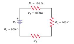
**4-36** In Fig. 4–40, solve for  $R_T$ ,  $V_1$ ,  $V_3$ ,  $V_4$ ,  $R_2$ ,  $R_3$ ,  $P_T$ ,  $P_1$ ,  $P_2$ ,  $P_3$ , and  $P_4$ .
