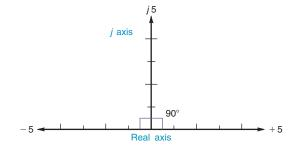
**Figure 24–3** The *j* operator indicates 90° rotation from the real axis; the -j operator is  $-90^{\circ}$ ;  $j^2$  operation is  $180^{\circ}$  rotation back to the real axis in a negative direction.
