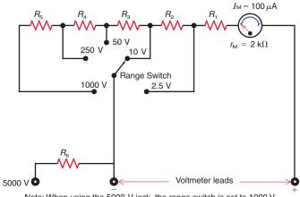
Note: When using the 5000-V jack, the range switch is set to 1000 V.
