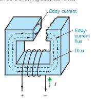
Figure 19–22 Laminated iron core. (a) Shell-type construction. (b) E- and l-shaped laminations. (c) Symbol for iron core.
