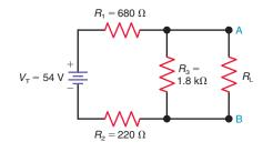
**10–11** In Fig. 10–29, use the Thevenin equivalent circuit to calculate  $I_{\rm L}$  and  $V_{\rm L}$  for the following values of  $R_{\rm L}$ :  $R_{\rm L} = 200~\Omega$ ,  $R_{\rm L} = 1.2~{\rm k}\Omega$ , and  $R_{\rm L} = 1.8~{\rm k}\Omega$ .
