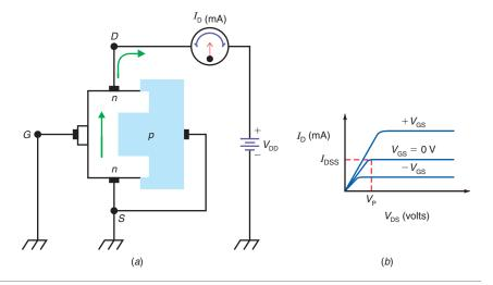
Figure 30-17 (a) Drain current increases with positive gate voltage. (b) Drain current decreases with negative gate voltage.
