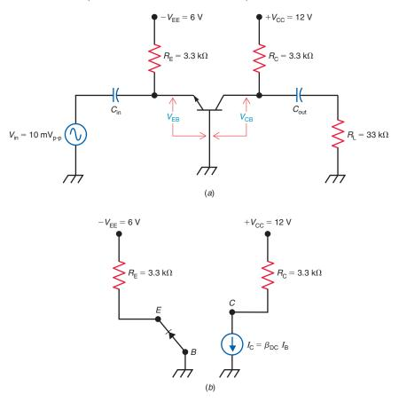
It is important to note that the DC emitter voltage equals  $-0.7\,\mathrm{V}$  with respect to ground.
