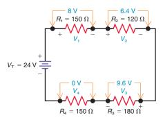
Assume that the series circuit in Fig. 4–22 has failed. A technician troubleshooting the circuit used a voltmeter to record the following resistor voltage drops:
