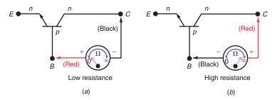
Although not shown, the resistance measured between the collector and emitter should read high or infinite for both connections of the meter leads.
