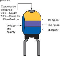
**Figure 16–19** Tantalum capacitor for Example 16–10.
