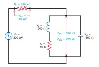
To measure  $Z_{\rm EQ}$ , first tune the LC circuit to resonance. Then adjust  $R_1$  in Fig. 25–9 to the resistance that makes its AC voltage equal to the AC voltage across the tuned circuit. With equal voltages, the  $Z_{\rm EQ}$  must have the same value as  $R_1$ .
