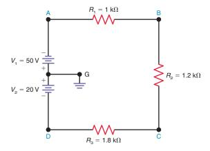
**9–12** In Fig. 9–17, solve for the voltages  $V_{\rm AG}$ ,  $V_{\rm BG}$ , and  $V_{\rm CG}$ . Indicate the proper polarity for each voltage.
