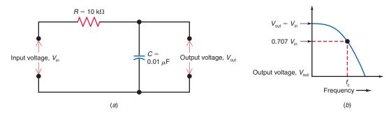
voltage. What follows is a more mathematical approach in analyzing the operation of the most basic low-pass and high-pass filter circuits.
