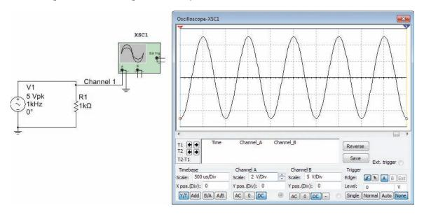
**Figure F-59** Generic oscilloscope icon Ouick Hint.
