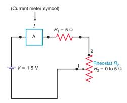
$R_1$  and the voltage source to vary the total resistance  $R_T$  in the circuit. When  $R_T$  changes, the current I changes, as read by the meter.
