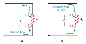
**Figure 4–9** Example of two *IR* voltage drops in series. Electron flow shown for direction of *I*.
