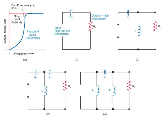
of a high-pass filter with a stop band of 0 to 50 Hz. Above the cutoff frequency of 50 Hz, the higher audio frequencies in the passband can produce af voltage across the output load resistance.
