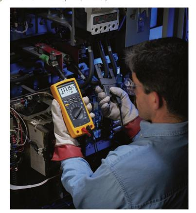
Figure 8–15 DMM with amp-clamp accessory.
