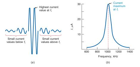
At the resonant frequency,  $X_L$  and  $X_C$  are equal, the net reactance is zero, and the current has its maximum value equal to  $V_T/r_S$ .
