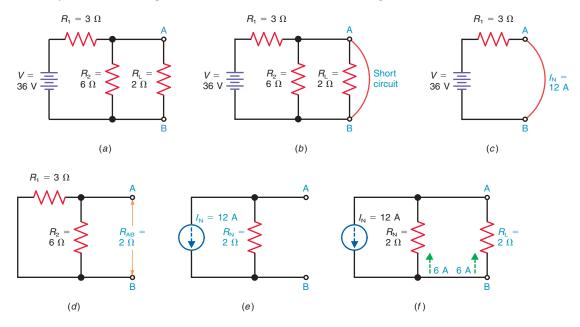
The resultant Norton equivalent is shown in Fig. 10–9e. It consists of a 12-A current source  $I_N$  shunted by the 2- $\Omega$   $R_N$ . The arrow on the current source shows the direction of electron flow from terminal B to terminal A, as in the original circuit.
