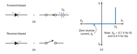
forward voltage,  $V_{\rm F}$ , reaches 0.7 V. Also, the diode is assumed to drop 0.7 V for all currents that pass through it.
