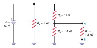
**10–13** In Fig. 10–30, use the Thevenin equivalent circuit to solve for  $I_L$  and  $R_L$ .
