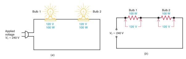
connected to 240 V, the filament would burn out. With the two bulbs in series, however, each has 120 V for proper operation. The two 120-V drops across the bulbs in series add to equal the applied voltage of 240 V.
