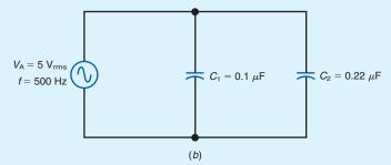
Construct the circuit in Fig. 17–19*b*. Set the frequency of the function generator to exactly 500 Hz. Next, using a DMM, measure and record the following values:
