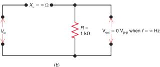
At very low frequencies, where  $X_{\rm L}$  is very small,  $V_{\rm out}$  is approximately equal to  $V_{\rm in}$ . This is true because the ratio  $R/Z_{\rm T}$  approaches one as  $Z_{\rm T}$  and R become approximately the same value. At very high frequencies, the output voltage is approximately zero, because the ratio  $R/Z_{\rm T}$  becomes very small as  $X_{\rm L}$  and thus  $Z_{\rm T}$  approach infinity.
