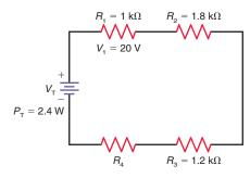
**4-38** In Fig. 4–42, solve for I,  $R_T$ ,  $R_2$ ,  $V_2$ ,  $V_3$ ,  $P_1$ ,  $P_2$ ,  $P_3$ , and  $P_T$ .
