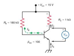
Notice that the calculation for  $V_{\rm CE}$  involves subtracting the voltage drop across  $R_{\rm C}$  from the collector supply voltage,  $V_{\rm CC}$ . Increasing  $I_{\rm C}$  reduces  $V_{\rm CE}$  because of the increased voltage drop across the collector resistor,  $R_{\rm C}$ . Conversely, decreasing  $I_{\rm C}$  increases  $V_{\rm CE}$  due to the reduction of the  $I_{\rm C}R_{\rm C}$  voltage drop.
