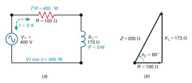
For example, the AC circuit in Fig. 23–13 has 2 A through a 100- $\Omega$  R in series with the  $X_L$  of 173  $\Omega$ . Therefore,
