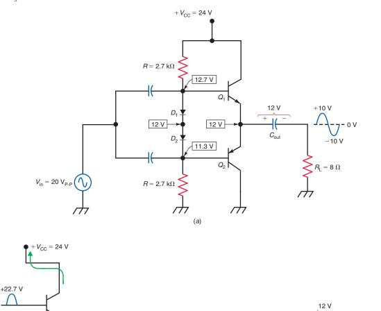
alternation of  $V_{\rm in}$ . The charging current flows through  $R_{\rm L}$  and the collector-emitter region of  $Q_{\rm l}$ .
