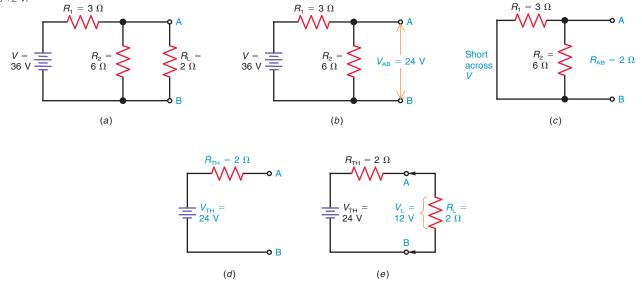
To find  $R_{\rm TH}$ , the 2- $\Omega$   $R_{\rm L}$  is still disconnected. However, now the source V is short-circuited. So the circuit looks like Fig. 10–3c. The 3- $\Omega$   $R_{\rm l}$  is now in parallel with the 6- $\Omega$   $R_{\rm l}$  because both are connected across the same two points. This combined resistance is the product over the sum of  $R_{\rm l}$  and  $R_{\rm l}$ .
