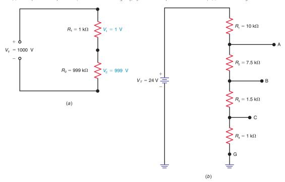
voltage at each tap point is measured with respect to ground. The voltage at tap point C, designated  $V_{\rm CG}$ , is the same as the voltage across  $R_4$ . The calculations for  $V_{\rm CG}$  are as follows:
