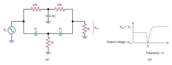
To calculate the notch frequency  $f_N$  in Fig. 26–19a, use Formula (26–11):
