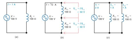
In Fig. 20–6c, each parallel reactance has its individual branch current, equal to the applied voltage divided by the branch reactance. Then each branch current equals  $100 \text{ V}/100 \Omega$ , which is 1 A. The voltage is the same across both reactances, equal to the generator voltage, since they are all in parallel.
