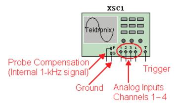
Figure F-72 Tektronix oscilloscope Quick Hint.
