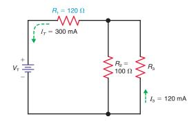
**6–29** In Fig. 6–39, solve for  $R_T$ ,  $I_T$ ,  $V_T$ ,  $V_T$ ,  $V_2$ ,  $V_4$ ,  $I_2$ , and  $I_3$ .
