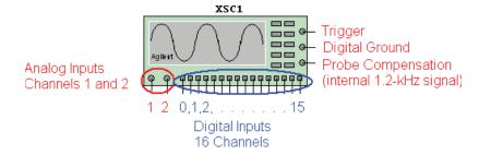
Figure F-65 Agilent oscilloscope Quick Hint.
