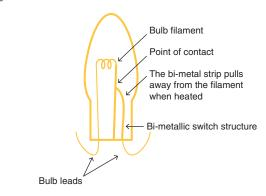
than two dissimilar strips of metal that bend when heated. When the heat produced by the bulb's filament reaches some predetermined level, the bi-metallic thermal switch opens. When the bulb cools off, it closes again. Since the flasher unit is in series with all of the bulbs in the entire series string, all of the lights blink on and off rapidly. Because strings of holiday lights are often used outdoors, the outside temperature may affect how fast the lights blink on and off.
