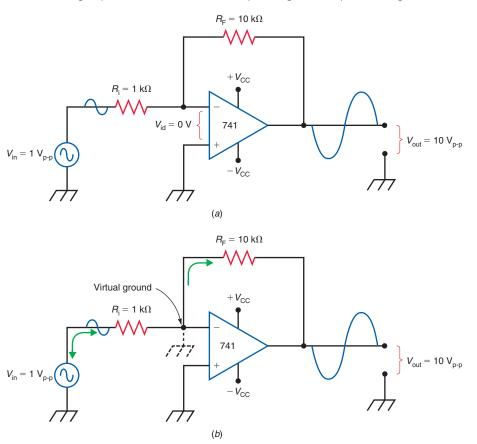
For all practical purposes,  $V_{\rm id}$  is so small that it can be considered zero in most cases. This introduces little or no error in circuit analysis. Since  $V_{\rm id}$  is so small (practically zero), the inverting input terminal of the op amp is said to be at virtual ground. This means that the voltage at the op amp's inverting input is at the same potential as ground, yet it can sink no current. This point of virtual ground is illustrated in Fig. 33–11b.
