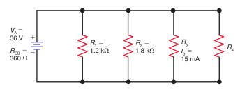
**5–58** In Fig. 5–36, solve for  $V_A$ ,  $I_1$ ,  $I_2$ ,  $R_2$ ,  $R_3$ ,  $I_4$ , and  $R_{EO}$ .
