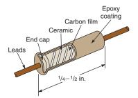
**Figure 2-5** Construction of metal-film resistor.
