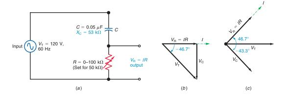
This circuit provides a phase-shifted voltage  $V_R$  at the output with respect to the input. For this reason, the phasors are redrawn in Fig. 18–5c to show the voltages with the input  $V_T$  as the horizontal reference. The conclusion, then, is that the output voltage across R leads the input  $V_T$  by 46.7°, whereas  $V_C$  lags  $V_T$  by 43.3°.
