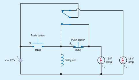
In this part of the lab we will experimentally determine the pickup current and the holding current for your relay. Recall that the pickup current is defined as the minimum amount of relay coil current required to energize or operate a relay. The holding current is defined as the minimum amount of current required to keep a relay energized or operating.
