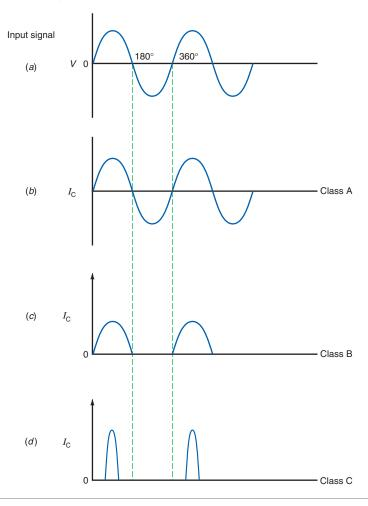
that is approximately one-half its maximum value at saturation. Then the AC output signal can swing above and below this value without the transistor immediately reaching either cutoff or saturation. The characteristics of a class A amplifier include both low distortion and low power efficiency.
