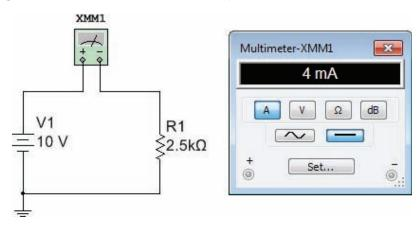
Figure F-55 Generic multimeter Quick Hint.
