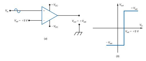
**Figure 33–26** Schmitt trigger. (a) Circuit. (b) Transfer characteristic.
