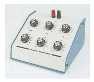
trying different *R* values in a circuit. Inside the box are six series strings of resistors, with one string for each dial switch.
