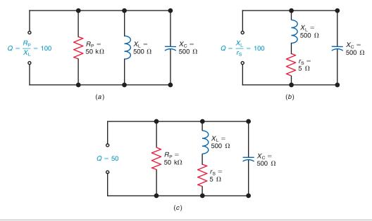
increasing the series resistance  $r_{\rm S}$  because the resonant response is more symmetrical with shunt damping.
