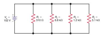
**5–10** Recalculate the values for  $I_1$ ,  $I_2$ ,  $I_3$ , and  $I_4$  in Fig. 5–23 if the applied voltage,  $V_A$ , is reduced to 51V.
