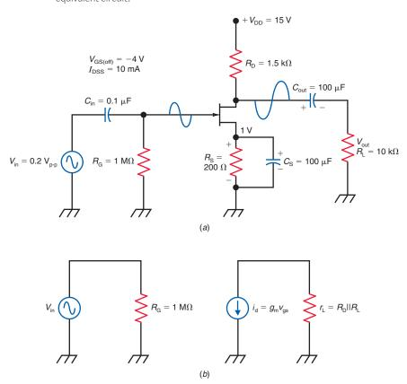
The AC equivalent circuit is shown in Fig. 30–12b. Notice that on the input side,  $R_{\rm G}=Z_{\rm in}$ , which is 1 M $\Omega$ . Again, this occurs because with practically zero gate current, the gate-source resistance, designated  $R_{\rm GS}$ , approaches infinity.
