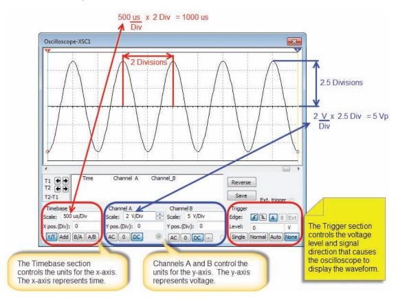
Figure F-61 Generic oscilloscope Quick Hint.
