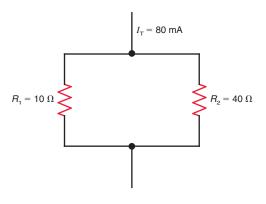
**7-16** Multi*Sim* In Fig. 7–21, solve for  $I_1$  and  $I_2$ .
