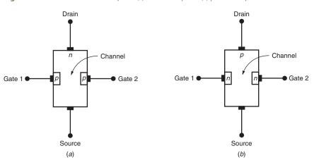
Figure 30–1 Construction of a JFET. (a) n-channel JFET. (b) p-channel JFET.
