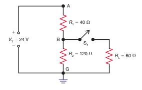
**7-25** In Fig. 7–29, explain why the voltage,  $V_{\rm BG}$ , decreases when the switch,  $S_1$  is closed.
