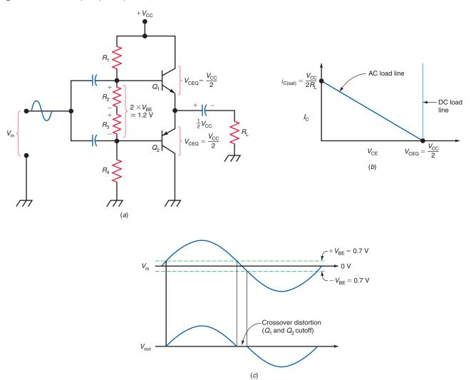
conducts and  $Q_2$  is cut off. Conversely, when  $V_{\rm in}$  is negative,  $Q_2$  conducts and  $Q_1$  is cut off. Careful examination of the circuit reveals that each transistor acts like an emitter follower for one half-cycle of the input voltage.
