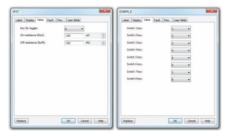
an individual switch within a switch pack, a white rectangle appears around the switch and the cursor changes into a pointing hand symbol. When the white rectangle is present and the cursor resembles a pointing hand, a single left mouse click will cause the switch to change positions. The black dot on the switch pack signifies the ON position.
