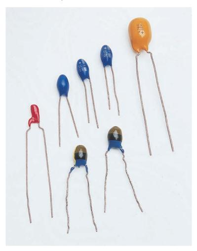
A nonpolarized electrolytic actually contains two capacitors, connected internally in series-opposing polarity.
