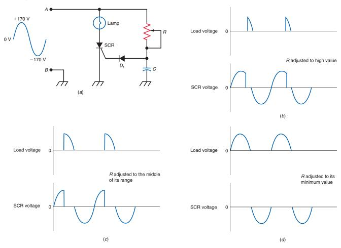
always  $90^{\circ}$  out of phase. In Fig. 32–6a, the voltage across the capacitor is applied to the anode side of the diode,  $D_1$ . The cathode lead of the diode connects to the gate of the SCR. Again, the purpose of using the diode is to ensure that the negative alternation of the input voltage cannot apply excessive reverse-bias voltage to the SCR's gate-cathode junction.
