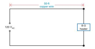
**11–2** In Fig. 11–22, recalculate the values in steps a through i in Prob. 11–1 if the 8- $\Omega$  heater is replaced with a 24- $\Omega$  fan.
