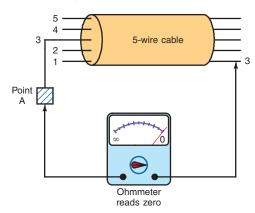
conductor can have an internal break which is not visible because of the insulated cover, or the wire can have a bad connection at the terminal. Checking for zero ohms between any two points along the conductor tests continuity. A break in the conducting path is evident from a reading of infinite resistance, showing an open circuit.
