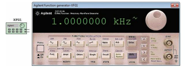
The Agilent function generator is controlled via the front panel, as shown in Fig. F–29. The buttons are "pushed" by a left mouse click. The dial can be turned by dragging the mouse over it or by placing the cursor over it and spinning the wheel on the mouse. The latter is by far the preferred method.
