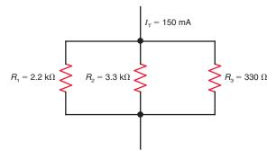
**7-21** In Fig. 7–26, solve for  $I_1$ ,  $I_2$ , and  $I_3$ .
