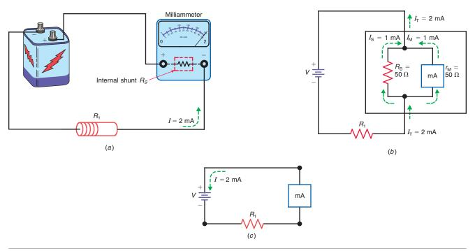
**Figure 8–5** Calculating the resistance of a meter shunt.  $R_s$  is equal to  $V_M/I_s$ . See text for calculations.
