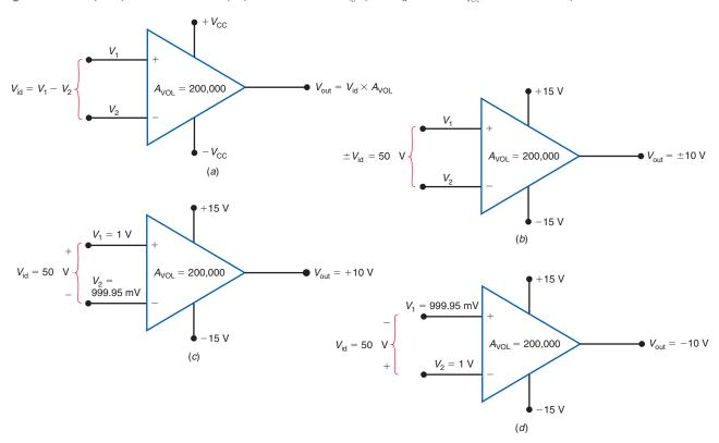
Assume in Fig. 33–6c that  $V_1 = 1$  V and  $V_2 = 999.95$  mV. What will the output be? Simply multiply  $V_{id}$  by  $A_{VOL}$ . First, find  $V_{id}$ :
