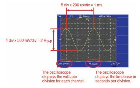
$$V_{\text{p-p}} = 4 \text{ divisions} \times \frac{500 \text{ mV}}{\text{division}}$$
