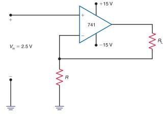
**33–48** In Fig. 33–41, calculate the output current,  $I_{\rm out}$ , for the following values of R:
