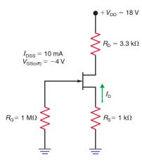
**30–16** In Fig. 30–27, what value of  $R_s$  will provide a drain current,  $I_D$ , of approximately one-half  $I_{DSS}$ ?
