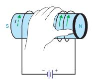
**Figure 14–11** Examples for determining the magnetic polarity of a coil with direct current *I*. The *I* is electron flow. The polarities are reversed in (*a*) and (*b*) because the battery is reversed to reverse the direction of current. Also, (*d*) is the opposite of (*c*) because of the reversed winding.
