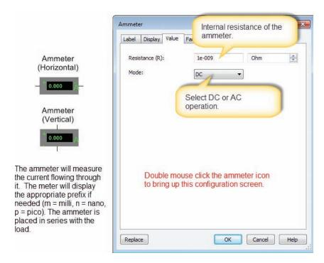
**Figure F–54** DC current measurement with a generic multimeter.
