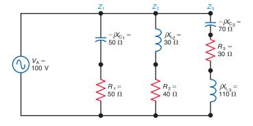
These steps are used in the following calculations to solve the circuit in Fig. 24–14. All the values are in A, V, or  $\Omega$  units.
