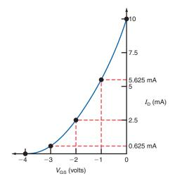
Notice how the transconductance,  $g_{\rm m}$ , increases with the height of the transconductance curve.
