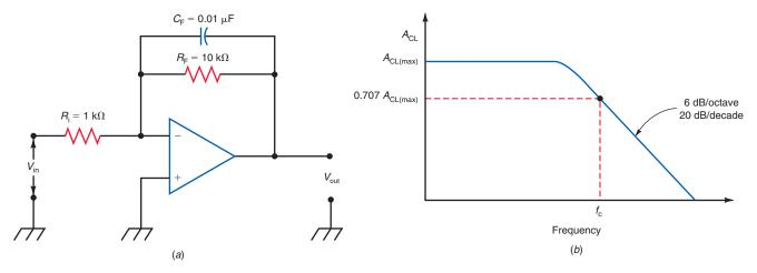
feedback. At extremely high frequencies,  $X_{\rm C}$  equals almost zero ohms and the voltage gain approaches zero.
