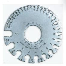
In typical applications, hookup wire for electronic circuits with current of the order of milliamperes is generally about No. 22 gage. For this size, 0.5 to 1 A is the maximum current the wire can carry without excessive heating.
