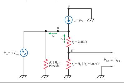
The AC load in the emitter circuit equals  $R_{\rm E}$  and  $R_{\rm L}$  in parallel. Its value is calculated as
