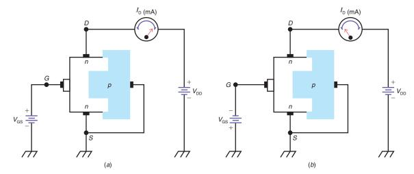
to the source. With the gate shorted to the source, drain current,  $I_{\rm D}$ , will flow in the n-type channel. Because the p-type substrate is grounded, the n-channel and p-type substrate are always reverse-biased; this results in zero current in the substrate. Also, note that zero gate current flows because of the extremely high resistance of the  ${\rm SiO}_2$  insulating layer. The resistance between the gate and channel is of the order of several thousands of megohms.
