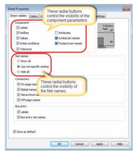
The initial configuration of Multisim will display the Net names within the circuit. The Net names are the numbers circled in red in Fig. F–77.
