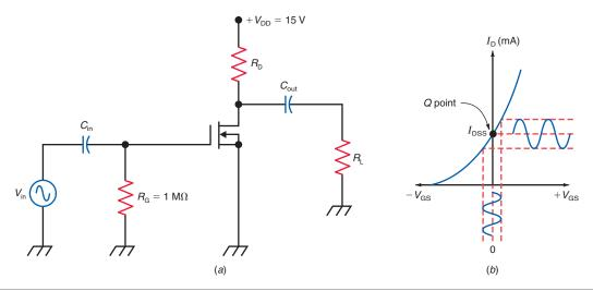
To calculate the DC voltage at the drain, use Formula (30–20):
