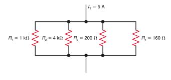
**7-23** In Fig. 7–28, solve for  $I_1$ ,  $I_2$ ,  $I_3$ , and  $I_4$ .
