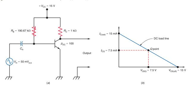
Note that when the transistor is cut off ( $I_{\rm C}=0$  mA), the collector-emitter region appears open and the voltage  $V_{\rm CE}=V_{\rm CC}$ , which is 15 V in this case. Conversely, when the transistor is saturated, the collector-emitter region appears shorted ( $V_{\rm CE}=0$  V) and only the values of  $V_{\rm CC}$  and  $R_{\rm C}$  limit  $I_{\rm C}$ .
