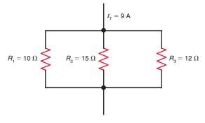
**7-20** In Fig. 7–25, solve for  $I_1$ ,  $I_2$ , and  $I_3$ .
