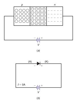
Any increase in the temperature of the diode increases the leakage current in the diode. These minority current carriers move in a direction that is opposite to the direction provided with forward bias.
