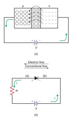
analyzing diode circuits. In this book, however, we will use electron flow when analyzing circuits containing diodes.
