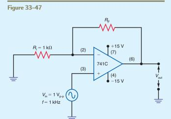
With channel 1 of the oscilloscope connected to the input voltage,  $V_{\rm in}$ , and channel 2 connected to the output of the op amp, measure and record the phase relationship between  $V_{\rm in}$  and  $V_{\rm out}$ .  $\theta =$  \_\_\_\_\_
