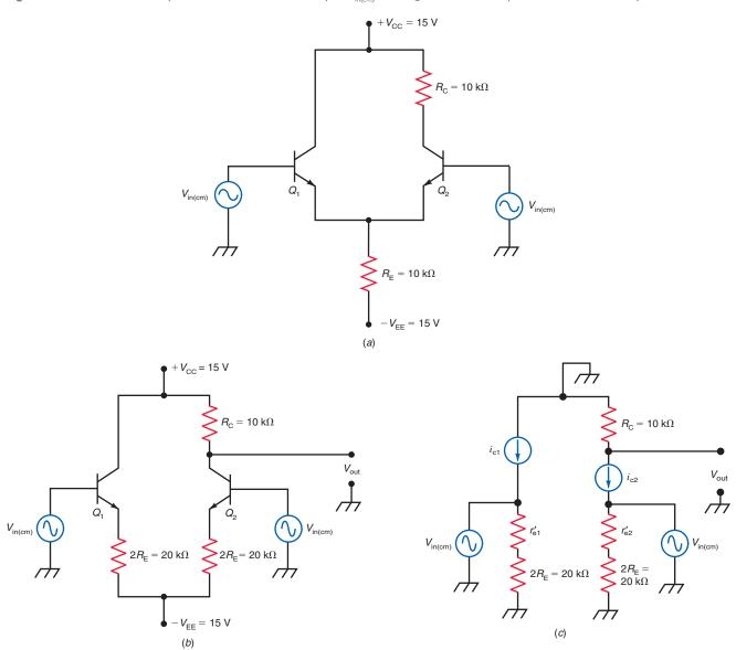
The AC equivalent circuit is shown in Fig. 33–4c. The output voltage equals
