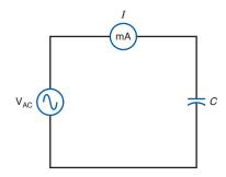
**17–5** In Fig. 17–11, list three factors that can affect the amount of charge and discharge current flowing in the circuit.
