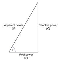
It should be noted that the reactive power,  $Q_1$ , in an inductor is at an angle of  $\pm 90^{\circ}$ , whereas the reactive power,  $Q_{c}$ , in a capacitor is at an angle of  $-90^{\circ}$ .
