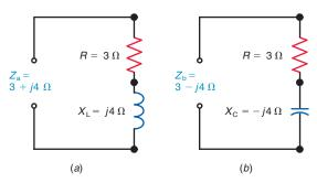
**Figure 24–6** Rectangular form of complex numbers for branch currents. (a) Current  $I_{\rm L}$  is -j. (b) Current  $I_{\rm C}$  is +j.
