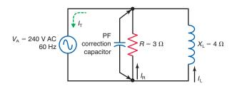
power factor decreases, the apparent power, total current, and overall power losses in the system increase. To say it another way, the ratio of delivered power to generated power decreases as the power factor decreases.
