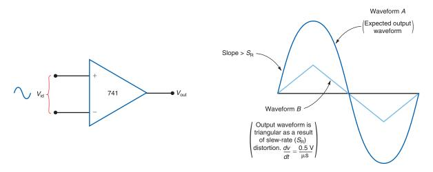
**Figure 33–10** Waveforms *A* and *B* have the same frequency but different slopes during positive and negative alternations.
