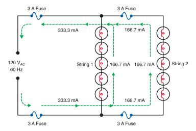
**Figure 5-19***c* Three sets of holiday lights connected together.
