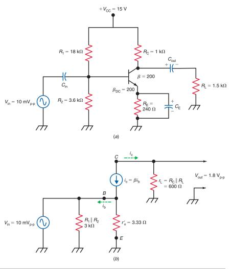
and  $R_L$  appear in parallel (see the AC equivalent circuit in Fig. 29–6b). The voltage gain,  $A_V$ , now is
