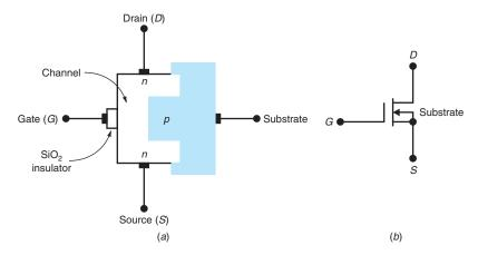
is at the top of the n-material and the source terminal is at the bottom. The block of p-type material forms the substrate into which the n-type material is embedded. The n-type material forms the channel. Along the n-channel, a thin layer of silicon dioxide (SiO $_2$ ) is deposited to isolate the gate from the channel. From gate to channel are the metal, silicon dioxide, and n-type semiconductor materials, in that order, which give the MOSFET its name.
