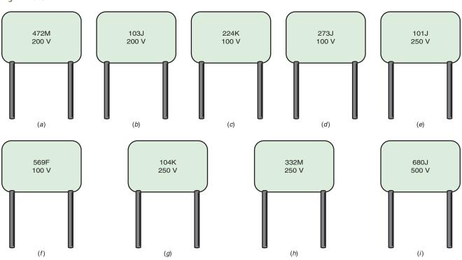
**16–9** Determine the capacitance and tolerance of each of the capacitors shown in Fig. 16–32.
