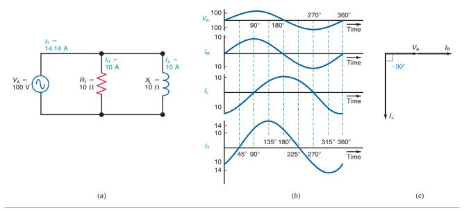
**Figure 21–6** Phasor triangle of inductive and resistive branch currents  $90^{\circ}$  out of phase in a parallel circuit to find resultant  $I_{\rm T}$ .
