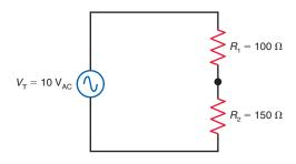
**15–38** In Fig. 15–34, solve for the following values:  $I_1$ ,  $I_2$ ,  $I_7$ ,  $R_{\rm EQ}$ ,  $P_1$ ,  $P_2$ , and  $P_7$ .
