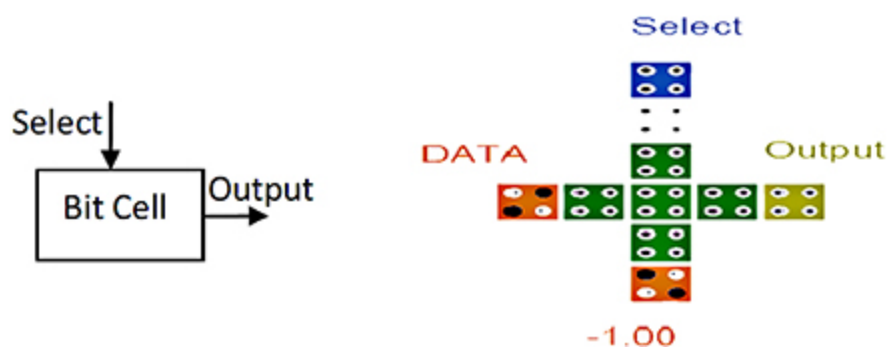
Figure 28.4. The block diagram of a ROM bit cell and its corresponding QCA structure. Reproduced with permission from [11]. Copyright 2008 IEEE.
