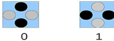
Figure 20.9. The symmetric adjustable QCA cell.
