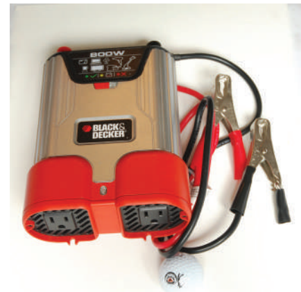
FIG. 13.72 12 V dc to 120 V ac inverter. (Don Johnson Photo)
