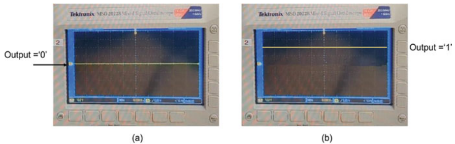
Fig. 13.18 Observation of level shift in the oscilloscope. (a) When output is zero, (b) when the output is one
