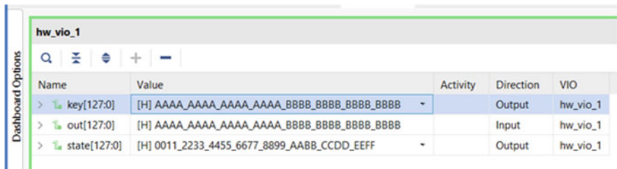
Fig. 5.14 Key leaked to the output when the Trojan is activated
