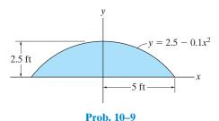
**10–10.** Determine the moment of inertia of the area about the x axis.
