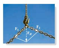
The parallelogram law must be used to determine the resultant of the two forces acting on the hook. (© Russell C. Hibbeler)
