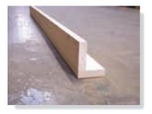
The effectiveness of this beam to resist bending can be determined once its moments of inertia and its product of inertia are known. (© Russell C. Hibbeler)
