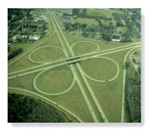
Motorists traveling along this cloverleaf interchange experience a normal acceleration due to the change in direction of their velocity. A tangential component of acceleration occurs when the cars' speed is increased or decreased. (© R.C. Hibbeler)
