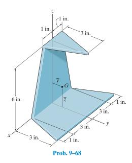
**9–69.** A triangular plate made of homogeneous material has a constant thickness that is very small. If it is folded over as shown, determine the location  $\bar{z}$  of the plate's center of gravity G.
