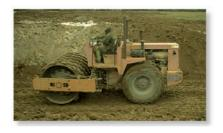
The total kinetic energy of this soil compactor consists of the kinetic energy of the body or frame of the machine due to its translation, and the translational and rotational kinetic energies of the roller and the wheels due to their general plane motion. Here we exclude the additional kinetic energy developed by the moving parts of the engine and drive train. (© R.C. Hibbeler)
