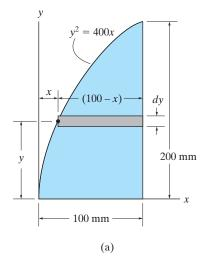
Determine the moment of inertia for the shaded area shown in Fig. 10–6a about the x axis.
