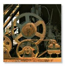
The gears used in the operation of a crane all rotate about fixed axes. Engineers must be able to relate their angular motions in order to properly design this gear system. (© R.C. Hibbeler)
