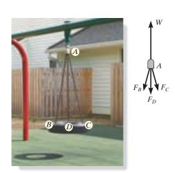
The joint at A is subjected to the force from the support as well as forces from each of the three chains. If the tire and any load on it have a weight W, then the force at the support will be W, and the three scalar equations of equilibrium can be applied to the free-body diagram of the joint in order to determine the chain forces,  $F_B$ ,  $F_C$ , and  $F_D$ . (© Russell C. Hibbeler)
