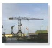
Simple trusses are often used in the construction of large cranes in order to reduce the weight of the boom and tower. (© Russell C. Hibbeler)
