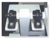
The journal bearings support the ends of the shaft. (5) (© Russell C. Hibbeler)
