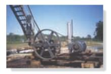
Flat or V-belts are often used to transmit the torque developed by a motor to a wheel attached to a pump, fan, or blower. (© Russell C. Hibbeler)
