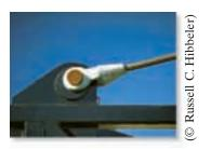
The cable exerts a force on the bracket in the direction of the cable. (1)
