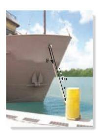
The force **F** acting along the rope can be represented as a Cartesian vector by establishing x, y, z axes and first forming a position vector **r** along the length of the rope. Then the corresponding unit vector  $\mathbf{u} = \mathbf{r}/r$  that defines the direction of both the rope and the force can be determined. Finally, the magnitude of the force is combined with its direction,  $\mathbf{F} = F\mathbf{u}$ . (© Russell C. Hibbeler)
