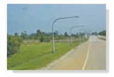
Integration must be used to determine the location of the center of gravity of this lamp post due to the curvature of the member. (© Russell C. Hibbeler) **Centroid of an Area.** If an area lies in the x-y plane and is bounded by the curve y = f(x), as shown in Fig. 9–5a, then its centroid will be in this plane and can be determined from integrals similar to Eqs. 9–3, namely,
