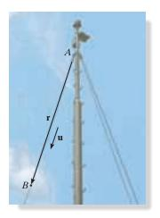
If an x, y, z coordinate system is established, then the coordinates of two points A and B on the cable can be determined. From this the position vector  $\mathbf{r}$  acting along the cable can be formulated. Its magnitude represents the distance from A to B, and its unit vector,  $\mathbf{u} = \mathbf{r}/r$ , gives the direction defined by  $\alpha$ ,  $\beta$ ,  $\gamma$ . (© Russell C. Hibbeler)
