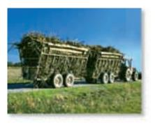
During high winds and when going around a curve, these sugar-cane trucks can become unstable and tip over since their center of gravity is high off the road when they are fully loaded. (© Russell C. Hibbeler)
