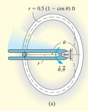
Due to the rotation of the forked rod, the ball in Fig. 12–35*a* travels around the slotted path, a portion of which is in the shape of a cardioid,  $r = 0.5(1 - \cos \theta)$  ft, where  $\theta$  is in radians. If the ball's velocity is v = 4 ft/s and its acceleration is a = 30 ft/s<sup>2</sup> at the instant  $\theta = 180^{\circ}$ , determine the angular velocity  $\dot{\theta}$  and angular acceleration  $\ddot{\theta}$  of the fork.
