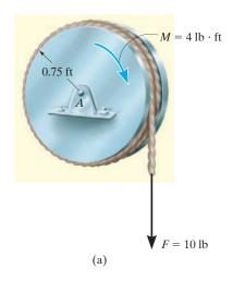
The 20-lb disk shown in Fig. 19–5a is acted upon by a constant couple moment of 4 lb·ft and a force of 10 lb which is applied to a cord wrapped around its periphery. Determine the angular velocity of the disk two seconds after starting from rest. Also, what are the force components of reaction at the pin?
