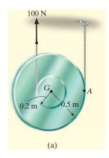
Determine the angular acceleration of the spool in Fig. 17–20a. The spool has a mass of 8 kg and a radius of gyration of  $k_G = 0.35$  m. The cords of negligible mass are wrapped around its inner hub and outer rim.
