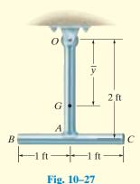
The pendulum in Fig. 10–27 consists of two thin rods each having a weight of 10 lb. Determine the pendulum's mass moment of inertia about an axis passing through (a) the pin at O, and (b) the mass center G of the pendulum.
