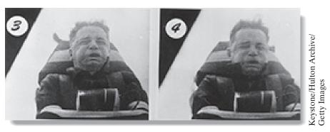
Upon deceleration the force of the seatbelt  $\mathbf{F}'$  tends to pull his body to a stop, but his head leaves contact with the back of the seat and his face distorts forward, again due to his inertia or tendency to continue to move forward. No force is pulling him forward, although this is the sensation he receives.
