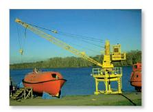
The boom can rotate up and down, and because it is hinged at a point on the vertical axis about which it turns, it is subjected to rotation about a fixed point. (© R.C. Hibbeler)
