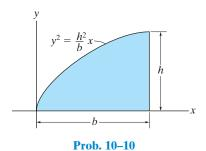
**10–11.** Determine the moment of inertia for the shaded area about the x axis.
