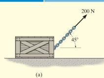
The 100-kg crate shown in Fig. 15–5a is originally at rest on the smooth horizontal surface. If a towing force of 200 N, acting at an angle of 45°, is applied for 10 s, determine the final velocity and the normal force which the surface exerts on the crate during this time interval.
