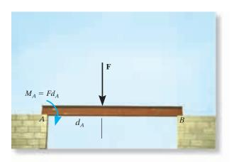
As illustrated by the example problems, the moment of a force does not always cause a rotation. For example, the force  $\mathbf{F}$  tends to rotate the beam clockwise about its support at A with a moment  $M_A = Fd_A$ . The actual rotation would occur if the support at B were removed. (© Russell C. Hibbeler)
