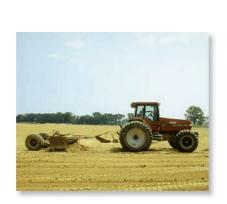
The scraper box behind this tractor represents a device that gains mass. If the tractor maintains a constant velocity v, then dv/dt=0 and, because the soil is originally at rest,  $v_{D/i}=v$ . Applying Eq. 15–29, the horizontal towing force on the scraper box is then T=0+v(dm/dt), where dm/dt is the rate of soil accumulated in the box. (© R.C. Hibbeler)
