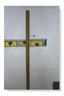
Regardless of the weight of the rake or shovel that is suspended, the device has been designed so that the small roller holds the handle in equilibrium due to frictional forces that develop at the points of contact, A, B, C. (© Russell C. Hibbeler)
