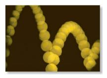
The quality of a manufactured tennis ball is measured by the height of its bounce, which can be related to its coefficient of restitution. Using the mechanics of oblique impact, engineers can design a separation device to remove substandard tennis balls from a production line. (© Gary S. Settles/Science Source)
