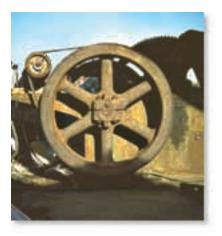
This flywheel, which operates a metal cutter, has a large moment of inertia about its center. Once it begins rotating it is difficult to stop it and therefore a uniform motion can be effectively transferred to the cutting blade. (© Russell C. Hibbeler)
