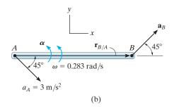
The rod AB shown in Fig. 16–27a is confined to move along the inclined planes at A and B. If point A has an acceleration of 3 m/s<sup>2</sup> and a velocity of 2 m/s, both directed down the plane at the instant the rod is horizontal, determine the angular acceleration of the rod at this instant.
