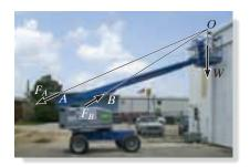
The boom and bucket on this lift is a three-force member, provided its weight is neglected. Here the lines of action of the weight of the worker,  $\mathbf{W}$ , and the force of the two-force member (hydraulic cylinder) at B,  $\mathbf{F}_B$ , intersect at O. For moment equilibrium, the resultant force at the pin A,  $\mathbf{F}_A$ , must also be directed towards O. (© Russell C. Hibbeler)
