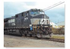
The power output of this locomotive comes from the driving frictional force developed at its wheels. It is this force that overcomes the frictional resistance of the cars in tow and is able to lift the weight of the train up the grade. (© R.C. Hibbeler)
