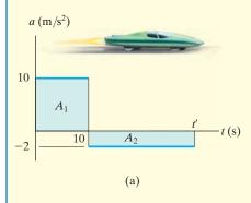
The car in Fig. 12–14*a* starts from rest and travels along a straight track such that it accelerates at  $10 \text{ m/s}^2$  for 10 s, and then decelerates at  $2 \text{ m/s}^2$ . Draw the v-t and s-t graphs and determine the time t' needed to stop the car. How far has the car traveled?
