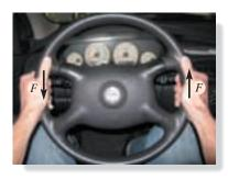
Steering wheels on vehicles have been made smaller than on older vehicles because power steering does not require the driver to apply a large couple moment to the rim of the wheel. (© Russell C. Hibbeler)
