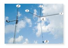
Complicated spatial motion of the concrete bucket B occurs due to the rotation of the boom about the Z axis, motion of the carriage A along the boom, and extension and swinging of the cable AB. A translating-rotating x, y, z coordinate system can be established on the carriage, and a relative-motion analysis can then be applied to study this motion. (© R.C. Hibbeler)
