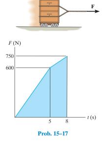
**15–18.** The motor exerts a force F on the 40-kg crate as shown in the graph. Determine the speed of the crate when t = 3 s and when t = 6 s. When t = 0, the crate is moving downward at 10 m/s.
