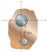
**F15–18.** Two disks A and B each have a mass of 1 kg and the initial velocities shown just before they collide. If the coefficient of restitution is e = 0.5, determine their speeds just after impact.
