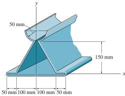
**9–55.** Locate the center of gravity  $(\bar{x}, \bar{y}, \bar{z})$  of the homogeneous wire.
