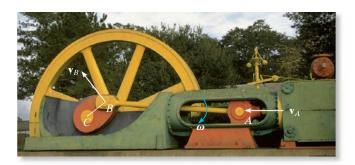
As slider block A moves horizontally to the left with a velocity  $\mathbf{v}_A$ , it causes crank CB to rotate counterclockwise, such that  $\mathbf{v}_B$  is directed tangent to its circular path, i.e., upward to the left. The connecting rod AB is subjected to general plane motion, and at the instant shown it has an angular velocity  $\boldsymbol{\omega}$ . (© R.C. Hibbeler)
