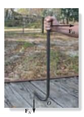
The ability to remove the nail will require the moment of  $\mathbf{F}_H$  about point O to be larger than the moment of the force  $\mathbf{F}_N$  about O that is needed to pull the nail out. (© Russell C. Hibbeler)
