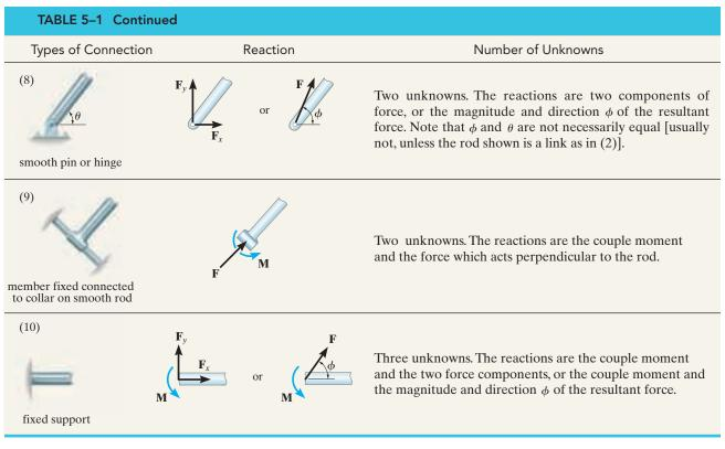
Typical examples of actual supports are shown in the following sequence of photos. The numbers refer to the connection types in Table 5–1.
