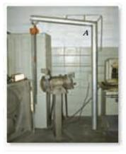
The designer of this shop crane realized the need for additional reinforcement around the joint at *A* in order to prevent severe internal bending of the joint when a large load is suspended from the chain hoist. (© Russell C. Hibbeler)
