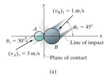
Two smooth disks A and B, having a mass of 1 kg and 2 kg, respectively, collide with the velocities shown in Fig. 15–18a. If the coefficient of restitution for the disks is e = 0.75, determine the x and y components of the final velocity of each disk just after collision.
