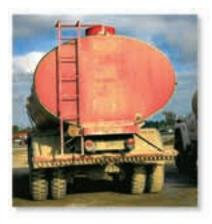
The resultant force of the water pressure and its location on the elliptical back plate of this tank truck must be determined by integration. (© Russell C. Hibbeler)
