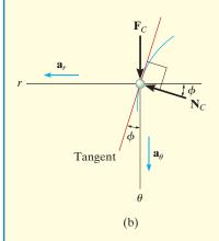
A can C, having a mass of 0.5 kg, moves along a grooved horizontal slot shown in Fig. 13–21a. The slot is in the form of a spiral, which is defined by the equation  $r=(0.1\theta)$  m, where  $\theta$  is in radians. If the arm OA rotates with a constant rate  $\dot{\theta}=4\,\mathrm{rad/s}$  in the horizontal plane, determine the force it exerts on the can at the instant  $\theta=\pi\,\mathrm{rad}$ . Neglect friction and the size of the can.
