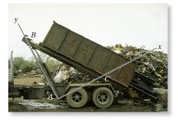
The rotation of the dumping bin of the truck about point C is operated by the extension of the hydraulic cylinder AB. To determine the rotation of the bin due to this extension, we can use the equations of relative motion and fix the x, y axes to the cylinder so that the relative motion of the cylinder's extension occurs along the y axis. (© R.C. Hibbeler)
