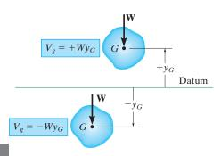
**Gravitational Potential Energy.** Since the total weight of a body can be considered concentrated at its center of gravity, the *gravitational potential energy* of the body is determined by knowing the height of the body's center of gravity above or below a horizontal datum.
