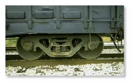
The suspension of a railroad car consists of a set of springs which are mounted between the frame of the car and the wheel truck. This will give the car a natural frequency of vibration which can be determined. (© R.C. Hibbeler)
