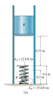
The ram R shown in Fig. 14–22a has a mass of 100 kg and is released from rest 0.75 m from the top of a spring, A, that has a stiffness  $k_A = 12 \text{ kN/m}$ . If a second spring B, having a stiffness  $k_B = 15 \text{ kN/m}$ , is "nested" in A, determine the maximum displacement of A needed to stop the downward motion of the ram. The unstretched length of each spring is indicated in the figure. Neglect the mass of the springs.
