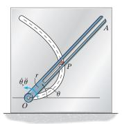
**F12–36.** Peg *P* is driven by the forked link *OA* along the path described by  $r = e^{\theta}$ , where r is in meters. When  $\theta = \frac{\pi}{4}$  rad, the link has an angular velocity and angular acceleration of  $\dot{\theta} = 2 \text{ rad/s}$  and  $\ddot{\theta} = 4 \text{ rad/s}^2$ . Determine the radial and transverse components of the peg's acceleration at this instant.
