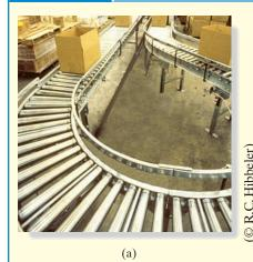
The boxes in Fig. 12–29*a* travel along the industrial conveyor. If a box as in Fig. 12–29*b* starts from rest at *A* and increases its speed such that  $a_t = (0.2t) \text{ m/s}^2$ , where *t* is in seconds, determine the magnitude of its acceleration when it arrives at point *B*.
