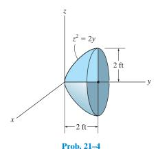
**21–5.** Determine by direct integration the product of inertia  $I_{yz}$  for the homogeneous prism. The density of the material is  $\rho$ . Express the result in terms of the total mass m of the prism.
