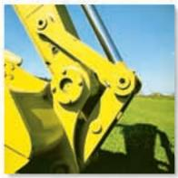
In each case, the link on the backhoe is a two-force member. In the top photo it is subjected to both bending and an axial load at its center. It is more efficient to make the member straight, as in the bottom photo; then only an axial force acts within the member. (© Russell C. Hibbeler)
