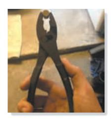
Common tools such as these pliers act as simple machines. Here the applied force on the handles creates a much larger force at the jaws. (© Russell C. Hibbeler)
