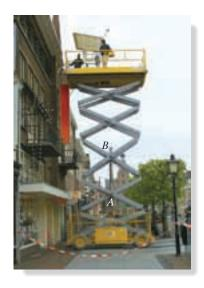
This scissors lift has one degree of freedom. Without the need for dismembering the mechanism, the force in the hydraulic cylinder *AB* required to provide the lift can be determined *directly* by using the principle of virtual work. (© Russell C. Hibbeler)
