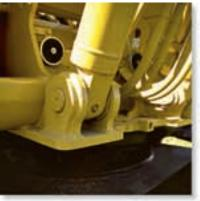
This thrust bearing is used to support the This pin is used to support the end of the strut used on a tractor. (8) (© Russell C. Hibbeler)
