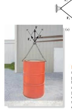
Using the parallelogram law the supporting force  $\mathbf{F}$  can be resolved into components acting along the u and v axes. (© Russell C. Hibbeler)
