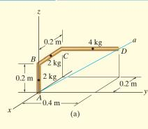
Determine the moment of inertia of the bent rod shown in Fig. 21-5a about the Aa axis. The mass of each of the three segments is given in the figure.
