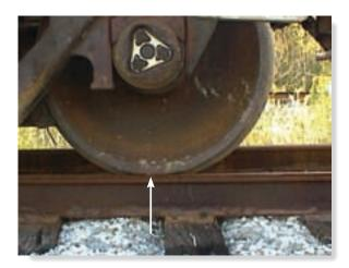
Steel is a common engineering material that does not deform very much under load. Therefore, we can consider this railroad wheel to be a rigid body acted upon by the concentrated force of the rail. (© Russell C. Hibbeler)
