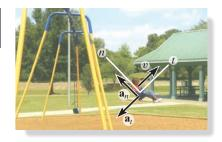
As the boy swings upward with a velocity  $\mathbf{v}$ , his motion can be analyzed using n-t coordinates. As he rises, the magnitude of his velocity (speed) is decreasing, and so  $a_t$  will be negative. The rate at which the direction of his velocity changes is  $a_n$ , which is always positive, that is, towards the center of rotation. (© R.C. Hibbeler)
