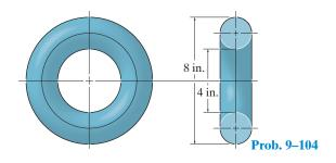
**9–105.** The heat exchanger radiates thermal energy at the rate of 2500 kJ/h for each square meter of its surface area. Determine how many joules (J) are radiated within a 5-hour period.
