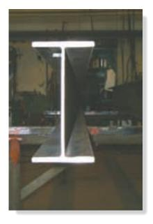
In order to predict the strength and deflection of this beam, it is necessary to calculate the moment of inertia of the beam's cross-sectional area. (© Russell C. Hibbeler)
