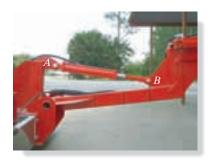
The hydraulic cylinder AB is a typical example of a two-force member since it is pin connected at its ends and, provided its weight is neglected, only the pin forces act on this member. (© Russell C. Hibbeler)
