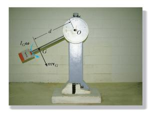
As the pendulum swings downward, its angular momentum about point O can be determined by computing the moment of  $I_G \omega$  and  $m\mathbf{v}_G$  about O. This is  $H_O = I_G \omega + (m\mathbf{v}_G)d$ . Since  $v_G = \omega d$ , then
