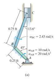
The crankshaft AB turns with a clockwise angular acceleration of  $20 \text{ rad/s}^2$ , Fig. 16–31a. Determine the acceleration of the piston at the instant AB is in the position shown. At this instant  $\omega_{AB} = 10 \text{ rad/s}$  and  $\omega_{BC} = 2.43 \text{ rad/s}$ . (See Example 16.12.)
