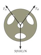
The 5-kg plate is suspended by two straps *A* and *B*. To find the force in each strap we should consider the free-body diagram of the plate. As noted, the three forces acting on it are concurrent at the center. (© Russell C. Hibbeler)
