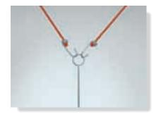
Three forces act on the ring. Since these forces all meet at a point, then for any force analysis, we can assume the ring to be represented as a particle. (© Russell C. Hibbeler)
