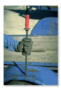
The impulse tool is used to remove the dent in the trailer fender. To do so its end is first screwed into a hole drilled in the fender, then the weight is gripped and jerked upwards, striking the stop ring. The impulse developed is transferred along the shaft of the tool and pulls suddenly on the dent. (© R.C. Hibbeler)
