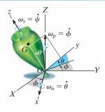
$$\Sigma M_x = -I\dot{\phi}^2 \sin\theta \cos\theta + I_z\dot{\phi} \sin\theta (\dot{\phi}\cos\theta + \dot{\psi})$$
