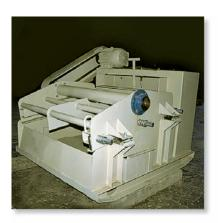
Shaker tables provide forced vibration and are used to separate out granular materials. (© R.C. Hibbeler)
