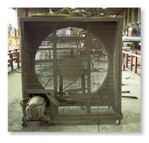
The air on one side of this fan is essentially at rest, and as it passes through the blades its momentum is increased. To change the momentum of the air flow in this manner, the blades must exert a horizontal thrust on the air stream. As the blades turn faster, the equal but opposite thrust of the air on the blades could overcome the rolling resistance of the wheels on the ground and begin to move the frame of the fan. (© R.C. Hibbeler)
