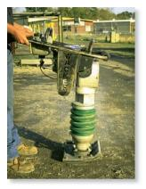
The soil compactor operates by forced vibration developed by an internal motor. It is important that the forcing frequency not be close to the natural frequency of vibration of the compactor, which can be determined when the motor is turned off; otherwise resonance will occur and the machine will become uncontrollable. (© R.C. Hibbeler)
