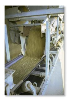
The conveyor belt must supply frictional forces to the gravel that falls upon it in order to change the momentum of the gravel stream, so that it begins to travel along the belt. (© R.C. Hibbeler)
