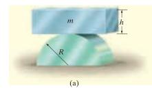
The uniform block having a mass m rests on the top surface of the half cylinder, Fig. 11–19a. Show that this is a condition of unstable equilibrium if h > 2R.
