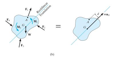
It is also possible to sum moments about other points on or off the body, in which case the moment of  $m\mathbf{a}_G$  must be taken into account. For example, if point A is chosen, which lies at a perpendicular distance d from the line of action of  $m\mathbf{a}_G$ , the following moment equation applies:
