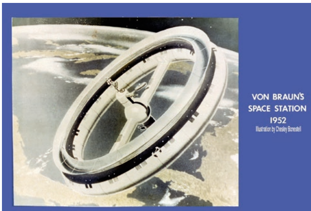
Fig. 2.3 Wernher von Braun's original concept for a rotating space station (NASA image)
