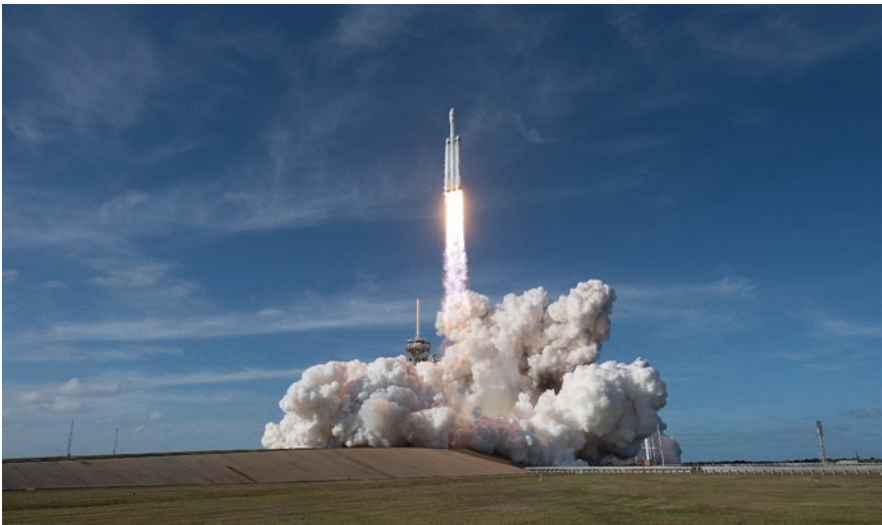
Fig. 1.7 The upward force on a rocket as it lifts off is a direct consequence of Newton’s third law of motion, because what the rocket is really doing is applying the same force downwards to its exhaust plume (Wikimedia Commons, CC-BY-4.0)
