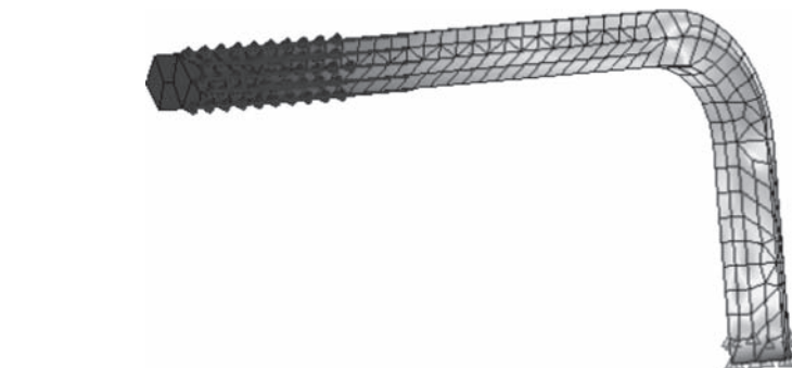
Figure P11-19 “Allen” wrench showing dimensions, loads, and typical finite element model (By Justin Hronek)
