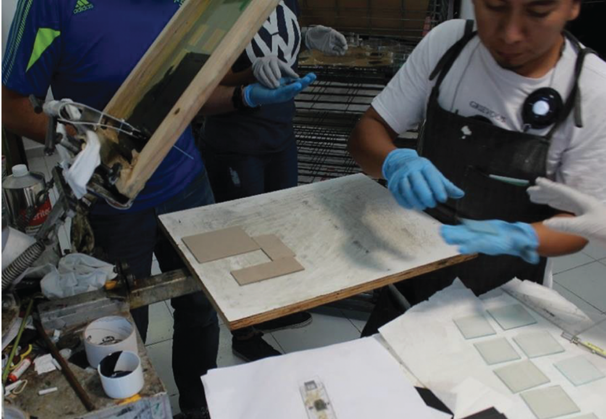
Figure 9.1 Manufacture of low-capital cost mCPSC mini-modules in “Serigrafía e impresos,” a family-run company based in Mérida, (Yucatan, Mexico). Project within a Newton institutional link funding for the collaboration between SPECIFIC-Swansea University and CINVESTAV-Mérida.
