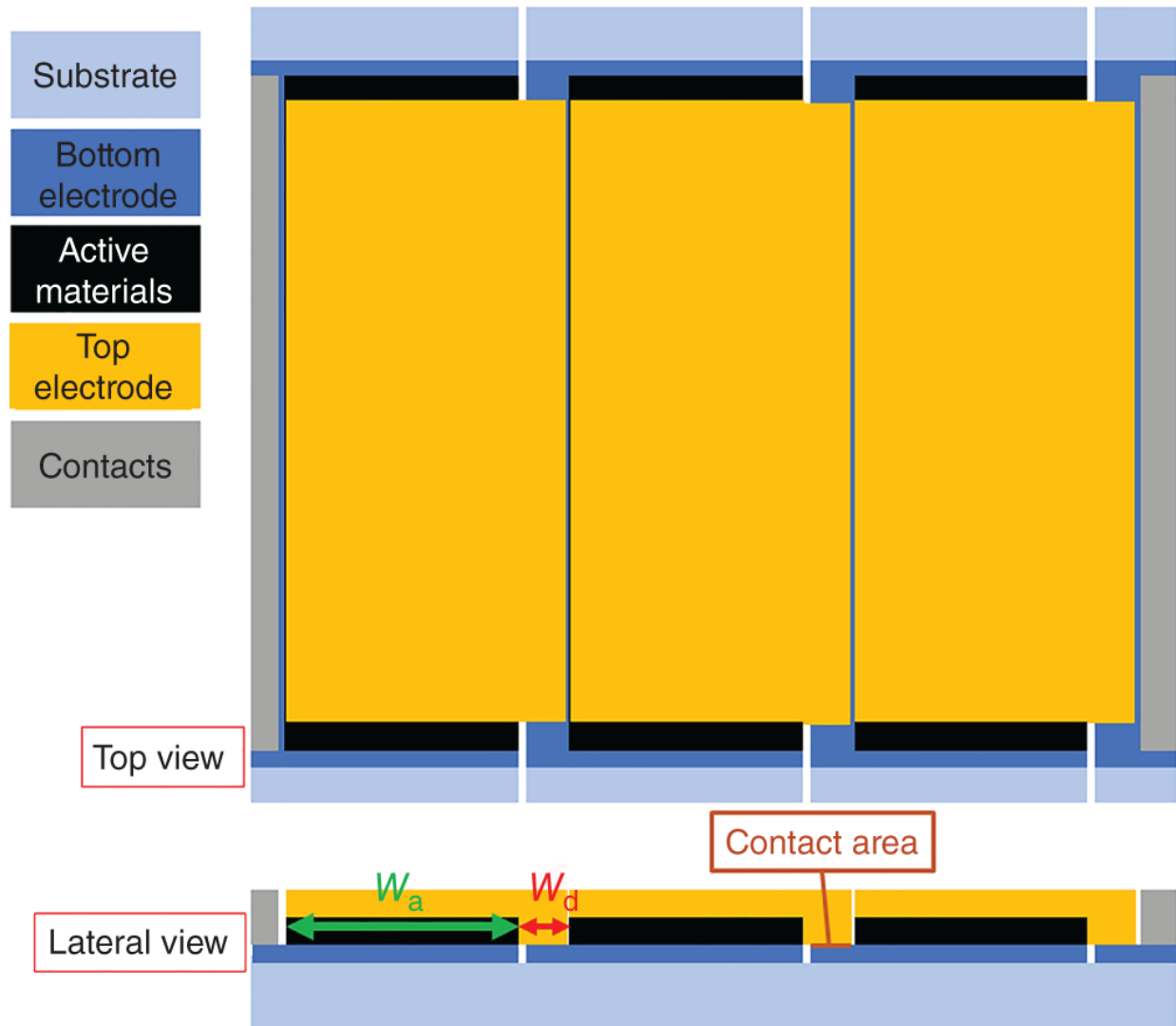
Figure 9.12 Schematic representation of a series-connected module with three single cells. Above, the top view; below, a lateral view.
