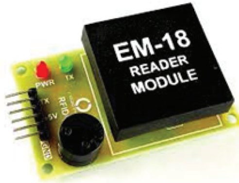
Figure 8.2 The topview EM18 reader modules.
