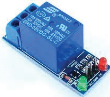
Figure 8.7 The proposed relay.
