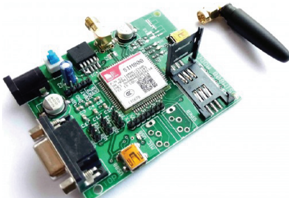
Figure 10.6 Schematic view of GSM module.
