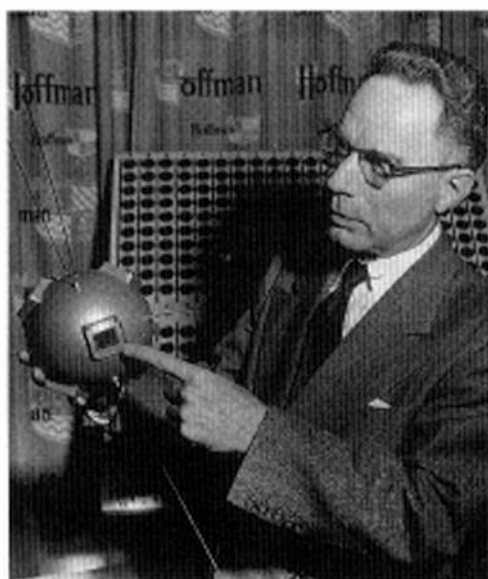
A Hoffman Electronics scientist holds the Vanguard that initiated solar power's use in space. The scientist is pointing to one of the four solar cell clusters that the company manufactured.
