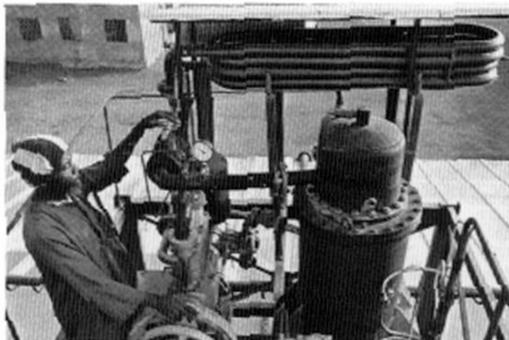
The complicated moving parts shown in this photograph proved to be a fatal flaw to solar-heat powered engines in Africa.
