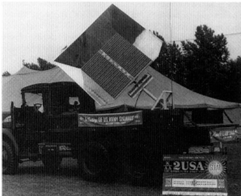
The photovoltaic panels atop this Army truck served as the power source for the first solar-powered transcontinental radio broadcast.
