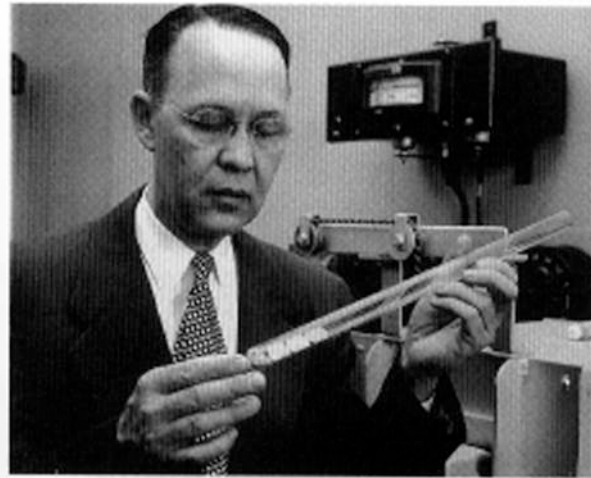
Calvin Fuller placed arsenic-laced silicon into a quartz-tube furnace where he introduced a controlled amount of boron to the material. This resulted in the first solar cell that could generate significant amounts of electricity.
