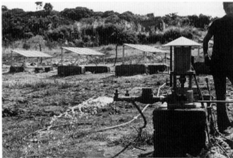
To realize Campana's vision, Dr. Jean Alain Roger designed the world's first photovoltaic-powered pump, shown here operating in Corsica.
