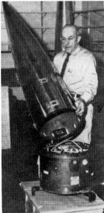
A Navy technician attaches a nose cone embedded with solar cells to a rocket that will be launched to test whether the cells can survive the rigors of space.
