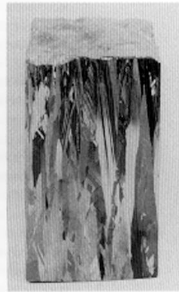
A large polycrystalline silicon ingot. Ingots such as this are sawn into thousands of very thin wafers, which are made into solar cells.
