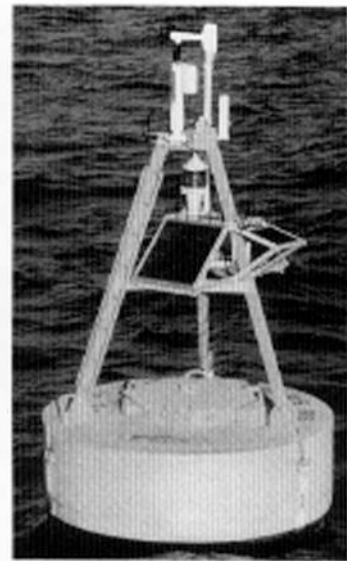
Solarex modules power this buoy's warning light and horn.
