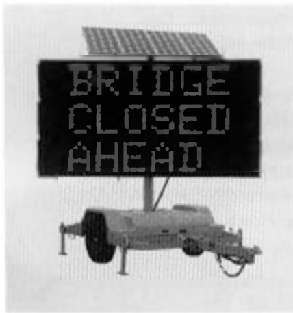
An increasingly common sight: mobile highway signs powered by photovoltaics.
