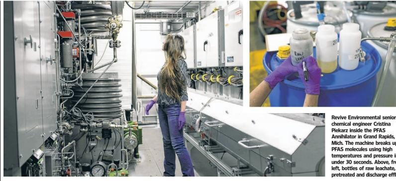
Piekarz inside the PFAS Annihilator in Grand Rapids, Mich. The machine breaks up PFAS molecules using high temperatures and pressure in under 30 seconds. Above, from left, bottles of raw leachate, pretreated and discharge effluent.
