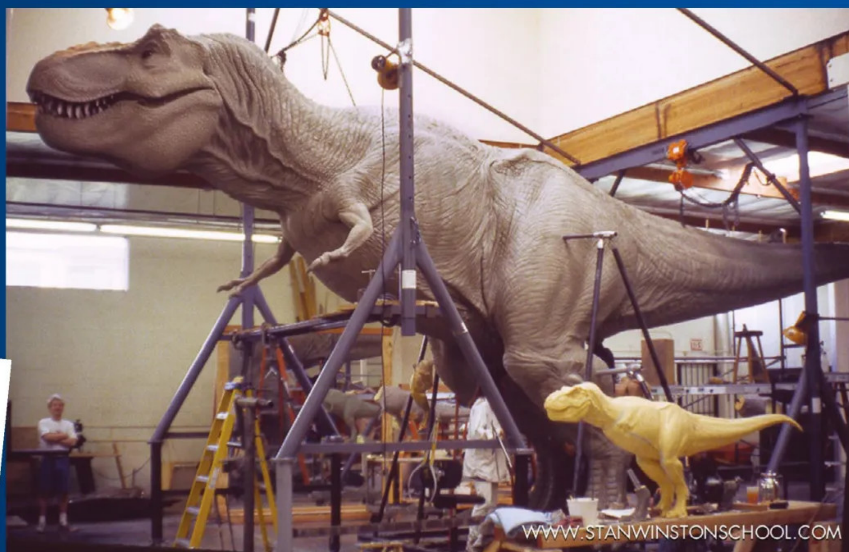
1 A metal skeleton A fifth scale model of the T-Rex is sliced into pieces then each slice is scaled up and cut from wood. These wooden slices are then slotted onto a metal frame.
