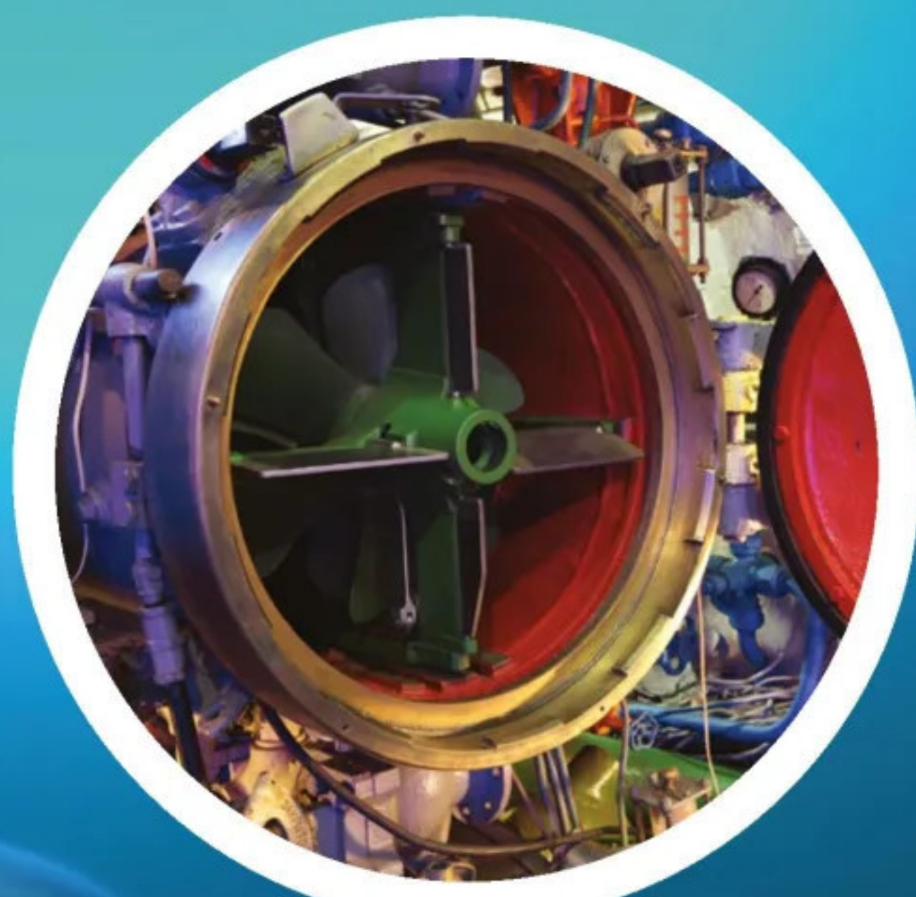
Torpedoes are fired from ships and submarines through torpedo tubes
