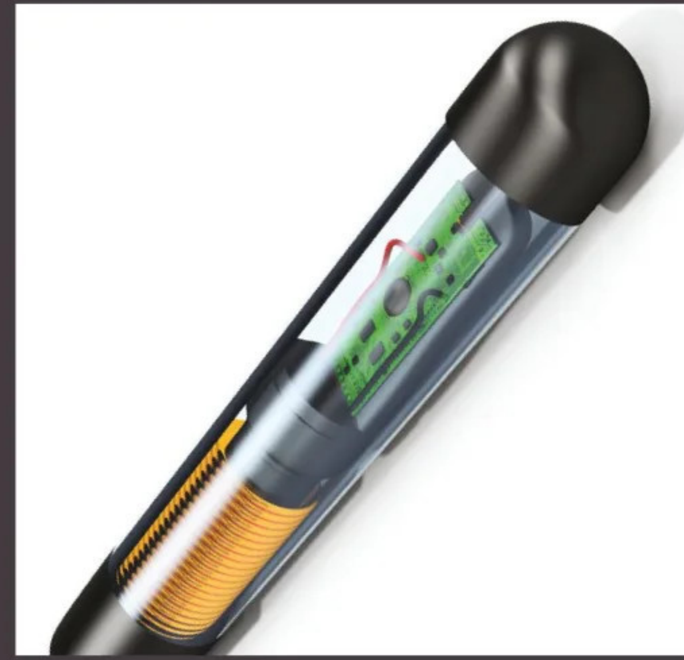
This RFID chip shows the coiled copper antenna it uses to communicate
