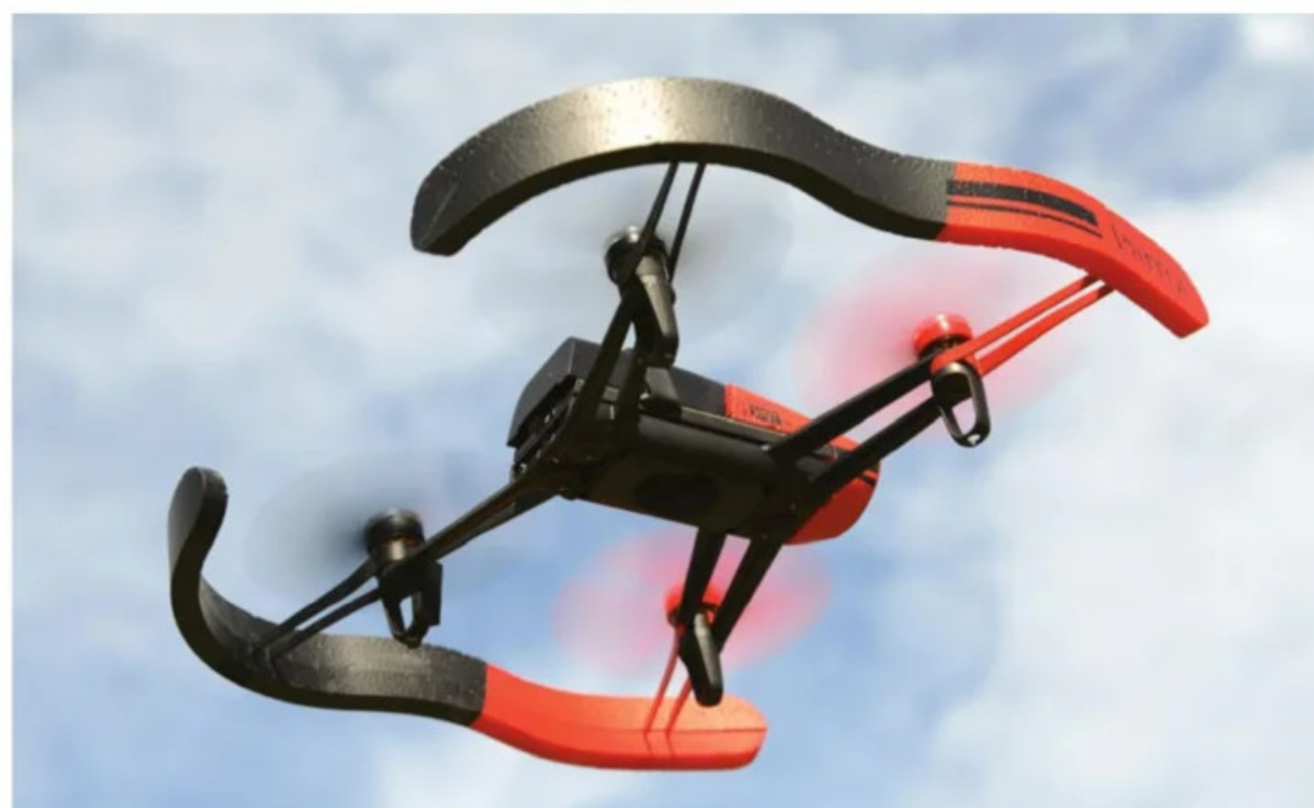
Multicopters typically have an even number of propellers; quadcopters have four
