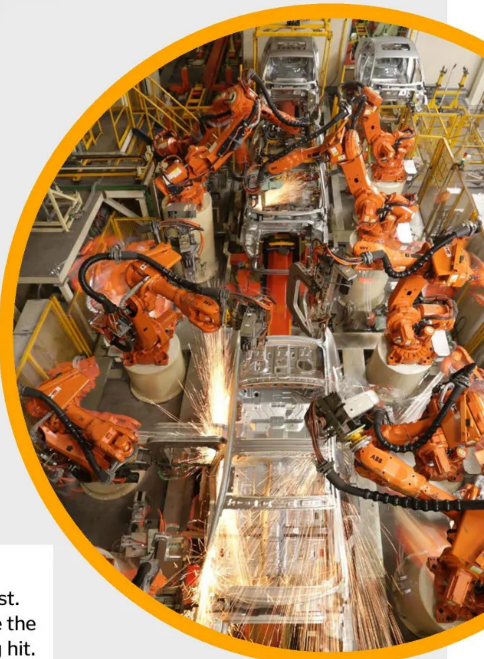
Joints welded by robots are stronger because they are more precise and consistent
