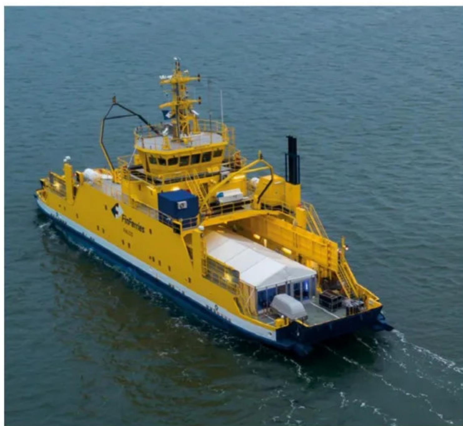
The first automated car ferry, Falco, on its journey across part of the Archipelago Sea
