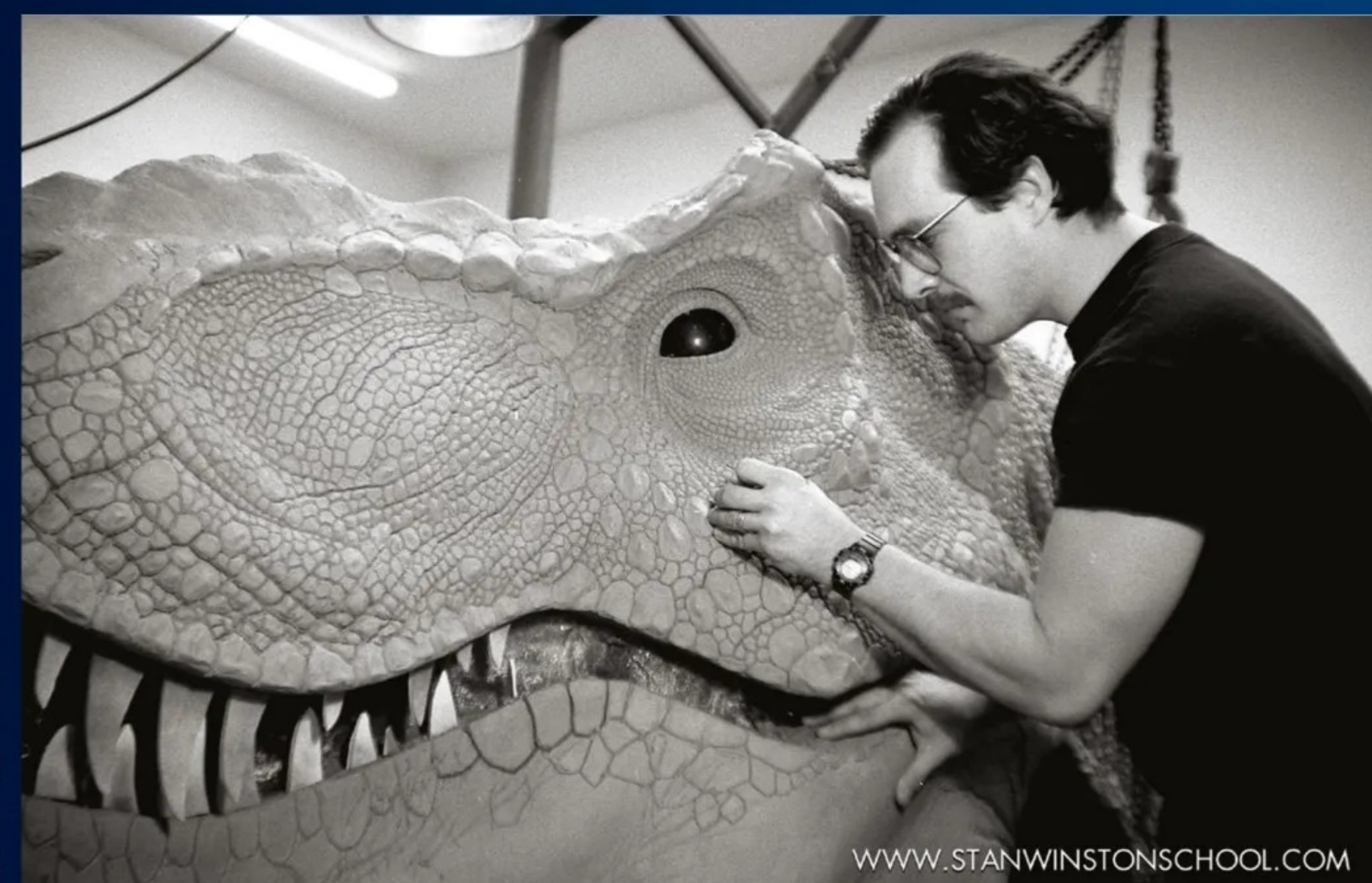
2 Sculpting the body The main frame is covered in chicken wire and fibreglass, then a layer of clay. The clay is sculpted to look like T-Rex scales, and serves as a mould for the skin.
