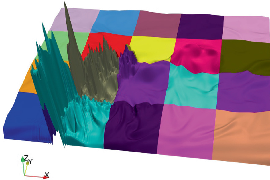
Fig. 1 One 2-d slice of an S3D dataset partitioned into 20 blocks and modeled in parallel, blocks colored by process ID
