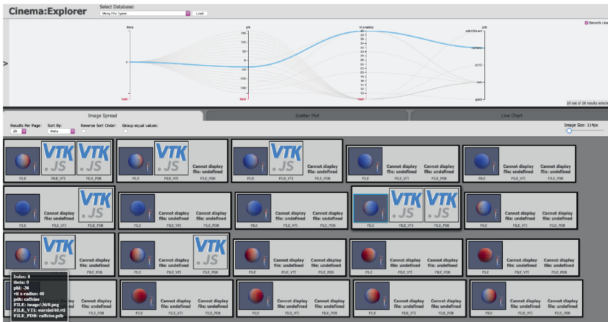
Fig. 9 A simple sphere Cinema database demonstrates the multiple data types in Cinema:Explorer. For each [r^2 - \delta] set of parameters, there is an image. Additionally, some of the [r^2 - \delta] parameter sets have other data types such as a vtk file or pbd file. Clicking on the thumbnail for each extract (vtk or pbd file) will bring up the data in a viewer for that specific data type, see Fig. 10
