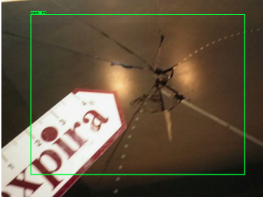
Figure 1.17: Detected crack in the image of hot plate
