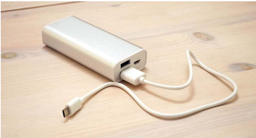
Figure 2-1: A power bank is a good power source for your Arduino experiments.
