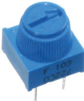
Figure 3-8: A trimpot-style variable resistor (image by oomlout under https://creativecommons.org/licenses/by-sa/2.0/deed.en license)
