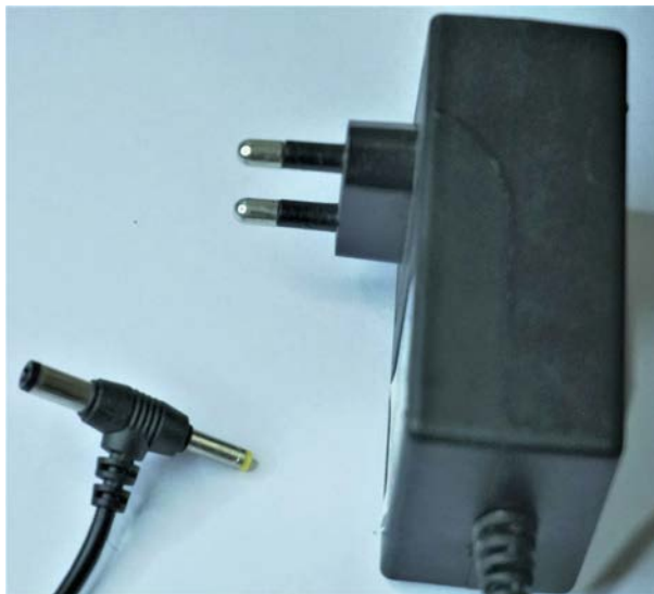
Figure 2-7: AC to DC power adapter with 2.1 mm barrel jack connector.
