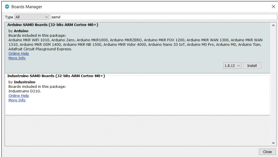
Figure 7-4: Installing, the support for SAMD board.
