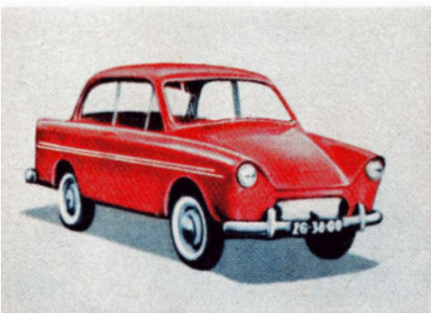
31 DAF Dutch five-passenger sedan with automatic clutch and transmission, V-belt drive, $1,650
