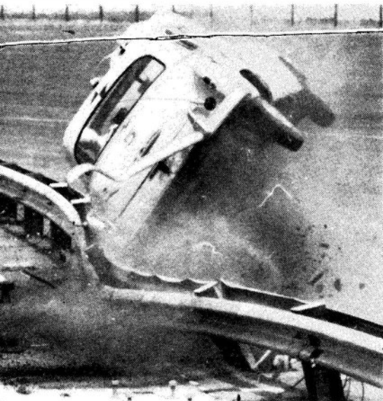
RAILS THAT FAILED include (above) rigid barrier that allowed car to climb fence and crash in other lane, and (left) a "W-section" rail that flipped car high into air, landing it upside down in middle of its own right-of-way.
