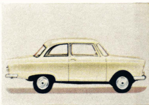
28 DKW 750 with two-cycle three-cylinder engine, front-wheel drive, automatic clutch, about $1,700
