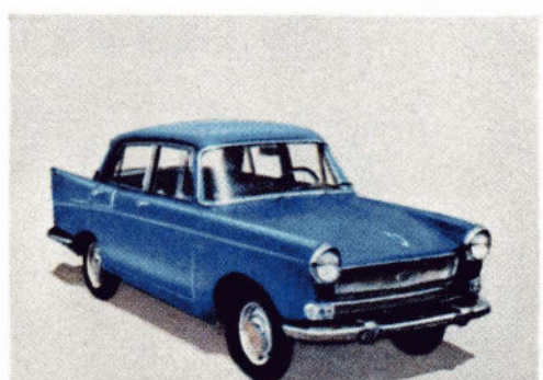
16 Austin A-55, styled by Farina, 53-hp, unitized construction with fully stressed skin, $2,198
