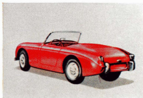
27 Austin-Healy Sprite sports car, 48-hp, 948-cc displacement, rack and pinion steering, $1,795
