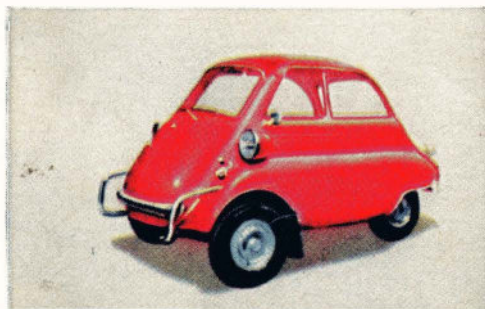
41 BMW Isetta 300 with "in-and-out" front door, seats two, parks nose to the curb, $1,048
