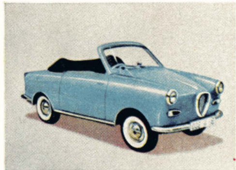
36 Goggomobil T-400 sports coupe, with air-cooled engine, five moving parts, 22-hp, $1,495
