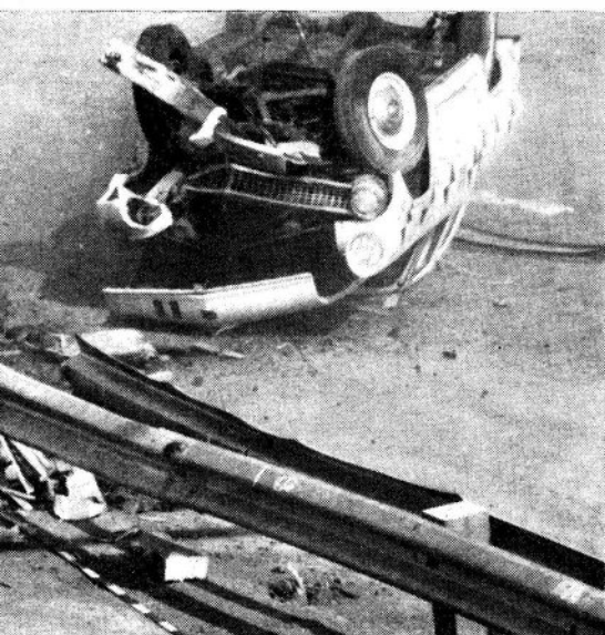
OTHER FAILURES included concrete posts (above) that permitted car to slash through, with little loss in velocity, into other lane, and (left) modified W-section rail that brutally halted car in own lane but demolished automobile.
