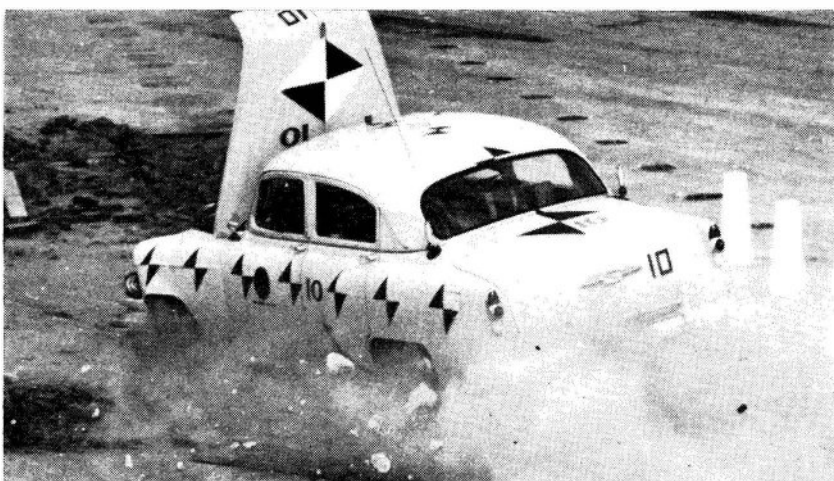
OTHER FAILURES included concrete posts (above) that permitted car to slash through, with little loss in velocity, into other lane, and (left) modified W-section rail that brutally halted car in own lane but demolished automobile.
