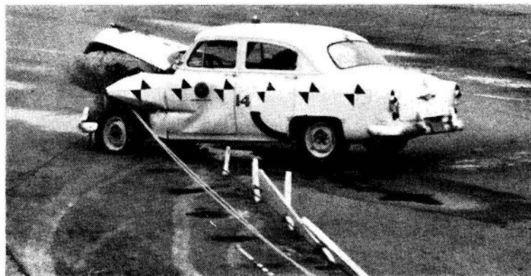
Brought to halt after 64-foot slide, car remains in lane. Tests showed dummy driver suffered "minor bruises."
