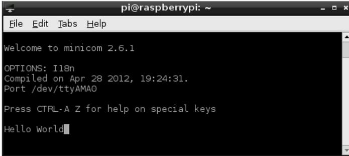
Figure 10.3. Minicom serial communications program.
