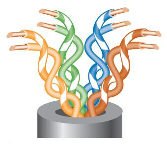
**Figure 2-4** Example of four-pair twisted pair cable
