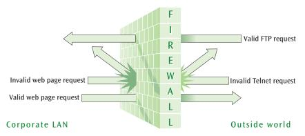
**Figure 8-7** A firewall as it stops certain internal and external transactions
