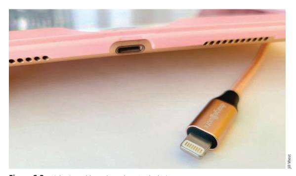
Figure 2-3 Lightning cables only work on Apple devices
