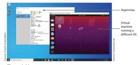
Figure 1-11 A Linux VM running in a hypervisor on a Windows computer
