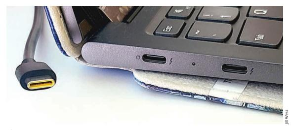
Figure 2-2 Thunderbolt cables use USB-C connectors
