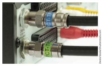
Figure 2-10 Coaxial cables connected to a satellite receiver
