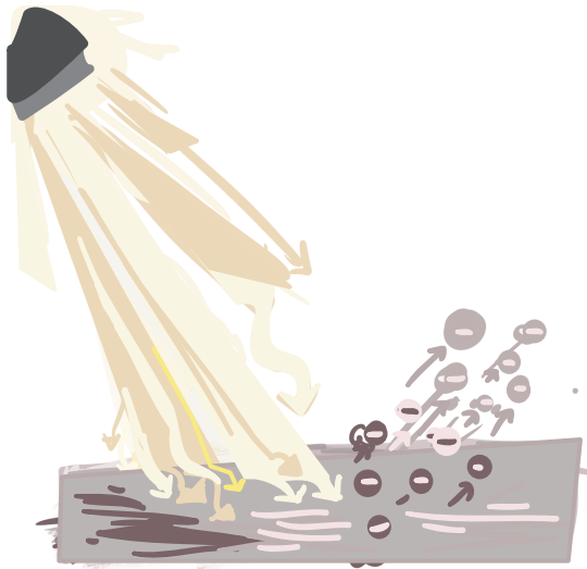
Figure 3. Cartoon view of photoelectric effect. Photons transfer their energy to the electrons in the metal which ejects them from the surface of the material.
